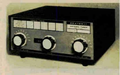
mal RF loss at high frequencies. Its large ceramic feed-through insulators are designed to withstand high voltage RF. This Antenna Tuner is capable of handling power input of up to 2000 watts PEP on side-band and 1000 watts on CW. S0-239 connectors allow incorporation into your 50  $\Omega$  system.
