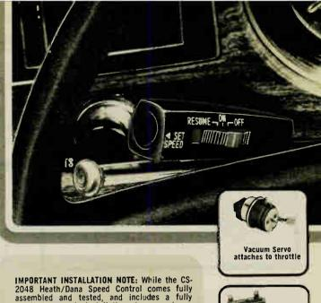
assembled and tested, and includes a fully detailed manual, installation does require a certain amount of mechanical proficiency. Modifications must be made to the throttle linkage of your car, and work must be performed under the vehicle in order to install the speed transducer unit. If you are uncertain of your abilities, you may wish to employ the services of a qualified auto mechanic to install your Speed Control.
