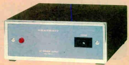
VFA-7401-1 SPECIFICATIONS: Output Voltage: 13.8 VDC regulated (Adjustable from approximately 12 to 15 VDC). Output Current: 4.0 amperes for 20 minutes (40% duty cycle). 3.0 amperes continuous. Output Regulation: Better than 1.5% from no load to full load (3.0 amperes). Output Ripple: Less than 2 mV peak-to-peak. Power Requirement: 110 to 130 VAC or 220 to 260 VAC, 50/60 Hz, at 85 watts (full load). Overall Dimensions: 31/6" H x 71/4" W x 97/6" D (7.8 x 18.4 x 25.1 cm).
