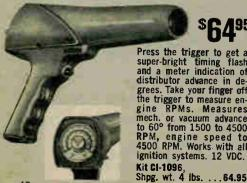
Press the trigger to get a super-bright timing flash and a meter indication of distributor advance in degrees. Take your finger off the trigger to measure en-gine RPMs. Measures mech. or vacuum advance to 60° from 1500 to 4500 RPM, engine speed to 4500 RPM. Works with all ignition systems. 12 VDC.
