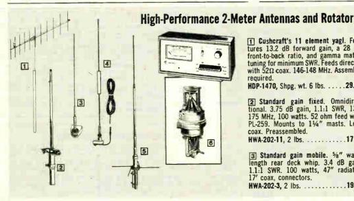
[1] Cushcraft's 11 element yagi. Features 13.2 dB forward gain, a 28 dB front-to-back ratio, and gamma match tuning for minimum SWR. Feeds directly with 52Ω coax, 146-148 MHz, Assembly
