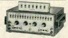
The IG-5257 makes receiver alignment fast and easy. It features 15 selectable markers, video and audio carrier markers for channels 4 and 10, and a diode modulator for Video Sweep Modulation. Other features include a 400 Hz tone for FM receiver alignment, and a multi-step attenuator pad to assure proper impedance matching and to avoid stage overloading.
