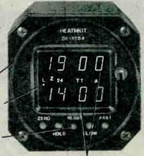
4-digit red LED displays with automatic dimming.
