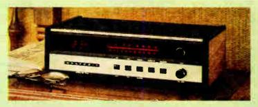
The front panel features finger-flip switches for on/off; AM/FM selection; radio or electronic alarm; "wake-up" alarm set; "Snooze" cycle; plus volume and AM/ FM tuning controls. Black plastic cabinet with brushed aluminum trim strip, and simulated walnut-grain end panels. For 120/240 VAC, 50/60 Hz operation. 41/2" H x 135/8" W x 81/8" D.
