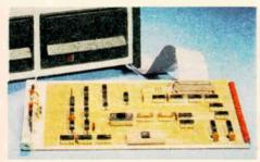
The WH17 INCLUDES the Interface/Oisk Controller Circuit Board — An Extra Cost Option with Most Other Units.
