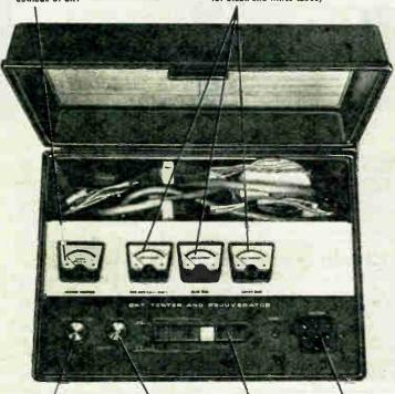
Heater Adjust Coutrel. Sets voltage at CRT cathode for precise testing. Cutoff/Power Control. Turns unit on or off, sets control grid voltage Pushbutton Operation. Positive action pushbuttons control all tests and processes. Restore Indicator.
