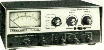
IP-2718 SPECIFICATIONS: Regulation: Load: less than 0.1% variation from no load to full load on 20-volt supplies; less than 2% variation from no load to full load on 5-volt supply. Line: less than 0.2% variation for line voltage change of 10 volts on 20 volt supplies; less than 0.15% variation for line voltage change of 10 volts on 5-volt supply. Power Requirement: 100-135 or 200-270 VAC, 60/50 Hz, 100 watts full load. Dimensions: 4½" H x 104" W x 9" D.
