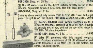
1 Hustler's 4-BTV vertical uses a single 50Ω feedline, covers 10-40 meters, and is rated at full legal power on SSB & CW.
