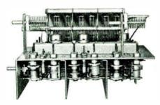
Coil and bandswitch assembly comes to you prewired and aligned. Note the ceramic coil forms and bandswitch wafers used for hi Q.
