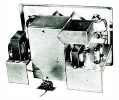
Note the extensive shielding used in the LG-1 to assure output only on pure fundamental frequencies, A line filter is also incorporated to prevent radiation through the line cord.
