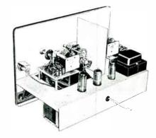
Sweep oscillator and marker sub-assemblies are well isolated through use of shielding and laminated phenolic sub-chassis, minimizing leakage, hum, and internal interference for uniform circuit performance.
