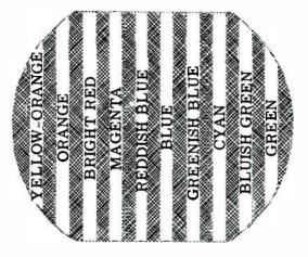
**COLOR BARS** Above are shown the color bars produced by the CD-1 when the hue control of the color set is in the center of its range. A white leading edge and black trailing edge are provided on the color bars to check color fit.
