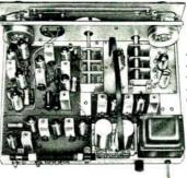
Unique design features a completely prewired and prealigned 3-tube front end for ease of construction. Note the heavy duty individual tuning flywheels.
