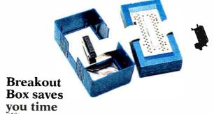
Breakout Box. It provides access to all 25 lines of RS-232C cables linking computer system devices. Twelve LEDs monitor key signal lines while 23 lines can be switch disabled and then cross-connected. Five jumper wires are included. Built-in dual DTE and DCE gender connectors eliminate the need for adapter cables and connectors. Two "AA" batteries power the line monitoring LEDs but they are not needed for the Breakout Box to operate. 13/8" H x 21/8" W x 6" D.
