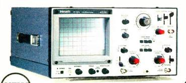
Dual trace 25 MHz oscilloscope
