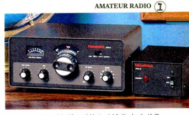
RECEIVER: Sensitivity: 0.2 μV for readable signal; 0.5 μV or less for 10 dB S + N/N. Selectivity: Wide, 1 kHz max. @ 6 dB; Narrow, 250 Hz @ 6 dB. Dynamic Range: 85 dB. Image & IF Rejection: 60 dB, min. Audio Hum Noise: –60 dB. Audio Output: 1 watt into 8Ω.
