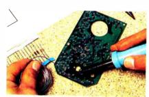
PROPER SOLDERING: Most Heathkit manuals teach reliable soldering for maximum kit life.
