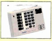
NEW optional RF Remote Control Accessory enables direct and computer control of HERO 1 from up to 100 feet away
