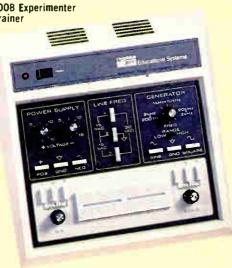
Solderless breadboard sockets for circuit building
