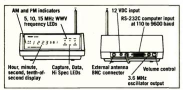
An RF receiver scans the 5, 10 and 15 MHz frequencies of WWV and locks onto the strongest signal. A selectable audio monitor permits you to listen to the audio broadcast on these frequencies. To improve reception of WWV frequencies, an external antenna is recommended but may not be required in your area.
