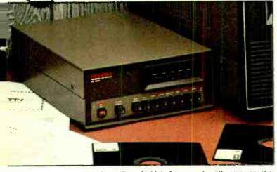
• A "universal" terminal interface – works with any personal or • home computer, such as Heath H-8 or H-89, Commodore, Atari, Radic Shack, Texas Instruments, Apple, IBM, etc. • Built-in supply for noncomputer 20/60 mA TTY operation
