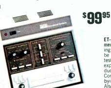
Solderless breadboard sockets for circuits
