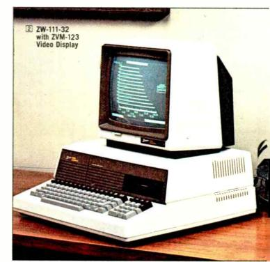
With this control, you can create highly detailed drawings, graphs, etc. Thirtythree special graphic characters are already available from the H/Z-100's keyboard to be arranged and grouped for less detailed graphics. Add eight colors to your monochrome graphics with two Z-219-1 Color Video RAM Chip sets (p. 33).
