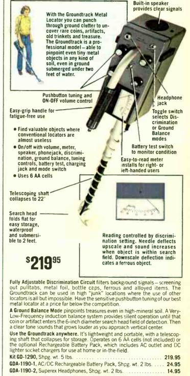
GD-1290 SPECIFICATIONS: Sensitivity: Locates dime at 4" to 6" typical, may be less depending on soil conditions, mode of operation and amount of discrimination selected. Method of Detection: Induction-balance circuit. Detector Output: Meter, speaker, phone jack. Power Requirement: Six AA cells or Rechargeable Battery Pack. Dimensions: Extended height, 451/2." Net Weight: 3.4 lbs.
