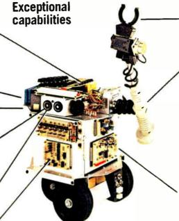
Highly maneuverable: HERO 1's three-wheel drive system, with one wheel both driving and steering, allows the robot to move any where and to turn in a 12-inch radius.
