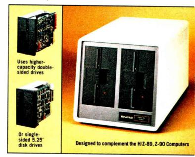
**Designed for 120/240 VAC, 50/60 Hz power,** the H-77/Z-87 and H-37 Floppy Disk Systems are housed in a structural foam cabinet matching the decor of the H/Z-89 and Z-90, measuring 8% H x 8% W x 15" D (21.92 x 22.56 x 38.1 cm).
