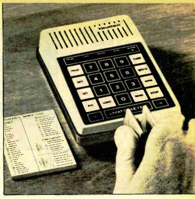
nostics check the microprocessor each time the  $\mu$ Matic Memory Keyer is turned on, and tests buffer memory whenever it is reset.
