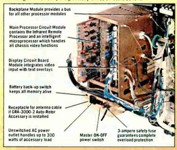
Trouble-saving hookups: The GR-3000 is cable-ready for immediate installation in equipped areas. Direct audio and video input and output jacks on the rear panel permit you to connect and switch between a video recorder/disc player or standard channel reception. A separate input labeled Channel 1 Audio lets you pre-empt program sound (during a commercial, for example) with that from an external source like FM radio, which can be enabled by selecting channel 1 on the remote as usual.
