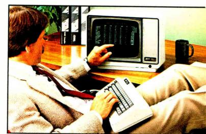
The assembled and tested ZT-1 Information Terminal meets FCC Class B radiofrequency interference (RFI) requirements for use in homes or businesses.
