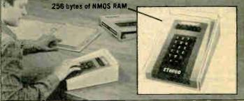
Trainer is mini digital computer: The ET-6800 Trainer has an 8 bit parallel, NMOS, bus-oriented central processing unit. You can access memory locations, enter programs, single-step through programs, alter memory.
