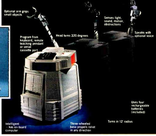
to pick up small objects. The arm extends, retracts and turns — performing mechanical tasks with precision. The robot can also be programmed to speak complete sentences with the optional ET-18-2 Speech Synthesizer.
