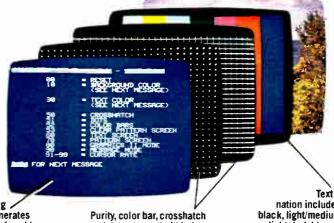
Purity, color bar, crosshatch and dot patterns built in for testing and adjustment after the kit is assembled available for Backdrop and Text in any combination include: transparent, black, light/medium/dark green, light/dark blue, light/medium/ dark red, light/dark yellow, cyan, magenta, gray and white
