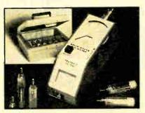
This solid-state Dip Meter can determine the approximate resonant or operating frequency of energized or de-energized circuits and help you adjust traps, detect parasitics or function as a signal generator. A MOSFET paraphase amplifier and hot-carrier diodes provide more sensitivity and a better dip. It uses a Q-multiplier for greater detector sensitivity and a responsive 150 μA meter movement for positive marking. Operates on one
