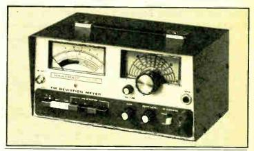
IM-4180 SPECIFICATIONS: Carrier Freq. Ranges: Fundamental, 25 to 50 MHz. Deviation Ranges: 0-2, 0-7.5. 0-20 & 0-75 kHz. Accuracy: ± 3%, full scale, input imped.: 5011 Max. input: 5 V. Scope Output: 13 mV kHz peak
