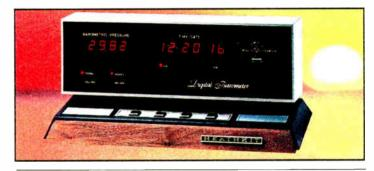
10-1990 SPECIFICATIONS: Barometer Display: 4-digit readout. Separate indicators show whether the pressure is rising or failing, and whether the display is in inches of mercury, millibars or kiloPascals. Pressure Ranges: 28.00 to 32.00 inches Hg (mercury), 981 to 1050 millibars or 98.1 to 105 kiloPascals. Accuracy: 29.00 to 31.00 Hg  $\pm$  0.03 in. Hg at 15-35° C. Power: 120 240 VAC.
