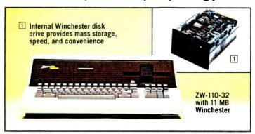
① Winchester disk drive: Conveniently store data that would require several dozen floppy diskettes. And access it ten to twenty times faster. With a massive 11 megabyte storage capacity, the Winchester drive in an H/Z-100 Computer provides more on-line storage for those large accounting, inventory, data base, or technical jobs that once required an expensive mainframe or minicomputer system.
