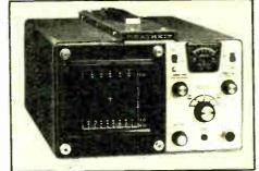
Following the tune-up specifications for any auto and using the Analyzer Operation Handbook, you can detect shorted spark plugs, bad points, defective wiring, worn distributor parts, incorrect dwell angle, cam wobble, plus coil or condenser defects and transistorized or capacitive discharge problems.
