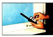
The Heathkit Heat Sniffer locates energy-robbing leaks quickly
