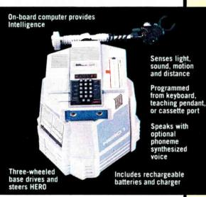
Programmable robot: Completely self-contained, HERO 1 is capable of interacting with its environment. It detects light, sound, motion and objects in its path. It can travel over a set course and repeat specific functions on a predetermined schedule. With an optional arm and voice, HERO 1 can grasp items and speak.
