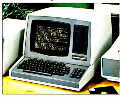
Calculator-format 12-key numeric pad: Makes entering arithmetic programs faster. Shifted functions give you control to make insertions or deletions.
