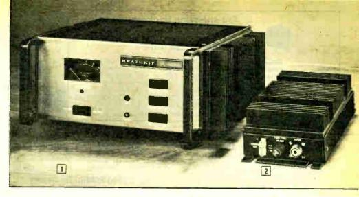
VI-2290 SPECIFICATIONS: Band coverage: 144 to 148 MHz.Power Input: 1 to 10 watts SSB. FM or CW. Impodance: 50\(\text{L}\) input YSWR: (@ 10 watts drive) 2.0:1 or less. Power Dutput: 75 watts @ 10 watts drive. Duty Cycle: 50\(\text{%}\). 10 minutes on. 10 minutes off. Inserfion Loss: (Antenna to Receiver) less than 0.6 dB. IM Distortion: -24 dB. Power Requirement: 120 VAC at 4 amperes; 240 VAC at 2 amperes: 12 VDC at 11 amperes. Dimensions: 6.25" Hx 13.5" Wx 12.25" D.
