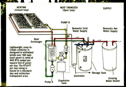
**Designed for maximum water heating efficiency:** In the NS-1100's custom-designed heat exchanger, both fluids (water and the heating fluid) are moved through the exchanger by separate pumps. The active flow of both fluids increases the system's water heating efficiency.
