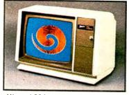
extensively. Use in home or office – has UL, and CSA approvals. For 120 VAC, 60 Hz power. The ZVM-134 Color Display Measures 13.5" H  $\times$  20" W  $\times$  15" D (34.29  $\times$  50.8  $\times$  38.1 cm).
