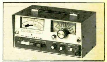
IM-4180 SPECIFICATIONS: Carrier Freq. Ranges: Fundamental, 25 to 50 MHz. Deviation Ranges: 0-2. 0-7.5, 0-20 & 0-75 kHz. Accuracy: \$3%, full scale. Input Imped.: 50\( \) Max. Input: 5 V. Scope Dutput: 13 mV kHz peak
