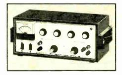
A time-saving, low-cost addition to any audio test bench: The IG-5218 provides both sine and square wave signals for gain & frequency response measurements, Harmonic Distortion checks and other amplifier tests. The square wave output with a risetime of 50 nanoseconds is ideal for audio response testing or as a trigger for digital circuit testing.
