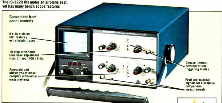
The first portable Heathkit oscilloscope features dual-trace capability, wide bandwidth, algebraic add, up to 5X sweep magnification, invert display function and a bright CRT
