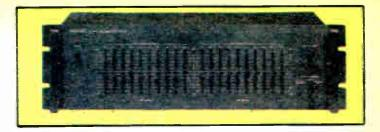
AO-1703 SPECIFICATIONS: Center Frequencies: 32, 64, 125, 250, 500, 1 k, 4 k, 8 k, and 16 kHz. Max. Boost: +11 dB. Max. Cut: -11 dB. S/N: 90 dB A weighted below 1.5 V. Total Harmonic Distortion: Less than .001% from 20-20,000 Hz @ rated output. Freq. Response: 20-20,000 Hz. Overload: 8 V rms. TIM: Less than .03%. Rated Output: 1.5 V rms. Filter Q: 1.2 ±5%. Clipping Indicator: Approx. 7 volts rms. Power Req.: 120/240 VAC. 50/60 Hz. Dimensions: 5.75" H x 19" W x 14" D.
