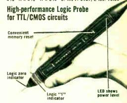
Detects and indicates high and low logic levels in TTL or CMOS circuitry. Detects logic signals to 100 mHz, polarity and presence of single pulses as short as 10 nSec, and shows intermediate or "bad" logic levels. Includes 34" power leads with strain relief and color-coded mini-clips, and detachable high-frequency ground clip. 34" H x 1" W x 944" L.
