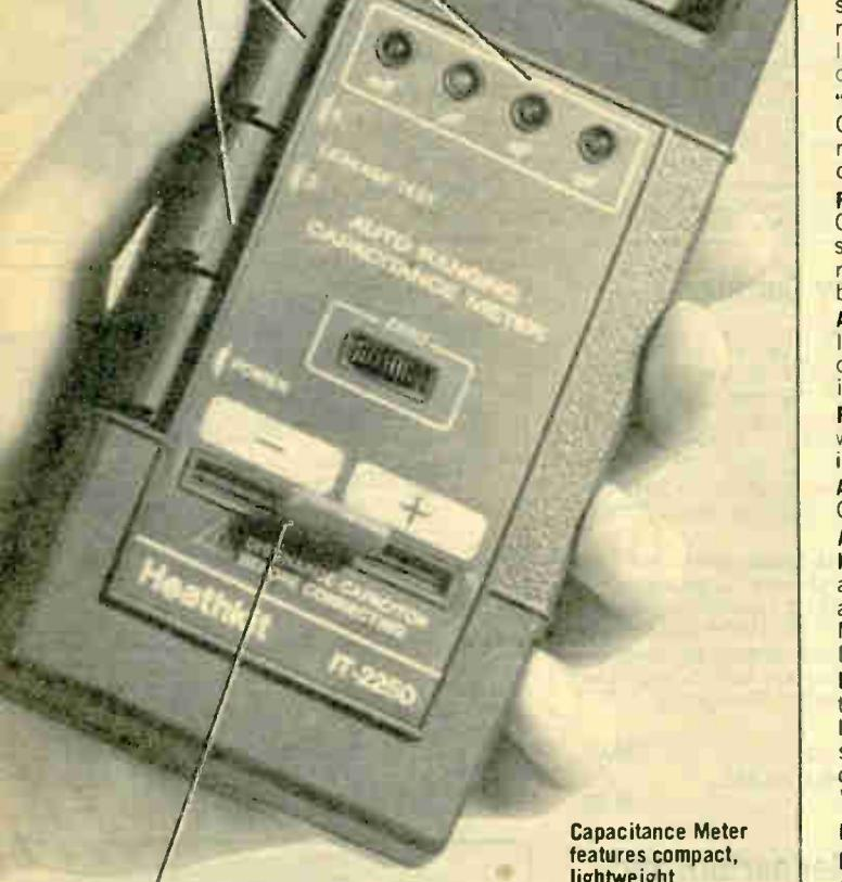
Polarized "Kelvin" terminals, combined with special test cable (included), allow more accurate capacitance measurements
