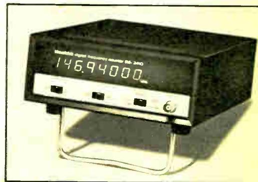
**IM-2410 SPECS:** Max. Sensitivity: 25 mV, RMS. Input impedance: 1 MΩ shunted by less than 24 pF. Input Protection: 150 VAC, up to 100 kHz—derating to 5 VAC from 160 MHz to 225 MHz. Time Base Frequency: 3.58 MHz. Temperature Stability: -10 ppm from 0° to 40°C. Power Req: 120/240 VAC, 50/60 Hz. Dimensions: 3.38" H x 7.25" W x 9.5" D (8.59 x 18.42 x 24.13 cm).
