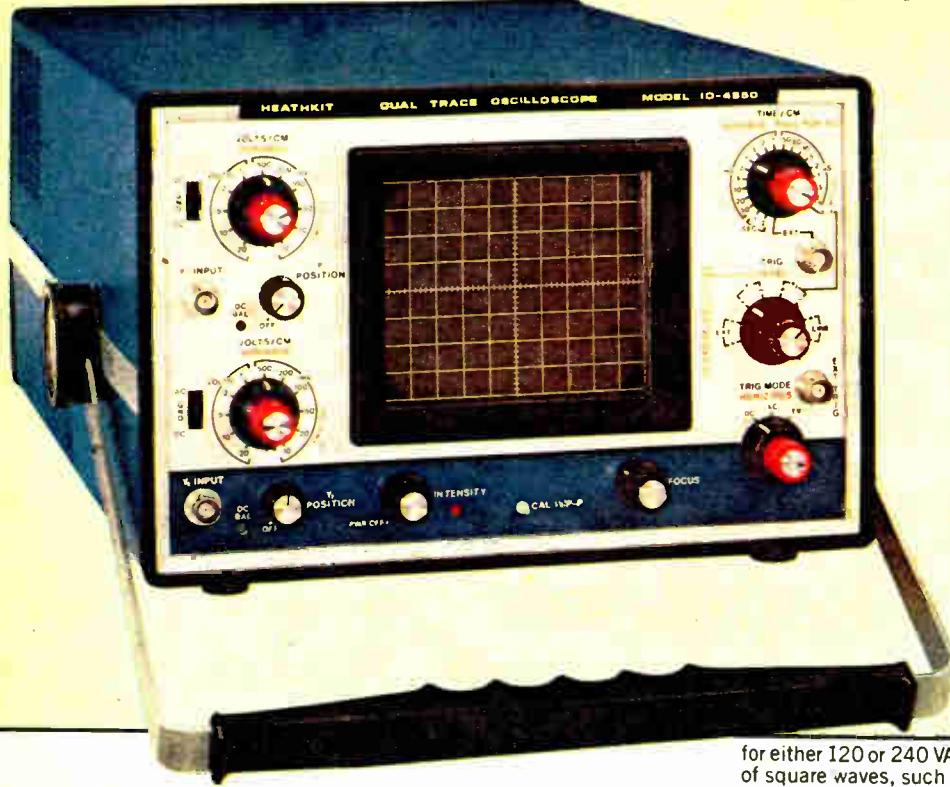
If you're looking for a dual-trace, DC-10 MHz oscilloscope to round out your test bench, look no further. The IO-4550's extra-bright trace allows easy reading, even in high ambient light. The two vertical input channels have a maximum sensitivity of 10 mV/cm to give you accurate measurements.
