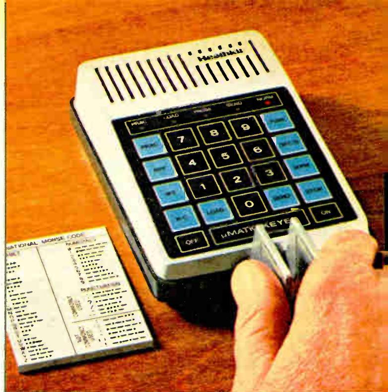
**CMOS memory with battery backup** retains the buffer contents, as well as the last-selected speed, spacing, weight, and repeat count whenever the Keyer is turned off or unplugged. Built-in diagnostics check the microprocessor each time the Keyer is turned on, and also test buffer memory whenever your μMatic Memory Keyer is reset.
