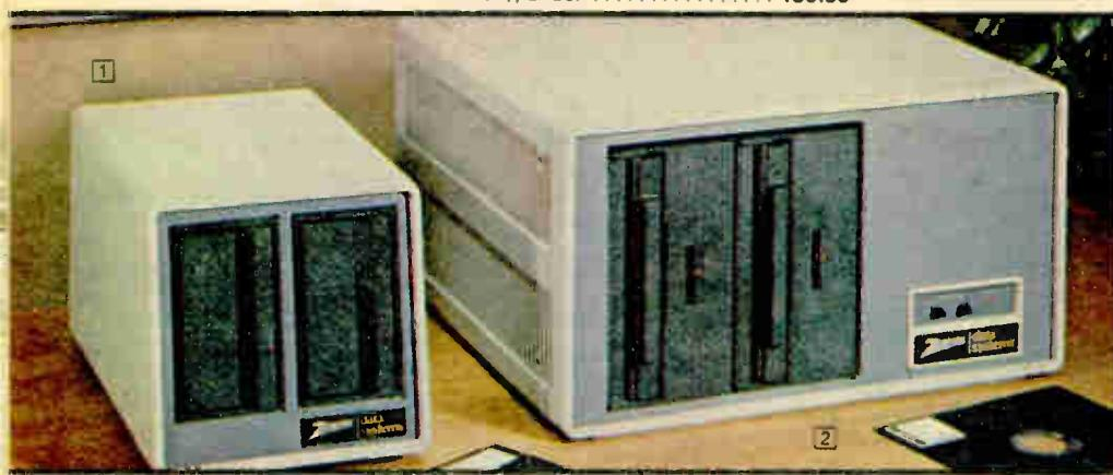
**① Add up to 1.28 megabytes of data storage with Z-37 Disk System**
