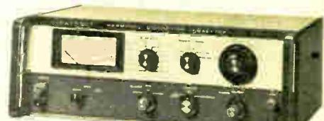
**Outstanding sensitivity and bandwidth:** The IM-5258 measures total harmonic distortion (THD) down to 0.03% from 5 Hz to 100 kHz, with +5% accuracy. Six ranges cover 0.03 to 100% harmonic distortion. The IM-5258 can also function as an 1 mV to 300 V AC voltmeter with +5% accuracy. Max. input impedance is 1 megohm shunted by 70 pF. Not for use in strong RF fields. 120/240 VAC, 50/60 Hz, 5.38" H x 15" W x 11.5" D.
