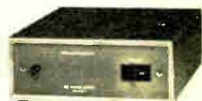
Designed to provide the 13.8 VDC required by the VF-7401, the VFA-7401-1 AC Power Supply may also be used with most other equipment requiring +13.8 VDC at a maximum of 3A continuous, 4A intermittent. Easy-to-build kit can be wired for either 120 or 240 VAC, 50/60 Hz. Output regulation within 1.5%. 3 1/4" H x 7 1/4" W x 9 1/4" D.
