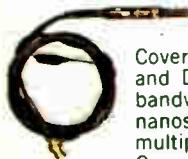
Covers DC to 15 megahertz (X1) and DC to 80 megahertz (X10) bandwidths. X10 rise time, 4.0 nanoseconds. Has two-position multiplier for X1 and X10 probe tip. Compensation range of 15 to 50 picofarads. Includes 4.5-foot cable and probe with three-position slide switch.
