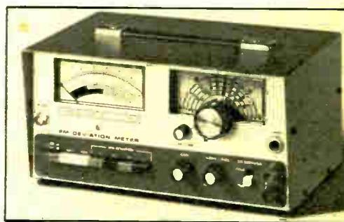
**IM-4180 SPECS:** Carrier Freq. Ranges: Fundamental, 25 to 50 MHz; Deviation Ranges: 0-2, 0-7.5, 0-20, & 0-75 kHz. Accuracy: ±3% full scale. Input Imped.: 50 Ω. Max. Input: 5 V. Scope Output: 13 mV/kHz peak.
