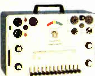
Test vacuum tubes on basis of total emission – for shorts, leakage, open elements and filament continuity.
