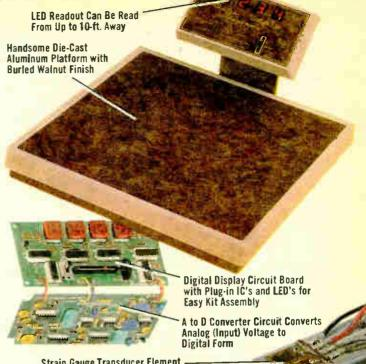
Strain Gauge Transducer Element Similar to Those Used in Expensive **Laboratory Scales**
