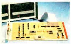
The H17 INCLUDES the Interface/Disk Controller Circuit Board — An Extra Cost Option with Most Other Units.
