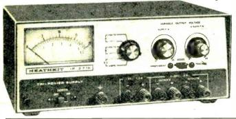
!P-2718 SPECIFICATIONS: Regulation: Load: less than 0.1% variation from no load to full load on 20-volt supplies; less than 2% variation from no load to full load on 5-volt supply. Line: less than 0.2% variation for line voltage change of 10 volts on 20 volt supplies; less than 0.15% variation for line voltage change of 10 volts on 5-volt supply. Power Requirement: 100-135 or 200-270 VAC, 60/50 Hz, 100 watts full load. 0imensions:  $4\frac{1}{2}$ " H x  $10\frac{3}{4}$ " W x 9" D.
