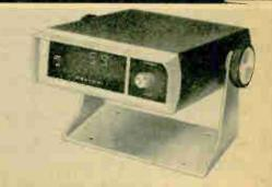
MI-101 SPECIFICATIONS: Accuracy: ±2%, ±1 digit. Current drain: 300-500 mA. Power requirement: 10-17 VDC @ 500 mA. Dimensions: 21/4" H x 65/8" W x 81/2" D (less gimbal hardware).
