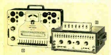
17-3117 SPECIFICATIONS: Sockets: 4-pin, 5-pin, 6-pin combination and pilot light. 7-pin miniature, octal, loctal, 10-pin miniature, 9-pin novar, 9-pin miniature, 12-pin compactron, 5-pin nuvistor, 7-pin nuvistor, 7-pin muvistor, 8-by sions: 8-by2" H x 13" W x 5-by2" D.
