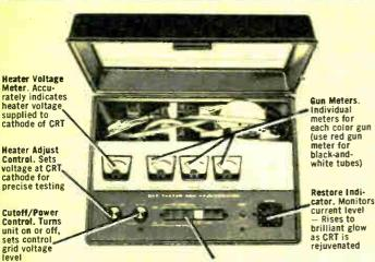
Pushbutton Operation for all tests and processes.
