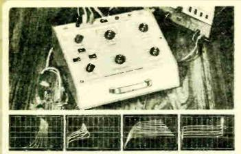
Negative resistance and interbase resistance (Rbb) for unijunction transistors.
