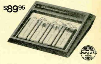
Makes basic circuit designing a breeze. Solderless sockets and a built-in power supply makes hook-up and teardown quick and easy. It can even be used to test electronic components.
