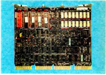
Fully Assembled and tested KD11F board
