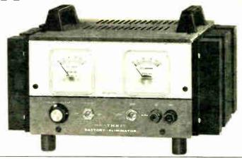
IP-2715 SPECIFICATIONS: Output Voltage; variable from 9-15 VDC. Output Current: 12 amps continuous, 20 amps intermittent (per derating curve in manual). Ripple: less than 1% at full load. Regulation: less than 2% variation from no load to full load. Fuses: 7A, 3 AG slow-blow primary; 20A, 3 AG output. Power Requirements: 110-130 VAC, 7A or 220-260 VAC, 3.5 A, 60/50 Hz. Dimensions: 5¼" H x 11# W x 11# D.
