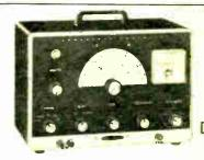
1 Stereo Generator -- Provides audio or composite stereo signal for multiplex adapter adjustments...RF carrier modulated by these signals for tuner & receiver adjustments...phase test function for subcarrier transformer adjustment...a variable level crystal-controlled 19 kHz pilot signal for checking receiver lock-in ranges...plus built-in sweep and marker signals for RF & IF alignment. With test leads.
