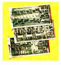
H8-1 Memory Board. 8Kx8 memory card supplied with 4K memory, plugs directly into H8 bus. Features maximum storage capacity of 8192 8-bit words. Uses modern 4Kx1 static memory IC chips for easy assembly and service. Access time, less than 450 nS. With on-board regulators, heat sinks and full buffering. Expandable to 8K memory with H8-3 chip set helow
