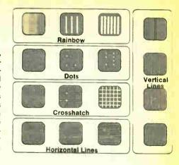
1G/SG-5240 SPECIFICATIONS: Chroma Carrier: 3563.795 kHz ±0.005% crystal-controlled. Master Timer: 377.616 kHz ±0.005% crystal-controlled. RF Carrier: Channel 4, 67.250 MHz ±0.01% crystal-controlled. RF Output Level: 5000 μV min. into 300 ohms. Video Modulation: 50% (approx.) On-Time Interval: 5 minutes min. OFF pushbutton can override time out. Power Requirement: Two 9-volt transistor batteries; with 180 mAH capacity (NEDA #1604). Dimensions: 5.4″ L x 2.75″ W x 1.15″ D.
