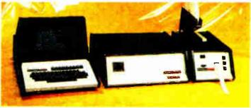
H11 System One: The minimum recommended H11 System. Includes H11 Computer, H11-1 4K Memory (for a total of 8K memory), H11-2 Parallel Interface, H11-5 Serial Interface, H9 Video Terminal and H10 Paper Tape Reader/Punch. If purchased separately, \$2765.00. Heath System Price is \$2626.75.
