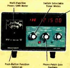
Adds real operating versatility to any station! The SB-634 features a 24-hour digital clock; ten-minute ID timer (with aural or visual alarm), RF wattmeter with 200 or 2000 watt full-scale ranges; an SWR bridge with sensitivity control; and phone-patch that can be used either manually or with VOX control. The wattmeter's impedance is a nominal 50 ohms and insertion loss is negligible. The phonepatch provides at least 30 dB of isolation between
