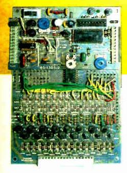
The "heart" of the GR-2000 is the channel selector circuit board. It provides the direct electronic tuning, the dot generator for color alignment, and positions and controls the numerical channel display.
