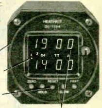
4-digit red LED displays with automatic dimming.
