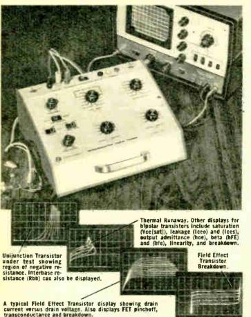
The fast, easy way to check semiconductor parameters is with your oscilloscope and the IT-3121 Curve Tracer
