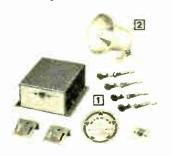
Ideal for cars with CB rigs, tape players, etc. Under-dash alarm set switch has a 5-15 second adjustable delay so you can enter or leave your car without sounding the alarm. An optional horn relay adapts the GD-1157 to cars whose horns do not use a relay or use a plug-in relay. Optional siren accessory provides attention-getting "yelp" sound instead of sounding the car horn. With all switches and hardware. Alarm unit, 21%" H x 434" W x 5" D. For 12 VDC negative ground only.
