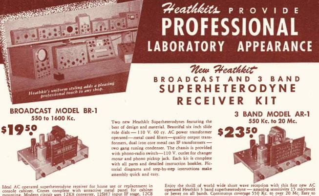
Ideal AC operated superheterodyne receiver for home use or replacement in console cabinet. Comes complete with attractive metal panel for cabinet mounting. Modern circuit uses 12K8 converter, 12SH7 input IF stage, 12C8 output IF stage and first audio 12A6 beam power output stage, 5Y3 rectifier. Excellent sensitivity for distant reception with selectivity which effectively researces adjacent stations. separates adjacent stations.
