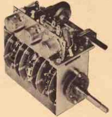
Farnsworth TV Tuner adjusts to any 8 channels. Rotary switch type with fine tuning control. Uses 6BA6RF 6AC5 mixer, 6J6 oscillator tubes (not supplied). Wiring diagram included. Have fun this winter experimenting with television. This well built tuner uses ceramic sockets--best of ceramic condenser and has individual slug tuned coils for each band. Quantity limited. Order now. No. 318. Shipping Wt. 3 lbs.
