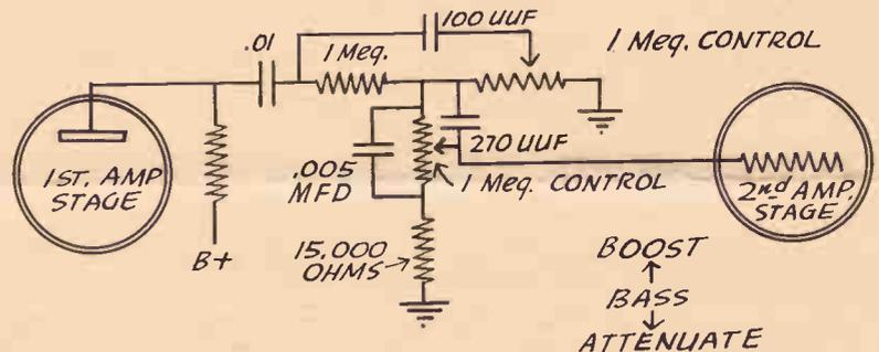
An excellent dual tone control using only standard resistors and capacitors which gives base and treble boost or attenuate. It is simple and easy to build and does not introduce the distortion inherent in choke and feedback type circuits--try it--it's the best we've heard and the cheapest. It does reduce overall volume however.
