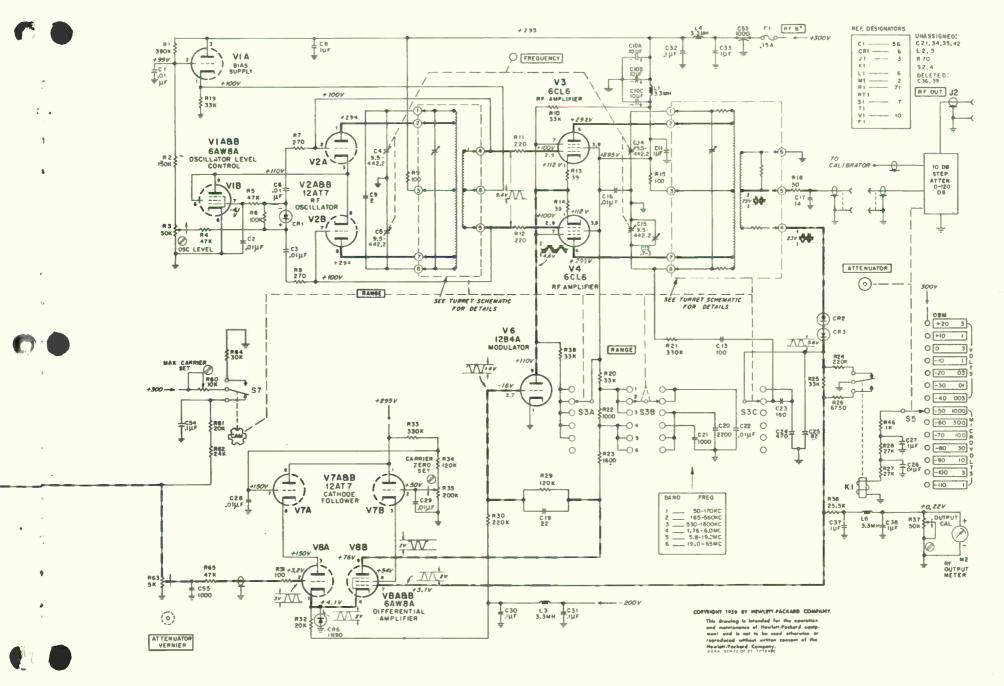
Figure 4-9. Signal Generator (Sheet 2 of 2)
