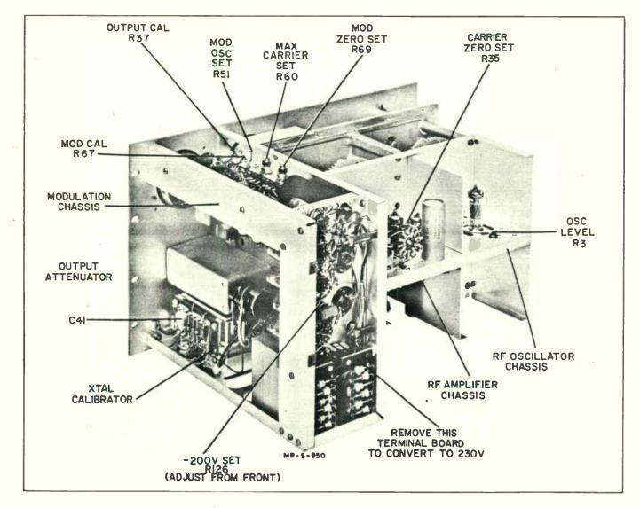
Figure 4-1. Location Diagram Model 606A
