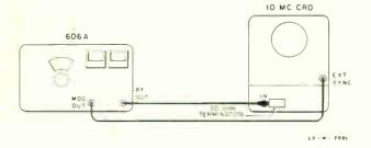
Figure 4-2. Modulation Meter Calibration
