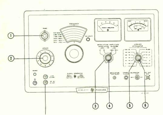
B + FUSE NO R.F. OUTPUT AND OUTPUT METER PINNED TO LEFT IF BLOWN.
