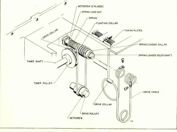
Figure 4-6. Installation of Drive Cable Assembly
