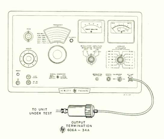
The attenuator on the Model 606A Signal Generator is calibrated only when used with a load of 50 ohms. For high impedance loads or receiver inputs the output termination (@ 606A-34A) is recommended. This output termination is designed for use at the end of a 50 ohm shielded cable, and to operate into a high impedance (500 ohms or greater) load.
