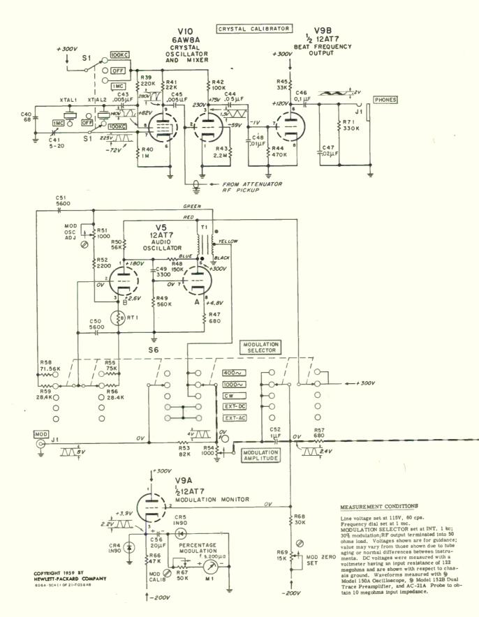
Figure 4-9. Signal Generator (Sheet 1 of 2)
