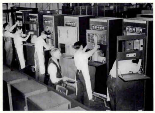
FIG. 6. ASSEMBLY LINE OF 1 KW. FM TRANSMITTERS AT GENERAL ELECTRIC'S SCHENECTADY PLANT. AMPLIFIER UNITS CAN BE ADDED TO INCREASE THE OUTPUT TO THE ANTENNA, IF NECESSARY
