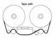
Insert the end of the leader tape into one of the hub sits of the take-up reel and slowly turn that reel by hand until the sit is covered by tape (at least one full turn). You can now move the tape forward by pressing PLAY (3) or F FWD (7).
