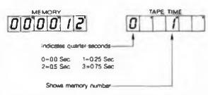
Thus memory point 1 has a time value of 12 00 seconds. Ouarter second values other than 0 are possible only during display of the current counter value (see next item). For example, if a number 3 was displayed on the TAPE TIME counter instead of the 0 in the above example, a time value of 12 75 (12 and three quarter) seconds would be indicated.
