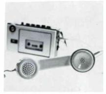
To play it back over the phone — just plug it into the output of the cassette machine and push the button — it couples right into the earphone . . . works better than the phone receiver!
