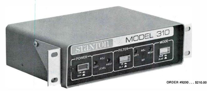
The Stanton 310 Preamp features universal mounting by special brackets, instant selection of flat or NAB postemphasis curves, switchable effective rumble filter, individual adjustment of gains and high frequency responses, trimming of the capacitive cartridge loading at the input, provision for setting the power transformer for either 117 or 230V operation at 50 or 60 Hz and immunity to external magnetic AC fields.
