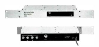
Modulation Sciences' CLD-2504 Composite DA is a problem solver. Its one-in four-out, unity gain configuration makes distribution of the composite baseband signal as easy as distributing audio. The high impedance input avoids circuit loading; the four low impedance outputs drive a wide range of equipment. All connectors are BNC's. The Composite DA provides greater than 50 dB of isolation between outputs.
