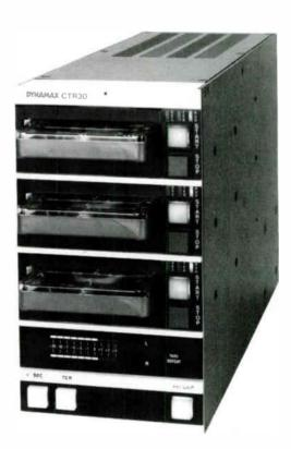
If space is at a premium, then the CTR 30 Triple Stack from Fidelipac is a must consideration. Three decks with the recorder built-in as standard. The bottom deck records as well as plays. Utilizes CTR10 electronics (see page 34). All Plug in boards are interchangeable with those used in CTR10 series machines. All Decks are removable for service without disabling the machine. Audio Switcher and mixer are included to permit connection to single console input.
