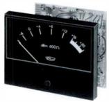
The PPMO2 peak program meter is designed for peak audio level measurement in a wide range of broadcast and professional applications, in place of the conventional average-reading VU meter. Because of its peak reading characteristic, the PPM provides a much more accurate representation of the maximum audio level
