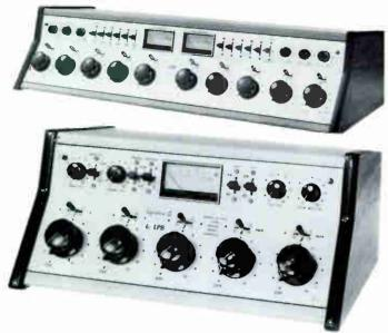
The LPB SIGNATURE II consoles feature transformer audio inputs. Monitor speaker muting and on-air light relays are provided. A cue position is provided in each mixer and all models include an internal cue system consisting of a cue amplifier, level control and 5" speaker. The internal monitor amplifier is switch selectable to monitor program or two external monitor inputs. The illuminated VU meter reads the program output at all times.
