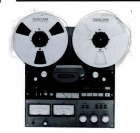
A 2-track  $\frac{1}{4}$ " 2 channel half track mastering and broadcasting recorder/reproducer with  $10\frac{1}{2}$ " reel capacity, sync capability, full servo, SMPTE interlock capability through accessory connector and punch in/out recording. The 42 also features NAB or IEC equalization, dump edit, search to zero and search to cue,  $7\frac{1}{2}$ -15 ips speeds and  $+4\frac{1}{2}$  input/output.
