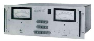
The AAM-1 Analog Antenna Monitor is designed specifically for measuring the parameters of AM broadcast frequency directional antenna systems. The monitor measures the relative current in each tower, the ratio of the current in each tower to that of a reference tower and the phase of the current in each tower relative to that of the reference tower. The AAM-1 can be equipped for up to eight input samples without external switching. Two reference towers can also be selected for DA-2 applications.
