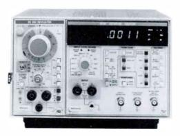
Used together, the AA 501 Distortion Analyzer and SG 505 Oscillator provide the *automatic* solution to your distortion measurement needs. The AA 501 is so automatic, that no level setting, tuning or nulling is necessary. In fact, the engineer at the transmitter end of a proof can literally sit back, put up his feet and read the numbers off the digital readout as it comes across.
