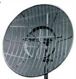
Anixter Communications (Mark Antennas) offers a variety of sizes of Heli-Arc welded aluminum Multi-element Grid Parabolas for point to point relay operation in the 400 to 2700 mHz frequency range. The patented grid of construction is lightweight, yet extremely strong. One of the outstanding advantages of the grid antenna is that it has wind loading characteristics of only 25 to 40% of comparable size solid parabolas.
