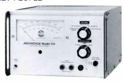
The Advantage 310 Audio Noise and Level Meter from Valley People incorporates the Trans-Amp<sup>TM</sup> active, balanced differential, low-noise preamplifier as the input stage which allows the device to accurately measure extremely low noise levels without errors caused by the use of op-amp "instrument" preamps commonly found in even the most expensive general purpose equipment.
