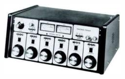
The Model 6618 audio console features six mixing channels, three inputs per mixer, stereo or mono outputs, built-in 10 watt monitor amplifier, selectable muting, on-air light relays, VCA audio attenuators, a choice of preamplifier types, LED line switch indicators, barrier strip input and output terminations, an extra monitor output at line level and plastic conductive main pots.
