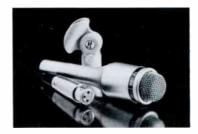
The DO-56 is a chock mounted omnidirectional dynamic microphone for hand-held broadcast applications. All handling noises and cord vibration are isolated from the microphone element. Shock isolation is enhanced by having the main acoustic cavity and the diaphragm/voice-coil assembly is isolated as a unit from the case making capsule/case collision impossible.
