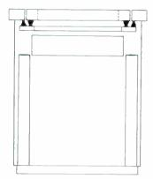
Allied's turntable isolator has been integrated into a package known as the 8100 shock absorber. This approach attacks head-on the many problems associated with protecting otherwise noise free turntable-tone arm combinations from all types of interference. Gives 8 to 10 dB of feedback headroom improvement and up to 20 dB of isolation.
