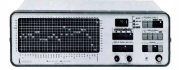
A fully portable unit for real time, ½ octave audio spectrum display and reverberation analysis. Peak and averaged measurements, two memories, RT60 and Decay Plot capabilities, built in Pink Noise Generator. I/O logic interfaces with digital peripherals.
