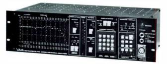
The White Instruments 200 signal analyzer offers 30 triple tuned filters on 1/3 octave I.S.O. centers from 25 Hz through 20 kHz. Octave band and 1/6 octave plug filers are available. 30 by 15 LED display plus separate dB/SPL, overrange, and 2 seven segment readouts. 8 memories. 1, 2 and 3 dB scales. Processes peak and average simultaneously. 3 time constants. All functions are microprocessor controlled. Offers a long list of plug-in options.
