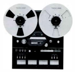
A 4-track  $\frac{1}{4}$ " recorder/reproducer with 15-7 $\frac{1}{2}$  ips speeds, 10 $\frac{1}{2}$ " reel capacity, full frequency response in sync mode, function and output select and punch in/out recording. The 34 also features  $\pm$  12% pitch control, dump edit, cue control, FL tape counter and zero return.
