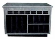
A-LINE turntable bases are constructed of ¾" high-density particle board covered with standard laminates. Tops are 1¼" thick. Turntable bases are normally supplied with rack rails constructed of 11 gauge steel, tapped to accept 10-32 standard EIA rack panels. Cover panels are available at \$6 per bay. Custom cabinets with record and/or tape storage inserts are available.
