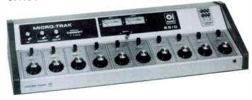
The Model 6510 features ten mixing channels, fourteen inputs, stereo or mono, selectable muting switch, relays for "on-the-air" lights, high quality VU meters, VCA attenuators, plug-in printed circuits cards and switches for easy maintenance, pushbutton input selector switches, barrier terminal strip input and output terminations, monitor output at line level, sealed main pots and compact design.
