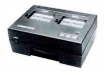
This duplicator system contains solid state digital logic using advanced integrated circuits to command two precision DC servo control motors for foolproof protection against destruction of your master tape. It provides for automatic stop at the end of the duplicating cycle. Automatic level controls, track selector switch, built-in erase and automatic rewind of the master and slaves are also standard features.
