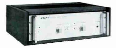
The CROWN Power Line Three is a rack-mounted power amplifier rated at 90 watts per channel into 8 ohms, with a T.H.D. of less than .05%, and I.M.D. of less than .05% and a slew rate of 12 volts per microsecond. The frequency analyzing display shows peak levels in all three frequency bands, provides information on spectral
