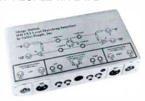
The HH 2 x 2 level matching interface is a line amplifier/attenuator which interfaces +4 or +8 dBm professional recording or broadcasting equipment with -10 dBm high fidelity and semi-pro equipment. Because the unit is transformerless, it achieves improved transient response. Each HH 2 x 2 level matching interface is a complete stereo system. Indeed, it is a stereo amplifier which boosts -10 dBm signals to a nominal +4 or +8 line level output.
