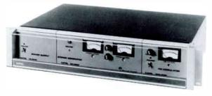
The SM2200 Stereo Generator consists of a sub-carrier oscillator, balanced modulator and channel amplifier, packaged in a modular unit for use with the FMX-2200S.
