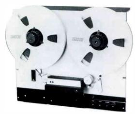
1/4" two channel, half track reproducer with 25 Hz tone sensor, end of message and cuetone relays with adjustable delay (100 milliseconds to 15 seconds). 7½-3¾ ips speeds. 19" rack mount. Designed for automated broadcast systems and other high reliability reproduce only applications. 15-7½ ips speeds available on special order.
