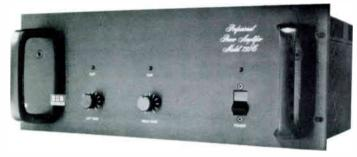
The BGW 750B and 750C are rack-mounted power amplifiers rated at 225 watts minimum sine wave continuous average power output per channel into 8 ohms over a power band of 20 Hz to 20 kHz with guaranteed transient intermodulation distortion of less than .02%, inclusion of clipping indicators on the 750C, addition of LED light ladder VU meter display on the 750B, dual professional input connecters, XLR and ¼" phone jack and a plug-in matching transformer provision.
