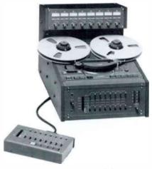
1/2" eight channel recorder/reproducer. DC-servo capstan with ±7% vari-speed. 15-7½ ips speed. +4 or -10 dB input/output level select. Real time tape counter with LED display. Zero return. Test oscillator (1 kHz or 10 kHz). Microprocessor controlled transport logic and dynamic braking. Full function channel status select panel with individual or master control. Automatic monitor switching. Headphone output with channel select. External test input.
