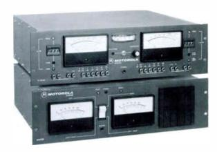
In the MOTOROLA C-QUAM AM STEREO SYSTEM, as in present AM broadcast standards, the angle modulated carrier is amplitude modulated with the sum of the audio information present in the pro-
