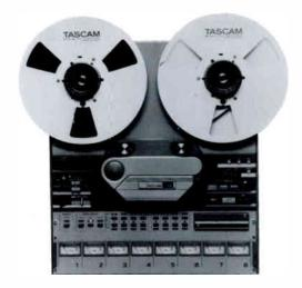
An 8-track ½" 8 channel production recorder/reproducer with -10 RCA input/output, 10½" reel capacity, full frequency response in sync mode, full servo, SMPTE interlock capability through an accessory connector and punch in/out recording. The 58 also features pitch control (15% coarse/0..7% fine), manual tach wheel edit, dump edit, search to zero and search to cue and 15 ips speed.
