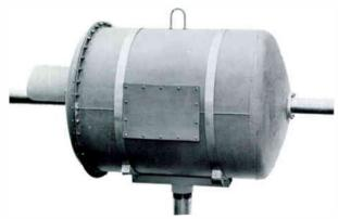
ERI isolation transformers are designed to couple the FM power across the base insulator of a transmitting tower used jointly for AM or FM antennae without introducing objectionable mismatch into the FM feed line.
