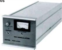
The FMX-2100S FM Modulator is a modular packaged frequency modulation cable transmitter designed specifically for CATV and CCTV applications. When used with the SM-2200 Stereo Generator it makes possible the origination of stereo programming. With direct audio sources it can add varied FM signals to the cable system.
