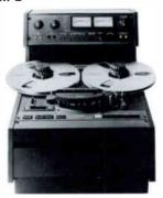
1/4" two channel, half track recorder/reproducer with extra quarter track playback head. Includes a microprocessor transport logic and dynamic braking. Zero return. External machine control interface connector for synchronizers or the optional CB-116 auto-locator.
