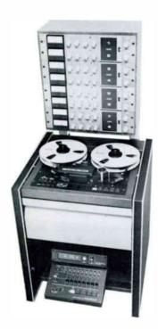
1" eight channel, recorder/reproducer. Includes remote session controller (DB-150) and real time tape counter with LED display. Zero stop. 30/15 ips speeds. 600 ohm balanced output. DC-servo capstan with  $\pm\,12\%$  vari-speed. Console mount. 15-7½ ips speeds available upon special order.
