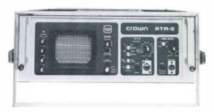
The Crown RTA-2 is designed for audio-range real-time spectrum analysis in 1/3 and full octave bands. All the sub-systems needed to perform quick, accurate on-site equalization of sound-reinforcement systems are included in the RTA-2.
