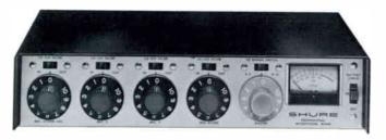
The M-67 is a transistorized microphone mixer/remote amplifier specifically designed for professional applications. The excellent performance and versatility of this complete, compact mixer make it an ideal choice for studio, remote, or original sound reinforcement use, and as an "add-on" mixer for expanding existing facilities. It is also ideally suited for use with tape recorders and VTR's to provide multiple microphone inputs.
