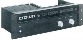
Retaining the D-150A tradition for sonic accuracy and reliability, the CROWN D-150A Series II is rated at 80 watts per channel into 8 ohms, 250 watts into 8 ohms mono. The frequency response is ± 0.1 dB DC to 250 kHz at one watt into 8 ohms-±1 dB DC to 100 kHz., less than .001% harmonic distortion, less than .01 l.M. distortion and 6 volts per microsecond slew rate.
