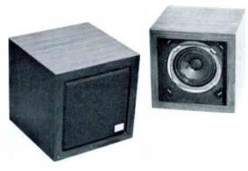
The ANNOUNCER full range loudspeaker is the ultimate in performance in a compact size. The wood cabinet is covered in walnutgrained vinyl and is perfectly square. As with all ALC loudspeakers, the grill snaps away and the system has an overall fuse. The high-compliant full range transducer produces quality sound from below 60 Hz to beyond 15 kHz.
