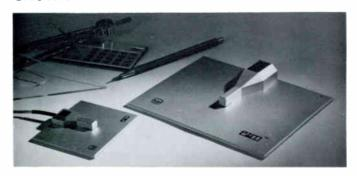
The pressure recording process, invented by Long and Wickersham, introduced a bright new concept to audio engineering. They discovered that sound approaching a boundary such as a floor, wall, table, podium, etc. creates a thin zone in which the direct and reflected signals are coherently in phase and reinforce each other. The Crown PZM microphone creatively realizes the potentials of that invention offering significant improvements in signal clarity and range. Comb filtering is eliminated.
