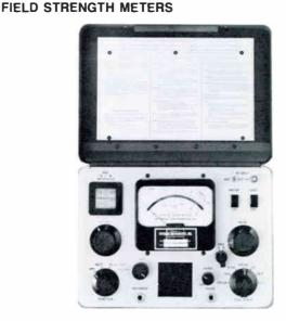
The Potomac line of field strength meters represent a new generation of precision instruments for direct measurement of electromagnetic fields in the 100 kHz to 960 mHz frequency spectrum. These units are intended for portable field use and include a laboratory quality receiver, integral shielded loop antenna, precision attenuator, internal calibration source, and voltage regulated battery
