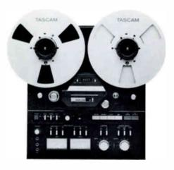
A half-track  $\frac{1}{4}$ " master recorder/reproducer with  $10\frac{1}{2}$ " reel capacity,  $15-7\frac{1}{2}$  ips speeds, independent L & R record mode, simul-sync, full frequency response in sync mode, function and output select and punch in/out recording. The 32 also features  $\pm 12\%$  pitch control, dump edit, mic inputs, independent input/output level controls, headphone jack with volume control, cue control, FL tape counter and zero return.
