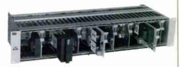
The MAP IMPAC series PC card system can provide simple solutions to your most complex audio processing and control requirements. IMPAC offers the unique choice of either self contained or remote controlled operation featuring solid state switching and voltage controlled amplifiers for silent remote control of all switching and level control functions.
