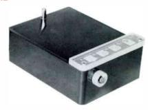
The AUDIOLAB TD-1B tape degausser with automatic overhead thermal protection erases audio tape, carts and cassettes. It erases up to 34" tape widths, accommodates up to 10½" reels, provides a wide focused magnetic field to assure complete erasure and provides results every time with a simple two pass operation for broadcast NAB audio cartridges.
