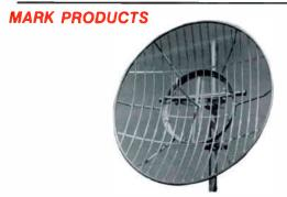
Mark Products offers a variety of sizes of Heli-Arc welded aluminum Multi-element Grid Parabolas for point to point relay operation in the 400 to 2700 mHz frequency range. The patented grid of construction is lightweight, yet extremely strong. One of the outstanding advantages of the grid antenna is that it has wind loading characteristics of only 25 to 40% of comparable size solid parabolas.
