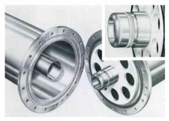
Comark rigid coaxial transmission line provides outstanding features such as constant impedance, high power capacity, and low insertion loss. Sizes to 8 3/16" Heliarc-welded flanges and wrist band bullet construction 3 1/8" and above.
