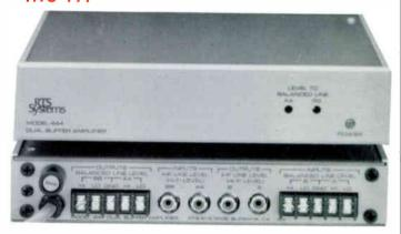
The Model 444 is a dual, two channel buffer amplifier designed to interface professional systems with semi-pro and high fidelity equipment. Although components designed for home use offer desirable features for studio applications, interconnections between the two kinds of equipment are complicated by differences in levels, impedances and balanced and unbalanced modes of operation. The 444 corrects these problems while maintaining signal integrity.
