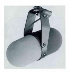
Specifically designed to minimize boom microphone problems in television studio and location applications, the SM-5B is also excellent for radio deejay use. A smooth, wide-range frequency response with moderate presence rise makes it especially suitable for vocal pickup as well as scoring assignments. The SM-5B has a cardioid pickup pattern with exemplary off-axis uniformity, even at
