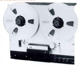
1/4" two channel, half track reproducer with 25 Hz tone sensor, end of message and cuetone relays with adjustable delay (100 milliseconds to 15 seconds). 71/2-33/4 ips speeds. 19" rack mount. Designed for automated broadcast systems and other high reliability reproduce only applications. 15-71/2 ips speeds available on special order.
