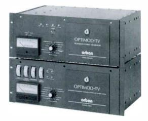
The new, second-generation ORBAN OPTIMOD® TV 8182A. Licensed from CBS TECHNOLOGY CENTER, and incorporating the latest research technology, the in-built loudness controller automatically recognizes program material whose perceived loudness exceeds a certain threshold, then quickly and indiscernably lowers the gain until the loudness is consistent with the rest of the program. The result is smoother more easily-listenable audio, operator errors are corrected and obnoxious commercials are
