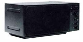
To achieve uncompromising fidelity with plenty of power, one 20-watt amplifier powers the 4½ inch woofer, and a second 5-watt amp drives the efficient 1¾ inch dome tweeter. Since each amplifier functions best within its own portion of the frequency spectrum, the radio's 25-watts are equivalent to over 40 watts from a conventional amplifier. The Schotz variable bandwidth PLL detects or gives a revolutionary and dramatic effect on reception. Optional "ears" available for rack mounting.
