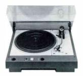
The EMT 938 is a complete turntable system intended for professional applications, consisting of a direct drive turntable, and especially developed shock/insulation mount, the EMT 929 high performance tone arm and built-in equalizer amplifiers for line level audio output.
