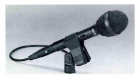
The D-80 is a cardioid dynamic microphone which was designed for both vocal and music applications. It is particularly suited for use with high quality sound reinforcement systems and cassette decks. A foam wind and pop filter eliminates pop and breath noise, as well as wind noise when the microphone is used in the open. ALLIED CARRIES THE ENTIRE AKG MICROPHONE LINE.
