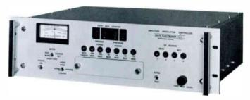
By continuously sampling the modulation levels at the AM transmitter output and comparing these levels with internal preset minimum and maximum modulation thresholds, the AMC-1 Amplitude Modulation Controller detects conditions of under or over modulation. The AMC-1 then uses a digital logic process to adjust the audio level of the transmitter. The audio control circuit is strictly linear so that no compression or asymmetry is added to the program.
