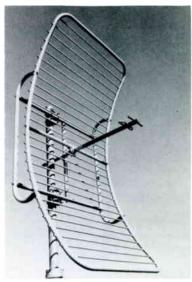
The Scala PR-450-U<sup>™</sup> is widely used in point to point communications and telemetry systems in the 350 to 1000 mHz spectrum. Paraflector<sup>™</sup> performance approximates that of a parabolic dish of the same aperture, and is easier to assemble and install. The PR-450U offers rugged construction for reliable long-term service, even in severe environmental conditions.
