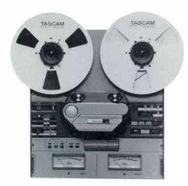
A 2-track ¼'' 2 channel half track mastering and broadcasting recorder/reproducer with +4 XLR/-10 RCA input/output, 10½'' reel capacity, sync capability, full servo and SMPTE interlock capability through an accessory connector. The 52 also features punch in/out recording, pitch control (15% coarse/0.7% fine), manual tach wheel edit, dump edit, search to zero and search to cue and 7½-15 ips speeds.
