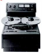
¼" two channel, half track recorder/reproducer with extra quarter track playback head. Includes a microprocessor transport logic and dynamic braking. Zero return. External machine control interface connector for synchronizers or the optional CB-116 auto-locator.
