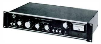
The DBX 165A is a result of combining the 165 and PEAKSTOP. The PEAKSTOP circuit which follows the compressor/limiter circuitry is a specially "soft clipper" that rounds the leading and trailing edges off the peak being clipped. By avoiding the normally sharp edges of a clipped peak, far fewer high order harmonics are generated making PEAKSTOP less audible than other types of clippers.
