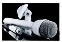
The RE-50 was designed expressly for hand-held ENG. It has the same tailored frequency response and high output level as the famous 635A. The RE-50 rubber shock mount "mike-within-a-mike" design achieves a degree of shock isolation never before known in the industry. The construction is also highly resistant to damage from mechanical shock.
