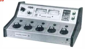
The Model 6509 audio console features five mixing channels, nine mixing inputs, outputs for stereo, mono, monitor, headsets and cue speaker, selectable muting, slotted screw terminal connections, illuminated VU meters. Crosstalk spec'd at -50 dB to -74 dB and distortion is 0.4% Re: +8 dBm output, 800 Hz, hi level input. Package size is 17¾ W x 12¾ D x 6½ H and weighs 16 lbs.
