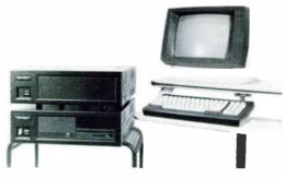
CompuSonics created the DSP-2002 for professional radio and television broadcasting service. Functionally, the DSP-2002 equals or exceeds conventional tape recorders with the additional benefits of digital sound quality, random access and interactive editing. Recording time capacity ranges from 30 to 960 minutes in stereo, depending on the number of Storage Modules installed.
