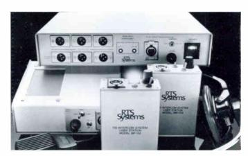
The TW Intercom System is a high performance conference line intercommunications system that features over 30 different components to allow a broad variety of system configurations. The system designed for teleproduction and broadcast operations as well as industrial and commercial applications. Proven performance by demanding professionals has established the TW Intercom System as a standard in the field of intercommunications.
