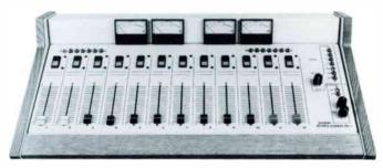
Designed for ease of operation, uncompromising performance and durability, is the 2000SC console. Each of the 12 channels features a single input per channel. Two remote select switches bring in an additional 14 inputs. Cue is accomplished by a detent on the industries finest fader while lighted momentary reed relay switches actuate the program and audition buses which are simultaneously monitored with VU meters. What console could be more rugged in
