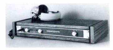
The CROWN D-75 offers significant benefits to the professional user, benefits like IOC input/output comparator that reports all forms of signal overload, lockable level control shafts, active-balanced XLR connectors as well as unbalanced ¼" phone plugs and signal presence indicators that notify the user whenever the D-75 output signal is greater than 1/8 watt. 35 watts per channel.
