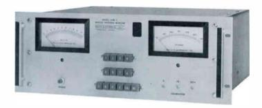
The AAM-1 Analog Antenna Monitor is designed specifically for measuring the parameters of AM broadcast frequency directional antenna systems. The monitor measures the relative current in each tower, the ratio of the current in each tower to that of a reference tower and the phase of the current in each tower relative to that of the reference tower. The AAM-1 can be equipped for up to eight input samples without external switching. Two reference towers can also be selected for DA-2 applications.
