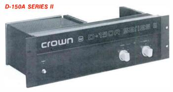
Retaining the D-150A tradition for sonic accuracy and reliability, the CROWN D-150A Series II is rated at 80 watts per channel into 8 ohms, 250 watts into 8 ohms mono. The frequency response is  $\pm 0.1$  dB DC to 20 kHz at one watt into 8 ohms;  $\pm 1$  dB DC to 100 kHz, less than .001% harmonic distortion, less than .01 l.M. distortion and 6 volts per microsecond slew rate.
