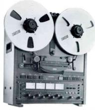
$^{\prime\prime}$  four channel, quarter track recorder/reproducer. DC-servo capstan with  $\pm 7\%$  vari-speed. 15-7 $^{\prime\prime}$ 2 ips speed.  $\pm 4$  or -10 dB input/output level select. Real time tape counter with LED display. Zero return. Headphone output with channel select. Test oscillator (1kHz or 10 kHz). Microprocessor controlled transport logic. Dynamic braking. Integral splicing block. External machine control interface connector for synchronizers.
