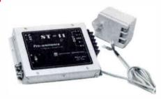
The ST-11 Pro-eminence phono pre-amp by Micro-Track is a super high performance unit. It is RFI resistant for use in AM, FM or TV. It is very compact and designed to match a 47K ohm magnetic stereo phono cartridge. Provision for a nominal 0 dBm output with headroom to a max. of +22 dBm. Distortion is .05 or less, THD and IM. The signal to noise ratio is -72 dB or better, also has a jumper selectable rumble filter internally.
