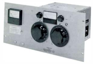
The Common Point Impedance Bridge is an invaluable device for directional array maintenance. The CPB-1 is designed for permanent installation in existing phasing equipment to provide an accurate indication of the common point impedance. The CPB-1 will handle common point powers of up to 5 kW with 100% modulation. The CPB-1A is designed for powers up to 50 kW.
