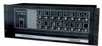
The new PRIMUS RS-1616 is an audio thru data routing/amplifying system with performance and versatility unmatched by any similar units on the market. In addition to performance that will surpass the requirements of even the most critical studio professional, the user friendly controls (local front panel, remote 4 bit binary, common 3 wire serial, or standard RS-232 personal computer control) provide you with the power to program or control these units, limited only by your imagination.
