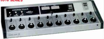
The Model 6510 features ten mixing channels, fourteen inputs, stereo or mono, selectable muting switch, relays for "on-the-air" lights, high quality VU meters, VCA attenuators, plug-in printed circuit cards and switches for easy maintenance, pushbutton input selector switches, barrier terminal strip input and output terminations, monitor output at line level, sealed main pots and compact desian.
