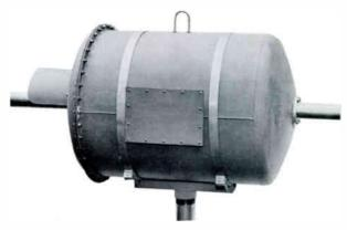
ERI isolation transformers are designed to couple the FM power across the base insulator of a transmitting tower used jointly for AM or FM antennae without introducing objectionable mismatch into the FM feed line.
