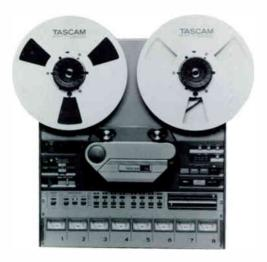
An 8-track ½" 8 channel production recorder/reproducer with -10 RCA input/output, 10½" reel capacity, full frequency response in sync mode, full servo, SMPTE interlock capability through an accessory connector and punch in/out recording. The 58 also features pitch control (15% coarse/0.7% fine), manual tach wheel edit, dump edit, search to zero and search to cue and 15 ips speed.
