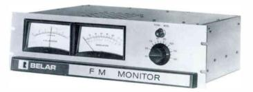
Belar FM monitors are designed as a totally integrated, solid-state system to enable the broadcaster to fulfill his monitoring equipment requirements as the need arises. The FMM-1 Frequency and Modulation Monitor is a wideband, all solid-state FM monitor expressly designed to fulfill all the requirements for monaural monitoring as well as to provide a virtually pure, distortionless signal to drive the companion FMS-1 and SCM-1 for multiplex monitoring.
