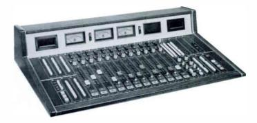
The 200 series on-air broadcast control console represents the culmination of latest technology applied for broadcast use. The design is based on information gathered during extensive research conducted throughout the broadcast industry and the expertise of Auditronics 15-year history in this business. The 200 series offers a high degree of reliability together with simplicity of use in a compact, operator oriented package.
