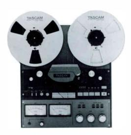
A 2-track 1/4" 2 channel half track mastering and broadcasting recorder/reproducer with 10½" reel capacity, sync capability, full servo, SMPTE interlock capability through accessory connector and punch in/out recording. The 42 also features NAB or IEC equalization, dump edit, search to zero and search to cue, 71/2-15 ips speeds and +4/-10 input/output.
