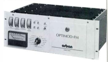
The ORBAN 8100A FM OPTIMOD® offers wideband or multiband operation, more versatile setup controls that permit precise "tuning" for different formats, improved voice/music balances, an improved stereo generator with cleaner baseband, new overshoot compensation that permits full modulation at all frequencies, yet doesn't increase low frequency IM distortion, plus a dual-chassis option, built-in crosstalk test generator, rigorous RFI shielding and true VC gain control. FM's favorite processor!
