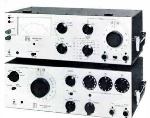
Designed primarily for commercial broadcast proof-of-performance measurements and equipment maintenance. The AG-51 Audio Generator and AA-51 Audio Analyzer are packaged separately for remote measurements requiring physical separation of signal source and signal analyzer. Both units are RFI shielded to enable accurate measurements in high level radio frequency environments typical of broadcast transmitter facilities. Signal input and output connectors are also RFI shielded.
