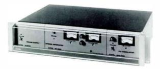
The SM2200 Stereo Generator consists of a sub-carrier oscillator, balanced modulator and channel amplifier, packaged in a modular unit for use with the FMX-2200S.
