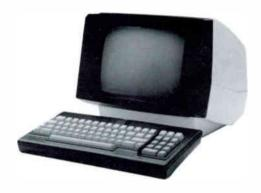
Option for cathode-ray tube (CRT) Terminal. Duplicates all panel functions of the MRC-1600 Control Terminal. Allows simultaneous display for 16 channels, including telemetry readings, status conditions, time of day, operation and error-oriented messages.
