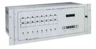
Microprocessor Remote Control System, consisting of one Control Terminal, one Remote Terminal. System is equipped with 32 command relays, 16 status channels (TTL/contact closure), and 16 digital telemetry channels. FCC acceptable for AM and FM broadcast transmitter remote control. Includes audible telco/telco data interface on each terminal.
