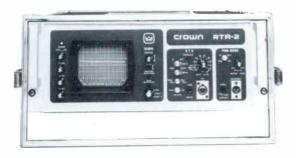
The Crown RTA-2 is designed for audio-range real-time spectrum analysis in ½ and full octave bands. All the sub-systems needed to perform quick, accurate on-site equalization of sound-reinforcement systems are included in the RTA-2.
