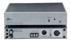
The Model 465 is a single channel, wideband microphone preamp designed for pro use in areas such as broadcast operations, television production, sound reinforcement and more. It features outstanding electrical specifications along with fully floating transformer balanced input and output circuits, switchable phantom power and an integral power supply. The 465 employs a switchable limiter to preclude the possibility of preamp overload from any mic source.
