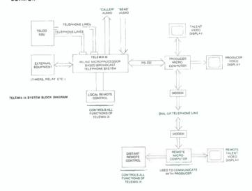
In summary, TELEMIX IX is a software driven, microprocessor based, multi-line telephone system that provides high quality telephone audio. The sytem is software driven, allowing maximum flexibility in processing telephone lines. The RS-232 port permits long distance remotability and in-house programming via a minicomputer. The system uses an advanced design telephone hybrid that produces produces clean, clear audio.
