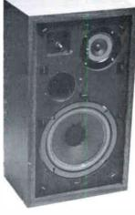
The MONITOR loudspeaker system provides a flat response from below 50 Hz to beyond 20 kHz. Its high compliance surround on the 8" woofer and phenolic tweeter combine to enhance any type of music. The tweeter control and the system fuse are behind the snap-away grille. It will handle 25 watts RMS continuous, 45 watts integrated program material at 8 ohms.
