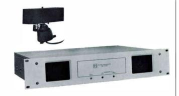
The SMR-11 is an AM broadcast band receiver of superior performance with many capabilities useful to the broadcaster. Receive tuning is continuous from 530 to 1700 kHz, and can be locked with crystal accuracy at any desired frequency. The antenna can be a remotely located tunable ferrite rod unit (ANT-11), broadband wire or a whip. Bandwidth is determined by two switch-selected 455 kHz ceramic filters with bandwidths of 28 kHz and 12 kHz. Other special filters are available and can be installed.
