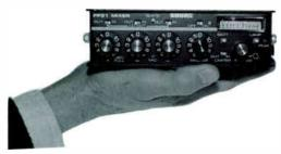
The Model FP-31 is a compact, portable microphone mixer specially designed for electronic news gathering (ENG) and electronic field production (EFP) use including film, video and remote broadcast applications. The FP-31 provides a wide, flat frequency response, low distortion, and up to +18 dBm output. The unit features extremely low internal noise and switchable low-cut filters for each input that effectively reject low-frequency handling and wind noise. 400 Hz slate tone, 1 kHz cue tone.
