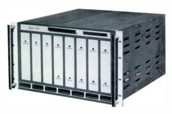
For Digital Satellite reception we recommend the FAIRCHILD DART 384 (formerly known as the COMTECH DART 384). The DART 384 receiver consists of down-converter, receiver-demodulator shelf, audio program channels, voice cue channels, and data program channels.
