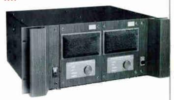
As opposed to the "fix-it-up-with-feedback" approach in common use today, UREI carefully departed from conventional design techniques. Each amplifier stage in the 6500 was engineered for optimum performance with no overall feedback. The 6500 features two channels on an independent, modular plug-in chassis with front panel access. The 6500 is rated at 275 watts into 8 ohms per channel output with .1 THD.
