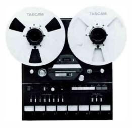
An 8-track ½" recorder/reproducer with 8 tracks on ½" tape, 10½" reel capacity, 15 ips speed, ±12% pitch control and function and output select. The 38 also features punch in/out recording, dump edit, cue control, FL tape counter and zero return.
