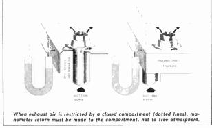
METHODS OF MEASURING PRESSURE DIFFERENTIAL
