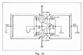
rig. 10 Screen-tuning neutralization circuit for use above 100 Mc. with 4-125A tetrode.
