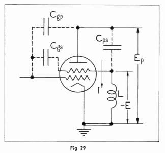
Tetrode characteristics involved in feedback circuit.
