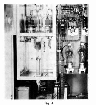
rig. \* Push-pull 110 Mc. amplifier employing 4-1000A tetrodes. Gates Radio Co. Model BF 3 kw trasmitter.
