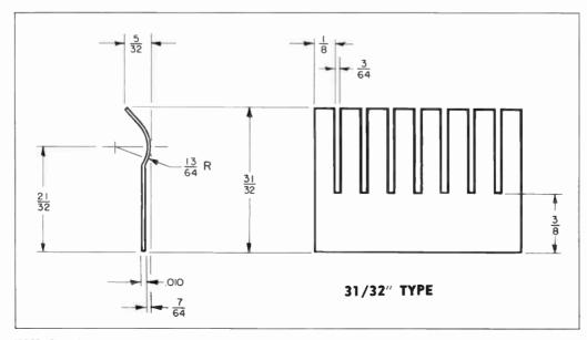
NOTE---The above dimensions should be regarded as carrying normal manufacturing tolerances because of variations in the shearing, forming and heat-treating processes.
