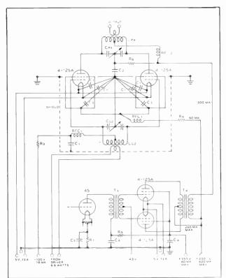
Typical high-level-madulated r-f amplifier circuit, with madulatar and driver stages, 380 watts plate input.
