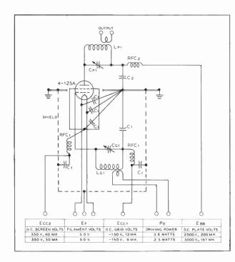
Typical radia-frequency pawer amplifier circuit, Class-C telegraphy, 500 watts input.
