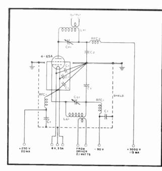
Typical radio-frequency power amplifier circuit, Class-C telegraphy, 345 watts input.
