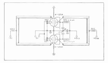
Screen-tuning neutrolization circuit for use above 100 Mc. C is a small split-stator capacitor.
