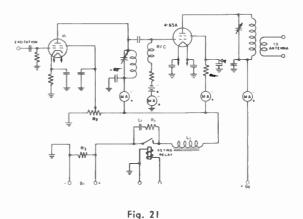
Tetrode amplifier keying circuit used by B. O. Ballou (W6BET)<sup>2</sup>.
