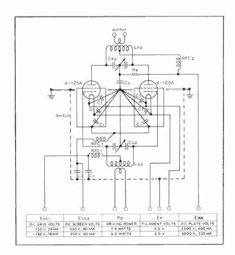
Typical radia-frequency pawer amplifier circuit, Class-C telegraphy, 1000 watts input.
