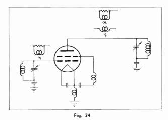
Placement of parasitic suppressors to eliminate VHF parasitic oscillations in HF r-f amplifiers.
