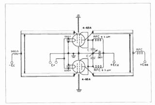
Screen-tuning neutralization circuit for use abave 100 Mc. C is a small split-statar capacitor. 640,000
