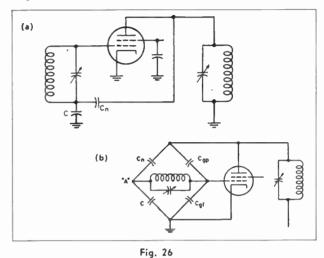
Single-ended grid neutralization described by Bruene<sup>6</sup>. a) Basic Circuit. b) Arranged as capacitance bridge.
