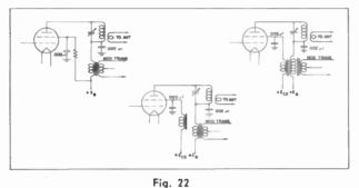
Basic high-level-modulating circuits for tetrodes.
