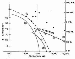
Fig. 2—Curve (1): Efficiency versus frequency for typical uhf tetrode —4X150G. (Plate dissipation 150 watts.) Curve (2): Efficiency versus frequency for typical uhf triode
