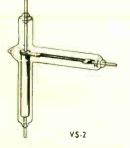
A single pole, double throw switch with contacts in high vacuum for high voltage switching. Contact spacing .015". Switch will handle r-f potentials as high as 20 Kv. In DC switching will handle approximately 1.5 amps. at 5 Kv.
