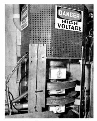
Fig. 8-The 5-kw klystron on test.
