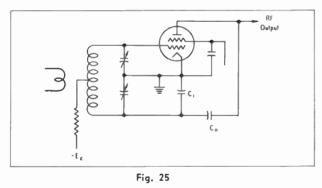
Push-pull grid neutralization, basic circuit.
