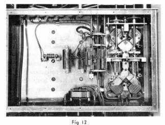
Underside of push-pull multi-band r-f amplifier employing 4-250A tetrodes. Designed and built by C. F. Bane (W6WB)<sup>3</sup>.
