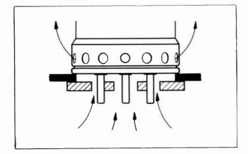
4-125A mounting providing base cooling, shielding and isolation of output and input compartments.
