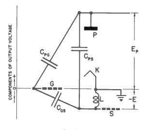
Fig. 30 Graphical presentation of components of output circuit voltages in tetrode when self neutralized.
