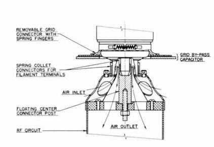
TYPICAL TUBE CONNECTORS AND STEM COOLING
