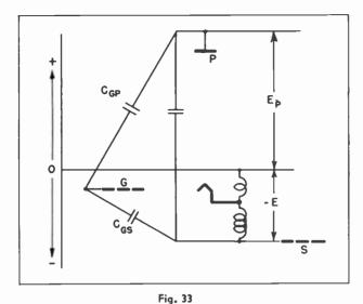
Components of output voltage of a tetrode neutralized by adding inductance common to screen and cathode return.
