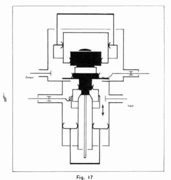
Schematic cavity section of 1250 Mc., amplifier employing 4X150G tetrode.
