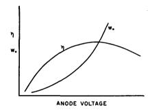
Fig. 5—Power output and efficiency versus anode voltage.
