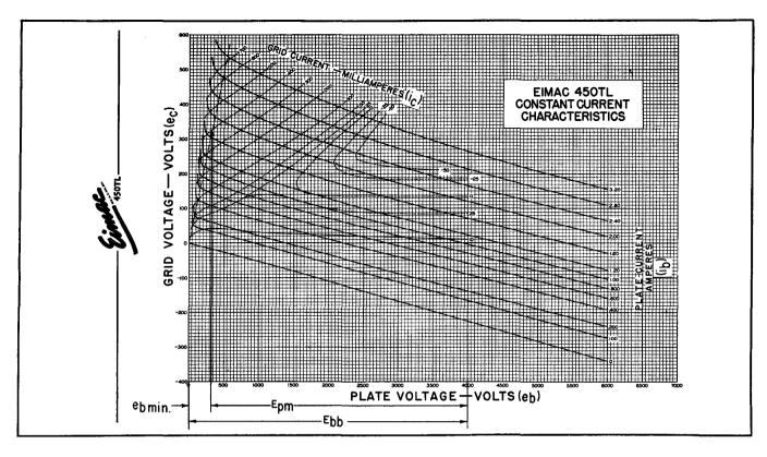
Figure 2. 450TL constant-current characteristics showing method of determining  $\mathbf{e}_{\mathrm{bm\,in}}$  and  $\mathbf{E}_{\mathrm{pm}}$  in steps 6 and 7 from value of  $\mathbf{i}_{\mathrm{b}}$  obtained in step 5.
