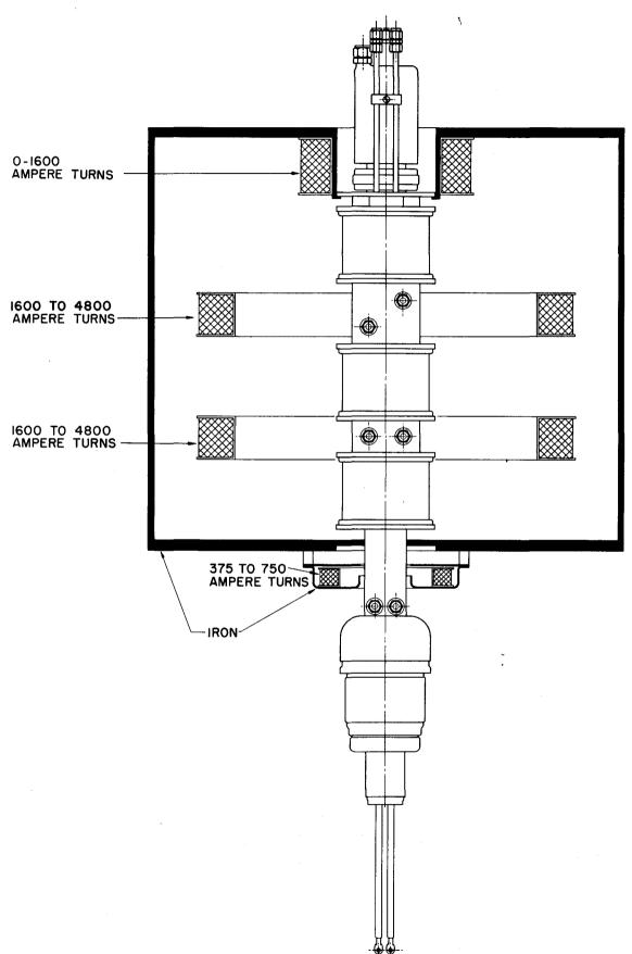
MAGNETIC CIRCUIT SCHEMATIC FOR 3K20,000LK
