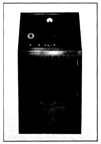
FIG. I—Front view of the experimental crystal-controlled diathermy unit. Apparatus on the panel includes, autotransformer control, PA plate meter, output tuning control, interval timer, PA plate tuning control, output jacks, output indicator lamp, oscillator and doubler tuning controls (screwdriver adjustment), power switches and pilot lamps.
