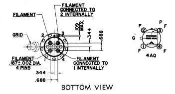
NOTE:—The grid terminal on the new 450TH and TL type tube is now .563" in diameter. To accommodate existing equipment which uses the 450TH or TL tubes with the old style .098" grid terminal, an adapter pin is provided. This adapter pin, if not needed, may be removed by unscrewing.
