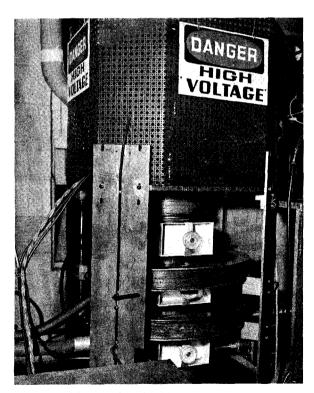
Fig. 8-The 5-kw klystron on test.
