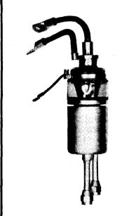
The water-cooled anode requires one gallon of cooling water per minute for the rated plate dissipation of 5 kilowatts. The outlet water temperature must not exceed a maximum of 70°C. under any conditions. The inlet water pressure must not exceed a maximum of 60 pounds per square inch. The pressure drop across the anode is negligible compared to the drop in the associated piping.
