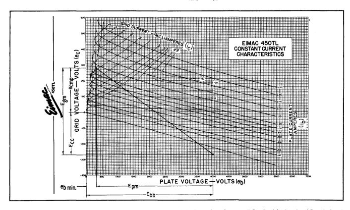
Figure 3. Method of determining  $\mathbf{e}_{emp}$  and  $\mathbf{i}_{e}$  on 450TL constant-current characteristics from values of  $\mathbf{e}_{bmin}$  and  $\mathbf{E}_{pm}$  found in steps 6 and 7 and value of  $\mathbf{i}_{b}$  found in step 10. The value of  $\mathbf{E}_{ec}$  and  $\mathbf{E}_{gm}$  from steps 13 and 14 and the operating line are also shown.
