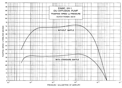
The curves at the left show the gas handling capabilities of the HV-I over a range of pressures both with and without a baffle. These curves apply when a forepump with the required capacity is used. The rapid loss in pumping speed at the higher pressures is due to the inability of the forepump to handle the necessary volume of gas. With a larger forepump, the pumping speed would be maintained out to higher pressures.
