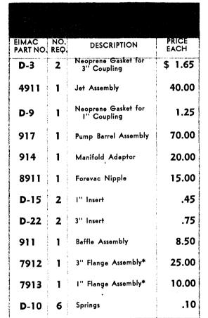
\*Each flange assembly includes necessary flanges, gaskets, inserts, bolts and hardware.
