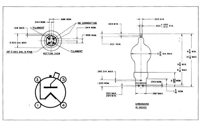
The Eimac 253 is a high-vacuum diode rectifier intended for use in rectifier units, voltage multipliers, or in special applications, whenever conditions of extreme ambient temperatures, high operating frequency, high peak inverse voltages, or the production of high-frequency transients would prevent the use of gas-filled rectifier tubes.
