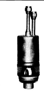
The water-cooled anode requires one gallon of cooling water per minute for the rated plate dissipation of 5 kilowatts. The outlet water temperature must not exceed a maximum of 70°C, under any conditions. The inlet water pressure must not exceed a maximum of 60 pounds per square inch. The pressure drop across the anode is negligible compared to the drop in the associated piping.
