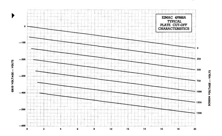
PLATE VOLTAGE — KILOVOLTS
