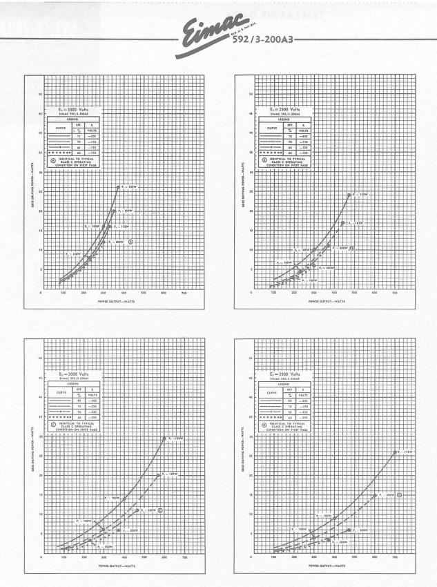
The four charts on this page show the relationship of plate efficiency, power output and grid driving power at plate voltages of 2000, 2500, 3000 and 3500 volts. These charts show combined grid and bias losses only. The driving power and power output figures do not include circuit losses. The plate dissipation in watts is indicated by  $P_p$ .
