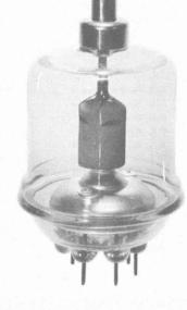
The Eimac 4-65A is a small radiation-cooled transmitting tetrode having a maximum plate dissipation rating of 65 watts. The plate operates at a red color at maximum dissipation. Short, heavy leads and low interelectrode capacitances contribute to stable efficient operation at high frequencies.
