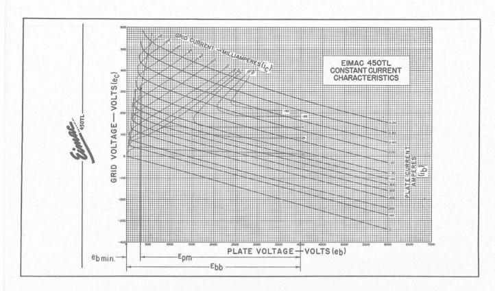
Figure 2. 450TL constant-current characteristics showing method of determining e<sub>bmin</sub> and E<sub>pm</sub> in steps 6 and 7 from value of i<sub>b</sub> obtained in step 5.
