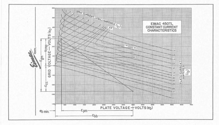
Figure 3. Method of determining e<sub>emp</sub> and i<sub>e</sub> on 450TL constant-current characteristics from values of e<sub>bmin</sub> and E<sub>pm</sub> found in steps 6 and 7 and value of i<sub>b</sub> found in step 10. The value of E<sub>ce</sub> and E<sub>gm</sub> from steps 13 and 14 and the operating line are also shown.
