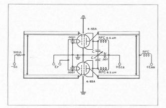
Screen-tuning neutralization circuit for use above 100 Mc. C is a small split-stator capacitor.  $C(_{uufd}) = \frac{640,000}{f^{\epsilon} (Mc.)}$ , approx.
