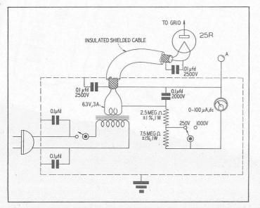
Figure 1. Peak vacuum tube voltmeter for making  ${\sf E}_{
