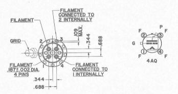
NOTE:—The grid terminal on the new 450TH and TL type tube is now .563" in diameter. To accommodate existing equipment which uses the 450TH or TL tubes with the old style .098" grid terminal, an adaptor pin is provided. This adaptor pin, if not needed, may be removed by unscrewing.
