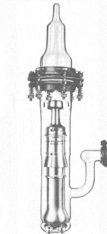
The Eimac HV-1 Diffusion Pump is a fast, triple-jet, aircooled vacuum pump of the oil-diffusion type. When used with a suitable mechanical forepump and Eimac type A oil it is capable of reaching an ultimate vacuum of  $4 \ge 10^{-7}$  mm of mercury.
