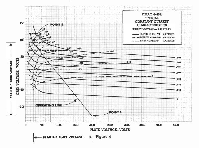
Where OB crosses the operating line the plate current is also 500 ma. At OC the plate current is about 450 ma, OD 300 ma, OE 90 ma, OF and OG 0 ma. Similarily we can see that the instantaneous screen current at the crossing of OA and the "Operating Line" is 200 ma, and the instantaneous grid current is almost 80 ma. Values are read for the other crossings and written down. These values are put in simple columns for calculating:
