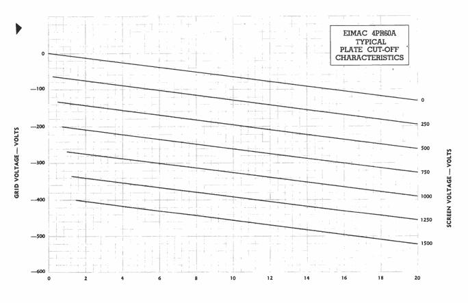
PLATE VOLTAGE - KILOVOLTS
