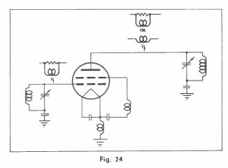
Placement of parasitic suppressors to eliminate VHF parasitic oscillations in HF r-f amplifiers.
