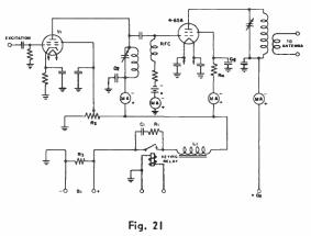
Tetrode amplifier keying circuit used by B. O. Ballou (W6BET)<sup>2</sup>.
