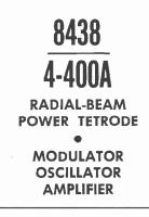
The EIMAC 8438/4-400A is a compact, ruggedly constructed power tetrode having a maximum plate dissipation rating of 400 watts. It is intended for use as an amplifier, oscillator or modulator. The low grid-plate capacitance of this tetrode coupled with its low driving-power requirement allows considerable simplification of the association circuit and driver stage.
