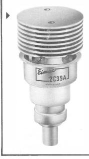
The Eimac 2C39A is a ceramic-metal high-mu planar triode with a platedissipation rating of 100 watts, designed for use as a power amplifier, oscillator, or frequency multiplier at frequencies to above 2500 megacycles. The new ceramic-metal construction results in extreme ruggedness, mechanical uniformity, reliable operation at seal temperatures up to 250°C, and longer life expectancy than its glass prototypes.
