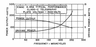
**Closs-C AM Telephony**—The R-F circuit considerations discussed above under Class-C FM or Telegraphy also apply to amplitude-modulated operation of the 4-65A. When the 4-65A is used as a class-C high-level-modulated
