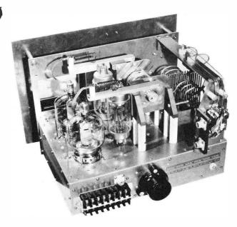
Fig. 2 Push-pull r-f amplifier employing 4-250A tetrodes. Designed and built by C. F. Bane (W6WB)<sup>5</sup>.
