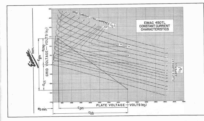
Figure 3. Method of determining e<sub>emp</sub> and i<sub>e</sub> on 450TL constant-current characteristics from values of e<sub>bmin</sub> and E<sub>pm</sub> found in steps 6 and 7 and value of i<sub>b</sub> found in step 10. The value of E<sub>ee</sub> and E<sub>gm</sub> from steps 13 and 14 and the operating line are also shown.
