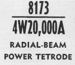
The Eimac 8173/4W20,000A is a high-power, water-cooled transmitting tetrode having a maximum plate dissipation rating of 20 kilowatts. This tube will operate efficiently as a power-amplifier at frequencies up to 250 Mc. A single 8173/4W20,000A operating as a television visual r-f amplifier will deliver a synchronizing power output of 26 kilowatts at 216 Mc., with a 5-Mc. bandwidth.
