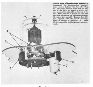
Fig 11 Eimac 4-400A/4000 Air System Socket providing balanced tube cooling by a single stream of air.
