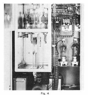
Push-pull 110 Mc, amplifier employing 4-1000A tetrodes. Gates Radio Co. Model BF 3 kw trasmitter.
