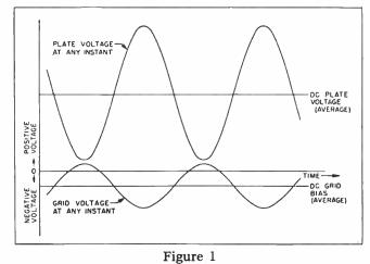
has a value which is the point marked "eg" on the gridvoltage sine wave. If one now finds the point on the tube curves corresponding to these values (where a line drawn from "eg" and a line drawn from "ep' cross) he will be at point A in Fig. 2. As the values of grid volt-age "eg" and plate voltage "ep" vary over the r-f cycle, the point A moves up and down a line, which in the case of the normal r-f power amplifier is a straight line. This line is called the "Operating Line."
