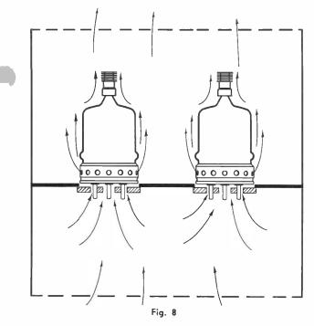
4-125A mounting providing cooling, shielding and isolation of output and input compartments.
