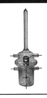
The filament temperature of the 100 IG must be low enough so that the emission is temperaturelimited. With a good vacuum, the filament voltage will be between 2.0 and 4.0 volts, and the filament current will be approximately 8.0 amperes. With a poor vacuum, it will be necessary to increase the filament voltage to approximately 7.5 volts, and the current will be about 12 amperes. (The tube should not be operated long at high filament voltage.)
