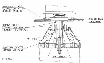
TYPICAL TUBE CONNECTORS AND STEM COOLING
