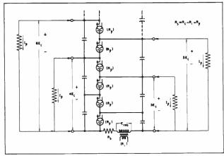
e. Half-Wave Voltage Multiplier (with common ground when R<sub>s</sub> is inserted on the "high" side of E<sub>rms</sub>)
