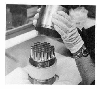
Final Assembly of VacCap\* Variable Vacuum Capacitor
