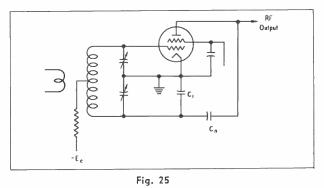
Push-pull grid neutralization, basic circuit.
