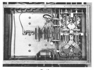
Fig 12 Underside of push-pull multi-band r-f amplifier employing 4-250A tetrodes. Designed and built by C. F. Bane (W6WB)<sup>5</sup>.
