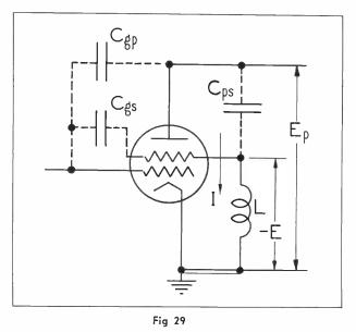
Tetrode characteristics involved in feedback circuit.
