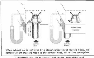
METHODS OF MEASURING PRESSURE DIFFERENTIAL
