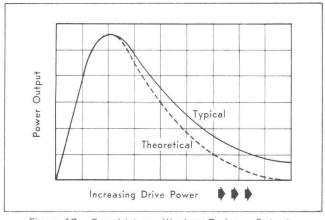
Figure 17—Overdriving a Klystron Reduces Output.
