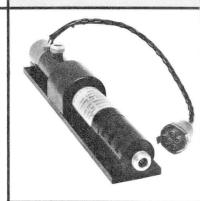
The EM-1016 features rugged ceramic and metal construction and focusing is provided by built-in periodic permanent magnets. These magnets are fully temperature compensated to allow operation from  $-55^{\circ}\text{C}$  to  $+85^{\circ}\text{C}$ . No additional cooling is required at these temperatures due to the integral heat sink/mounting flange supplied with the tube.
