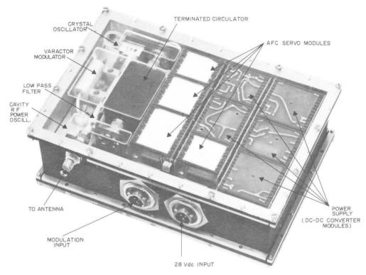
EM4534 TELEMETRY TRANSMITTER ASSEMBLY
