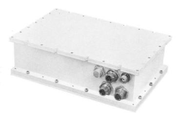
Model EM4567 is a complete transmitter, including a pre-regulated DC-DC converter. All circuits are solid state, except the rf power oscillator, which is a single stage rugged ceramic planar triode. RF is generated at the output frequency. The complete transmitter is packaged in less than 110 cubic inches, and weighs less than 8 pounds. Modulation is true FM. Major features of this transmitter include:
