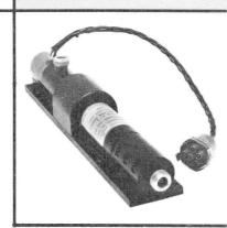
The EM-1011 features rugged ceramic and metal construction and focusing is provided by built-in periodic permanent magnets. These magnets are fully temperature compensated to allow operation from  $-55^{\circ}\text{C}$  to  $+~85^{\circ}\text{C}$ . No additional cooling is required at these temperatures due to the integral heat sink/mounting flange supplied with the tube.
