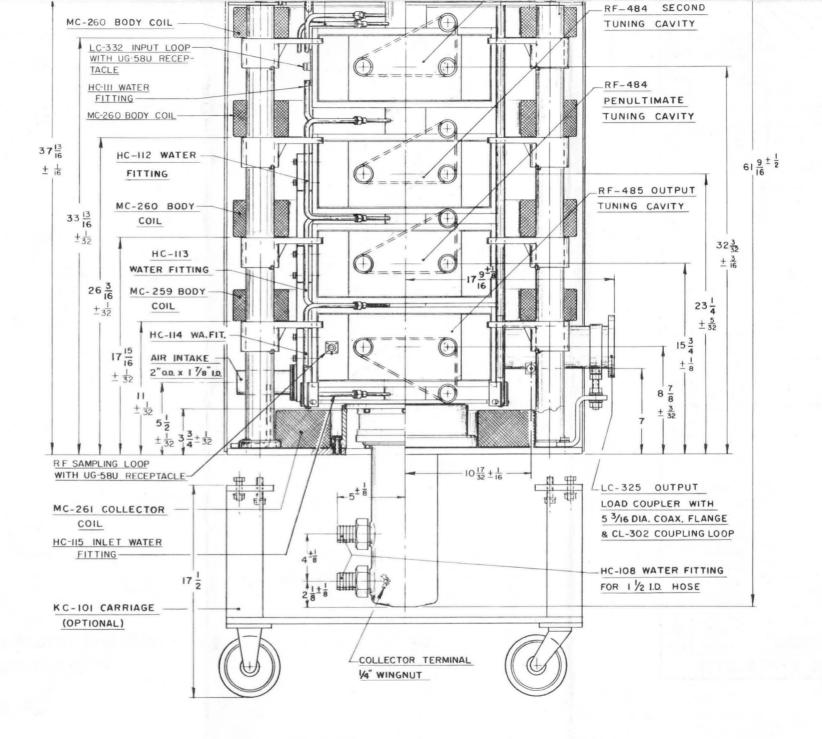
H-I33 KLYSTRON AMPLIFIER CIRCUIT ASSEMBLY
