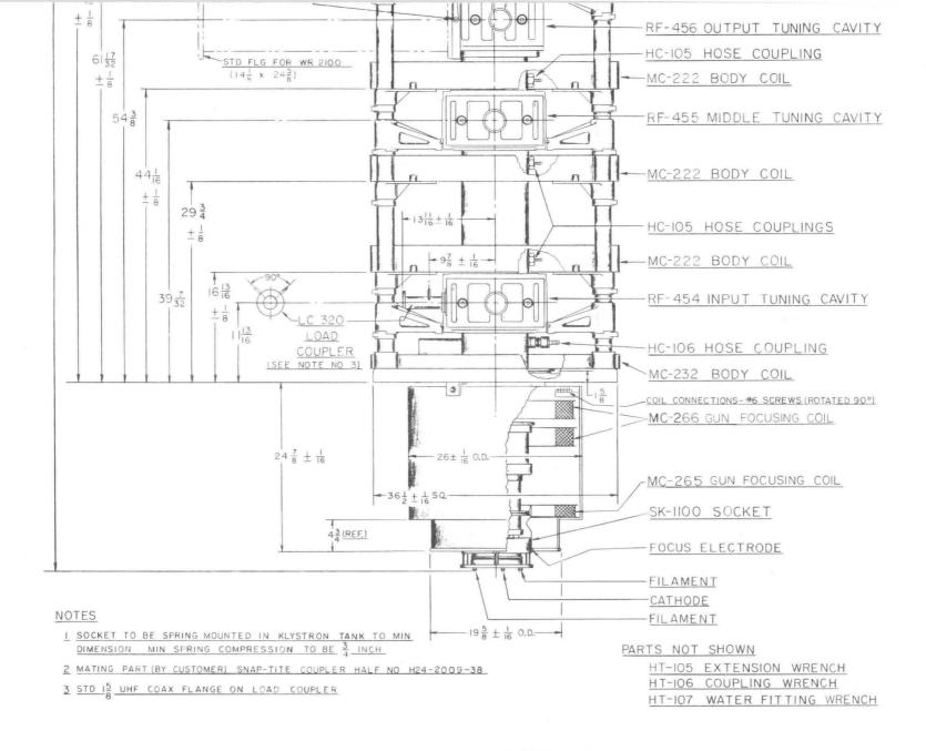
H-123B KLYSTRON AMPLIFIER CIRCUIT ASSEMBLY
