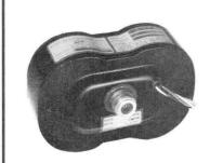
The extremely linear tuning characteristic of this magnetron simplifies programming and frequency sweep, by eliminating the complicated compensating networks required by other voltage tunable oscillators. In addition, the injection anode may be programmed to provide some leveling action on the output power during the frequency sweep.
