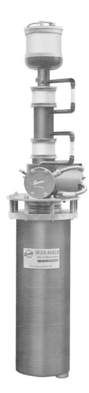
Eimac 3K210,000LQ. This 75 kW klystron is used in many tropo-scatter systems spanning distances up to 440 miles. This klystron is unique in that its input and penultimate cavities are external but its output cavity is integral.
