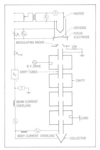
Figure 20—Klystron Power Supply Connections
