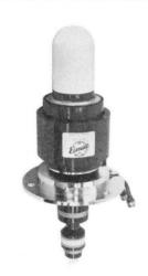
Anode voltage for the EM15LS is normally supplied from a full wave three-phase rectifier with or without filter choke. The degree of filtering in any particular application is dictated by the permissible amplitude and frequency modulation of the rf output power. These are mainly determined by the anode current ripple.
