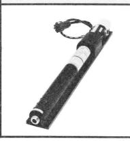
The EM-1050 features rugged ceramic and metal construction and focusing is provided by built-in periodic permanent magnets. These magnets are fully temperature compensated to allow operation from -55 to  $+85^{\circ}$ C. No additional cooling is required at these temperatures due to the integral heat sink/mounting flange supplied with the tube.
