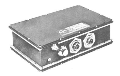
Model EM 4527 is a complete transmitter, including a pre-regulated DC-DC converter. All circuits are solid state, except the rf power oscillator, which is a single stage rugged ceramic planar triode. RF is generated at the output frequency. The complete transmitter package displaces less than 50 cubic inches, and weighs 4 pounds. Major features of this transmitter include:
