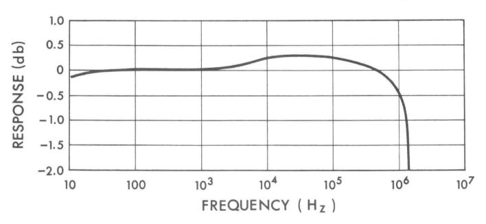
TYPICAL MODULATION FREQUENCY RESPONSE OF TRANSMITTER
