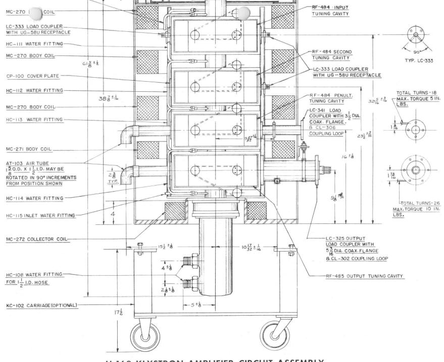
H-163 KLYSTRON AMPLIFIER CIRCUIT ASSEMBLY
