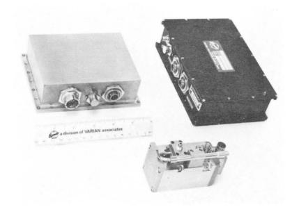
Model X4528 is a complete transmitter. It includes an exciter, a power amplifier and a preregulated dc-dc converter. All circuits are solid state, except the rf power oscillator and the power amplifier; these use rugged ceramic planar triodes. RF is generated at the output frequency, and stabilized by a crystal-referenced AFC servo circuit. Major features of this transmitter include:
