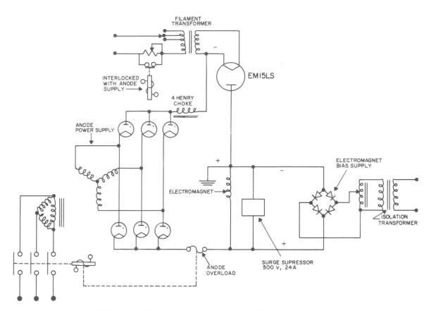
ELEMENTARY CIRCUIT FOR OPERATION WITH SERIES FIELD  $$\operatorname{\sc fig.}\,4$$
