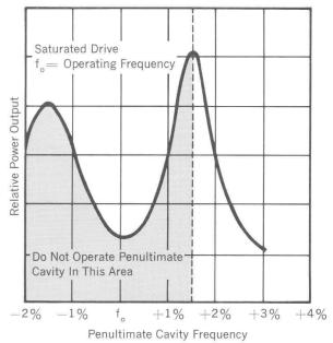
Figure 18—Penultimate Cavity Tuning
