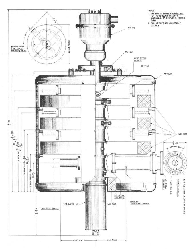
H-101A KLYSTRON AMPLIFIER CIRCUIT ASSEMBLY
