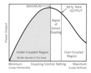
Figure 19—Adjustment of Output Coupling Control.
