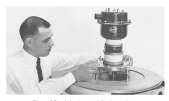
Figure 16—Adjustment of Prefocus Coil.
