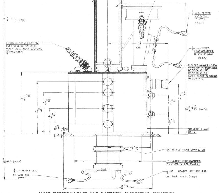
H-158 ELECTROMAGNET AND KLYSTRON SUPPORTING STRUCTURE
