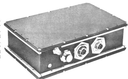
Model EM4534 is a complete transmitter, including a pre-regulated DC-DC converter. All circuits are solid state, except the rf power oscillator, which is a single stage rugged ceramic planar triode. RF is generated at the output frequency. The complete transmitter package displaces less than 50 cubic inches, and weighs 4.5 pounds. Major features of this transmitter include:
