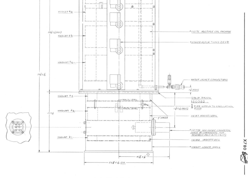
H-145 KLYSTRON AMPLIFIER CIRCUIT ASSEMBLY
