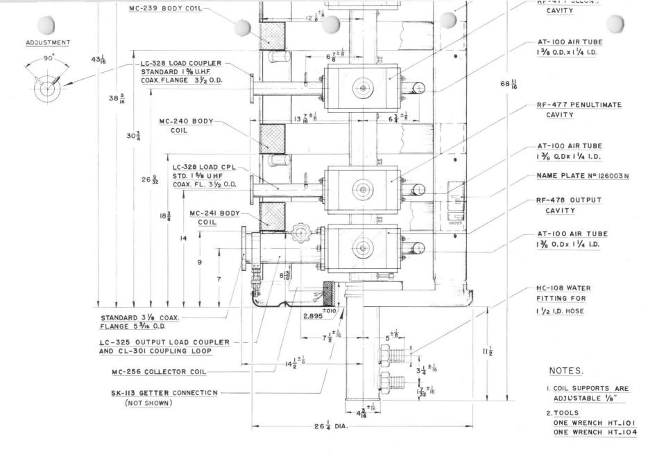
H-139 KLYSTRON AMPLIFIER CIRCUIT ASSEMBLY
