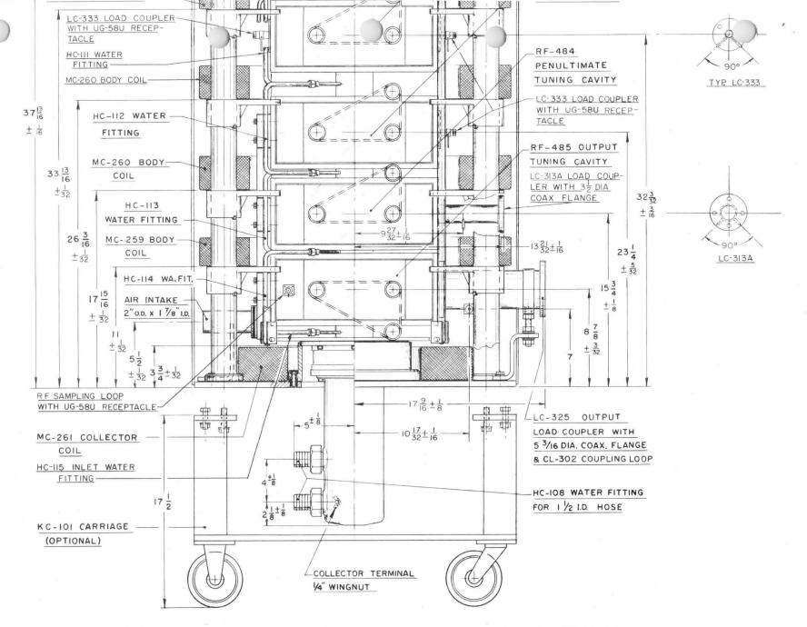
H-133 KLYSTRON AMPLIFIER CIRCUIT ASSEMBLY
