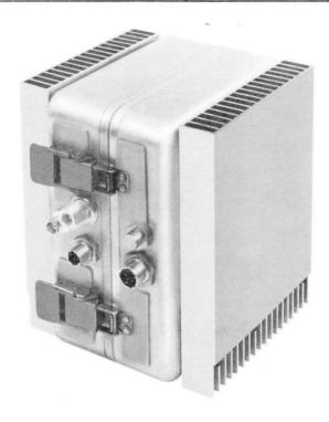
Model EM4575 is a complete transmitter, including a 400 CPS 115V power supply. All circuits are solid state, except the rf power oscillator, which is a single stage cavity using a rugged ceramic planar triode. RF is generated at the output frequency. The complete transmitter is packaged in less than 300 cubic inches, and weighs less than 11 pounds. Major features of this transmitter include:
