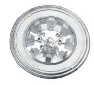
Normally the ceramic chimney SK-606 is used with these two sockets to direct the cooling air past the body of the tube as it flows from pressurized chassis through the socket, then through the tube anode fins. Reverse air direction may be used. (Type 8930 uses Chimney SK-646).
