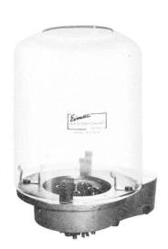
The electrical insulation for the connecting jacks and their terminals is a disk of low-loss insulating material, resting on a shoulder turned into the bottom of the socket body. The insulating disk is held in place by four machine screws which act as clamps. The design permits the insulation and terminal assembly to be rotated to any convenient direction and clamped firmly in place, so no compromise with wiring requirements will have to be made when the socket is installed.
