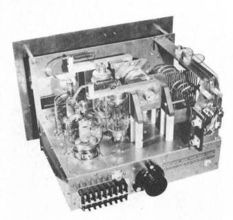
Fig. 2 Push-pull r-f amplifier employing 4-250A tetrodes. Designed and built by C. F. Bane (W6WB)<sup>4</sup>.
