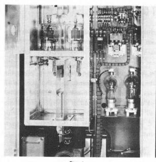
Fig. 4 Push-pull 110 Mc. amplifier employing 4-1000A tetrodes. Gates Radio Co. Model BF 3 kw trasmitter.
