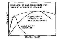
Fig. 4—Efficiency versus driving power, showing the effect of detuning the middle cavity.
