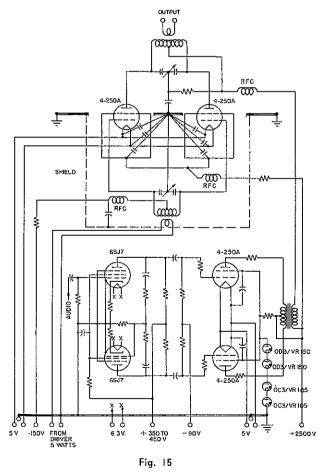
Typical high-level-modulated r-f amplifier circuit with modulator and driver stages, 1000 watts input.
