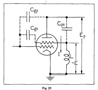
Tetrode characteristics involved in feedback circuit.
