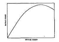
Fig. 3-Output power versus driving power for klystron.
