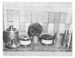
Fig. 7-Tube cavity parts and drift tube sections.
