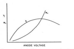
Fig. 5-Power output and efficiency versus anode voltage.
