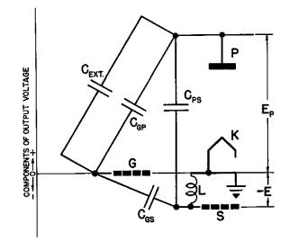
Fig. 31 Components of output voltage of a tetrode when neutralized by added series screen-lead capacitance.
