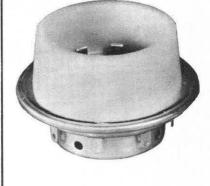
**MOUNTING**—If the tube and socket are to be used in a coaxial-line circuit, the Air-System Socket may be mounted directly on the end of the coaxial input line. The skirt of the socket fits over a cylinder of 1% " outside diameter, and four mounting holes are provided (See Outline Drawings).
