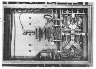
Fig 12 Underside of push-pull multi-band r-f amplifier employing 4-250A tetrodes. Designed and built by C. F. Bane (W6WB)<sup>4</sup>.
