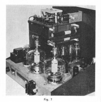
Experimental 500 watt Class-AB, audio amplifier. Designed and built by Eitel-McCullough Laboratories'.
