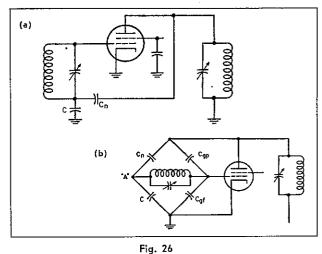
Single-ended grid neutralization described by Bruene<sup>s</sup>. a) Basic Circuit. b) Arranged as capacitance bridge.
