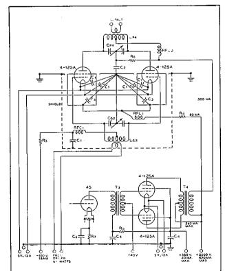
Typical high-level-modulated r-f amplifier circuit, with modulator and driver stages, 380 waits plate input.
