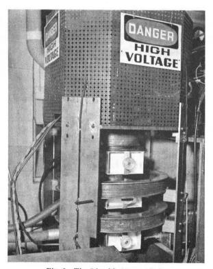
Fig. 8—The 5-kw klystron on test.
