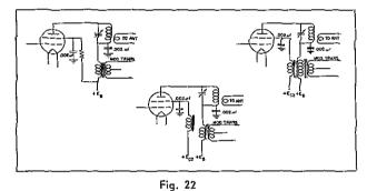
Basic high-level-modulating circuits for tetrodes.
