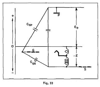
Components of output voltage of a tetrode neutralized by adding inductance common to screen and cathode return.
