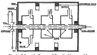
Fig. 1---Schematic diagram of 3-cavity klystron with magnetic focusing.
