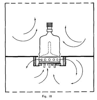
DO NOT SUB-MOUNT A METAL BASE SHELL TUBE. Base cooling is prevented and no improvement in shielding results.
