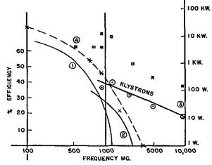
Fig. 2—Curve (1): Efficiency versus frequency for typical uhf tetrode --4X150G. (Plate dissipation 150 watts.)
