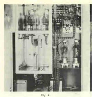
Push-pult 110 Mc. amplifier employing 4-1000A tetrodes. Gates Radio Co. Model BF 3 kw trasmitter.
