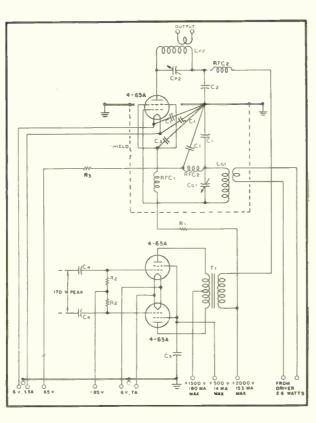
Typical high-level-modulated R-F amplifier, 240 watts plate input. Modulator requires zero driving power.
