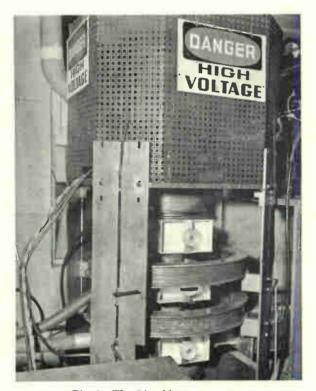
Fig. 8-The 5-kw klystron on test.
