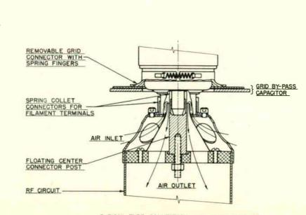
TYPICAL TUBE CONNECTORS AND STEM COOLING
