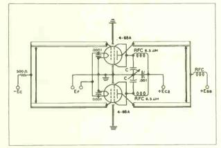
Screen-tuning neutralization circuit for use above 100 Mc. C is a small split-stator capacitor.  $C(_{\mu\mu}fd) = \frac{640,000}{f^2 (Mc.)}, \text{ approx.}$
