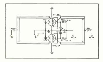
Screen-tuning neutralization circuit for use above 100 Mc. C is a small split-stator copacitor.
