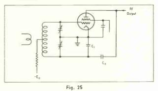
Push-pull grid neutralization, basic circuit.
