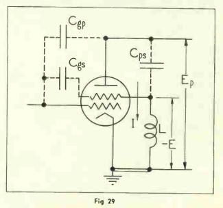
Tetrode characteristics involved in feedback circuit.
