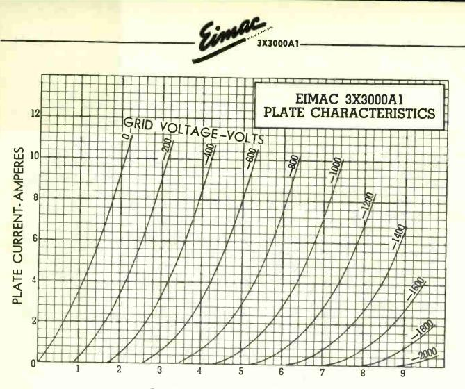
PLATE VOLTAGE - KILOVOLTS
