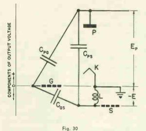
Graphical presentation of components of output circuit voltages in tetrode when self neutralized.
