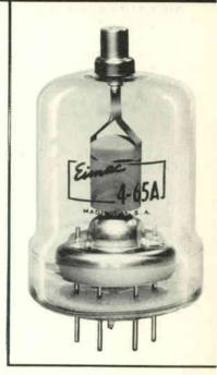
The Eimac 4-65A is a small radiation-cooled transmitting tetrode having a maximum plate dissipation rating of 65 watts. The plate operates at a red color at maximum dissipation. Short, heavy leads and low interelectrode capacitances contribute to stable efficient operation at high frequencies.
