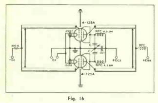
Screen-tuning neutralization circuit for use above 100 Mc. with 4-125A tetrode.
