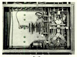
Fig 12 Underside of push-pull multi-band r-f amplifier employing 4-250A tetrodes. Designed and built by C. F. Bane (W6WB)<sup>3</sup>.
