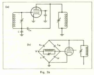
Single-ended grid neutralization described by Bruene<sup>6</sup>. a) Basic Circuit. b) Arranged as capacitance bridge.
