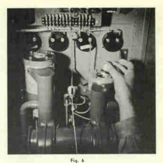
Experimental 950 Mc. doubler final and tripler driver employing 4X150A tetrodes. Designed and built by Eitel-McCullough Laboratories.
