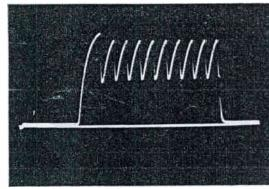
Figure 3-16. Veltage from oscillating neon bulb, applied through d-c amplifier channel. D-C voltages may be measured directly (base line represents zero volts)
