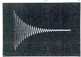
Figure 3-19. Waveform similar to that of Fig. 3-18. Increased accelerating potential of Type 304-H (3000 volts) rendered entire pattern visible
