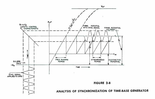
tial E<sub>x</sub>. At this point conduction ceases, and the plate potential rises slowly as the capacitor begins to charge through R55 and R57. The plate potential will again reach a point of conduction and the circuit will start a new cycle. The rapidity of the plate-voltage rise is dependent upon the circuit constants R55, R57, and the sweep-range capacitor selected, C18-C22, as well as the supply voltage E<sub>b</sub>. The exact relationship is given by:
