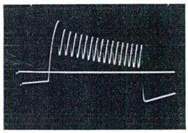
Figure 3-17. Waveform similar to that of Fig. 3-16, passed through a-c amplifier. Note tilt due to time constant of coupling circuit, and shift of reference axis
