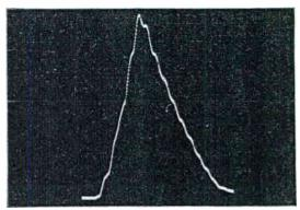
Figure 3-15. Indication of variation of volume of liquid in  $\alpha$  retort. Signal, applied through d-c amplifier channel, was displayed on a 10-second sweep
