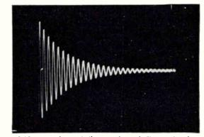
Figure 3-19. Waveform similar to that of Fig. 3-18. Increased acceleroting potential of Type 304-H (3000 volts) rendered entire pattern visible
