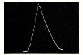
Figure 3-15. Indication of variation of volume of liquid in a retort. Signal, applied through d-c amplifier channel, was displayed on a 10-second sweep
