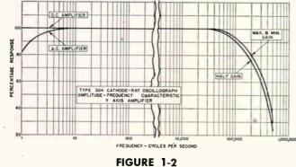
FREQUENCY-RESPONSE CURVE OF Y-AXIS AMPLIFIER
