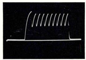
Figure 3-16. Voltage from oscillating neon bulb, applied through d-c amplifier channel. D-C voltages may be measured directly (bose line represents zero volts)
