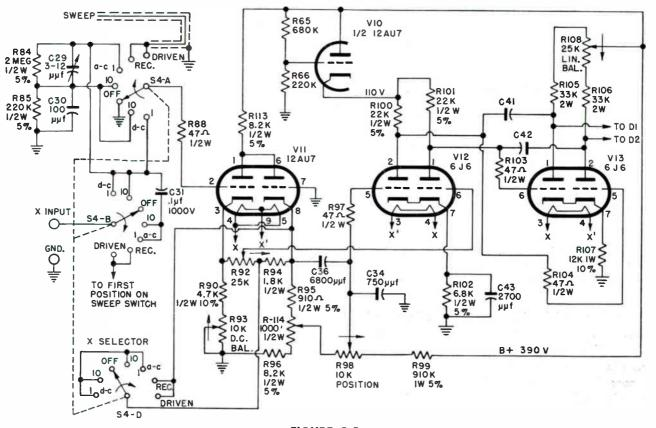
FIGURE 2-5 X-AMPLIFIER SCHEMATIC
