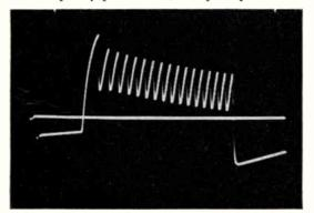
Figure 3-17. Waveform similar to that of Fig. 3-16, passed through a-c amplifier. Note tilt due to time constant of coupling circuit, and shift of reference oxis
