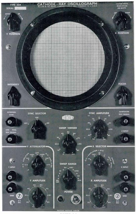
FIGURE 3-1 FRONT PANEL VIEW OF TYPE 304 AND 304-H CATHODE-RAY OSCILLOGRAPH For the operator who is well acquainted with cathoderay oscillographs, this table will probably furnish sufficient instructions to operate the instrument. For the new operator, however, the following discussion lists a step-by-step procedure for the efficient operation of the instrument. It is suggested that the new operator follow this procedure for learning the use of each of the operating controls.
