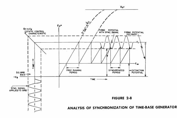
tial  $E_x$ . At this point conduction ceases, and the plate potential rises slowly as the capacitor begins to charge through R55 and R57. The plate potential will again reach a point of conduction and the circuit will start a new cycle. The rapidity of the plate-voltage rise is dependent upon the circuit constants R55, R57, and the sweep-range capacitor selected, C18-C22, as well as the supply voltage  $E_b$ . The exact relationship is given by:
