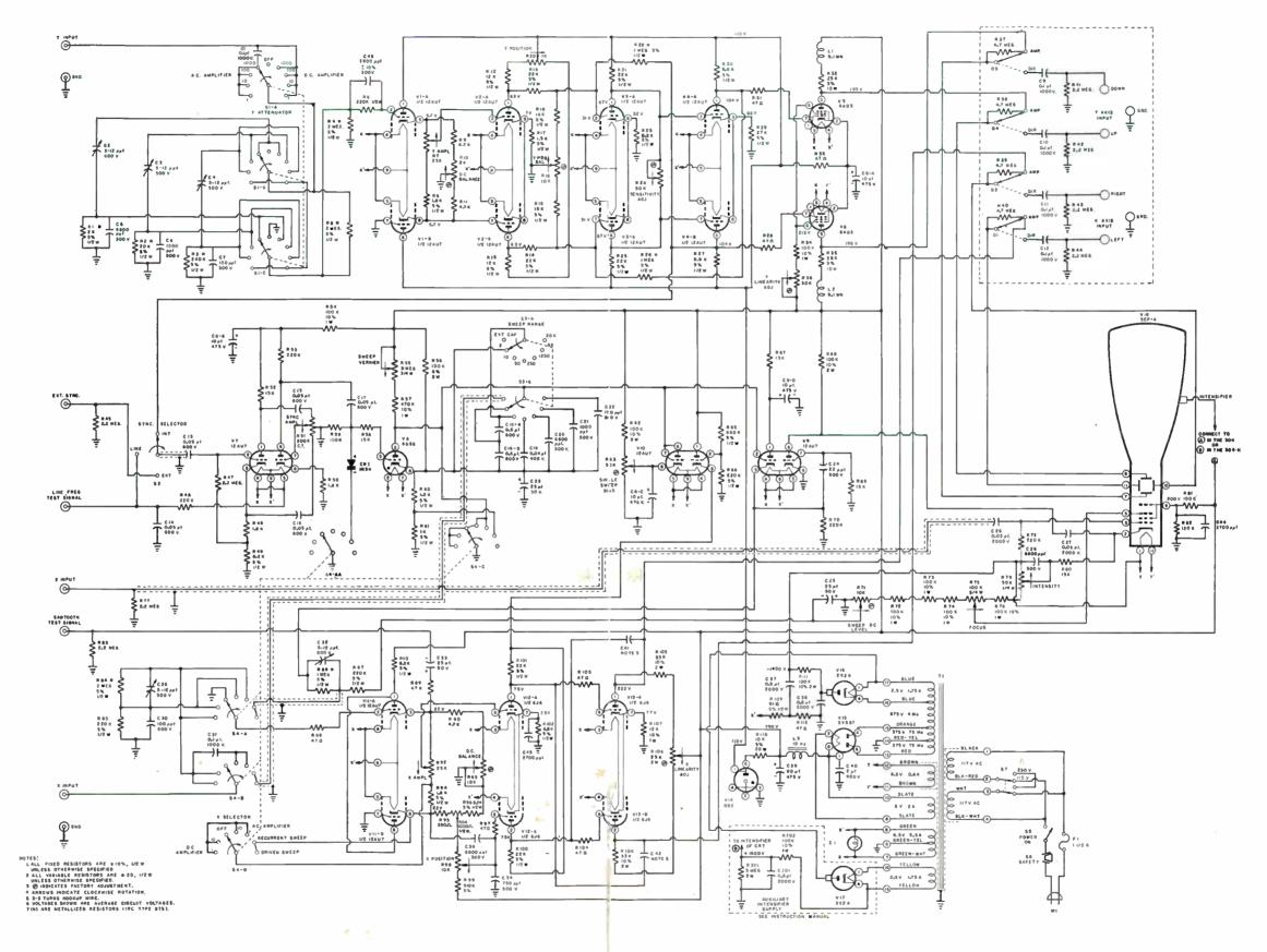
SCHEMATIC OF CIRCUIT OF THE DU MONT TYPES 304 AND 304-H CATHODE-RAY OSCILLOGRAPHS Ref. Dwg. 98000111-4 Issue 7
