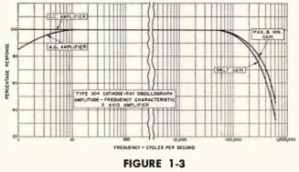
FREQUENCY-RESPONSE CURVE OF X-AXIS AMPLIFIER
