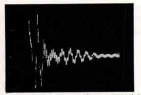
Figure 3-40. Kandom vibration in metal beam, recorded with Type 304 operating on single sweep. Note that entire phenomenon was recorded on the trace
