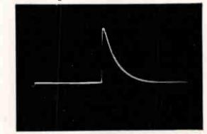
Figure 3-24. Observation of nerve potentials is an application requiring many features of the Types 304 and 304-H. Nerve potential below was recorded from Type 304
