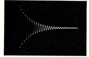
Figure 3-18. Relatively-high-speed transient in form of damped oscillation. With accelerating potential of 1780 volts, high-speed portion of trace was not recorded
