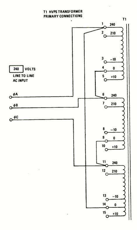
Figure 2-6. High-Voltage Power Supply Transformer Taps, 240-Volt Input.
