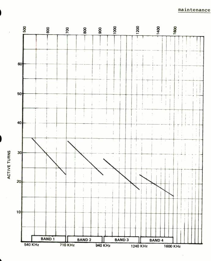
Figure 5-13. 315R-1 Node 2 Coil A9L2.
