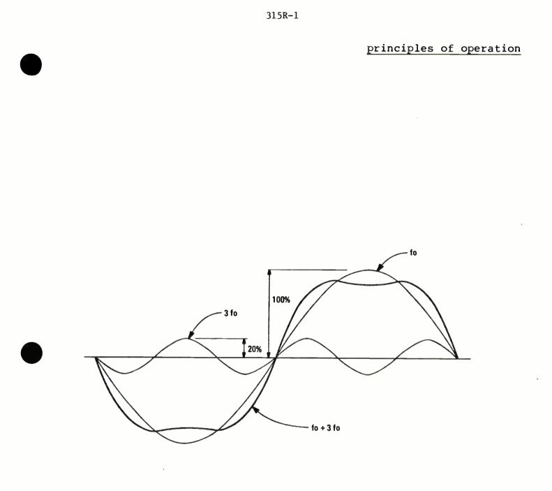
Figure 4-4. High-Efficiency Waveform.
