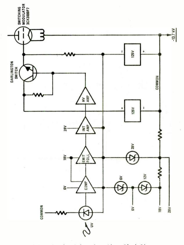
Figure 4-9. Switching Driver Operation, Block Diagram.
