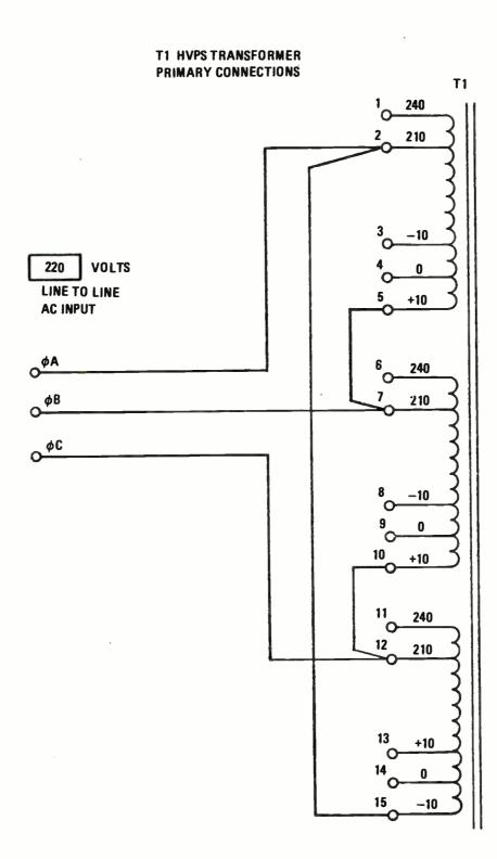
Figure 2-4. High-Voltage Power Supply Transformer Taps, 220-Volt Input.
