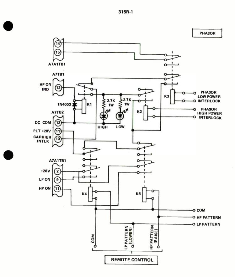
Figure 2-20. High/Low Power Switching Circuit
