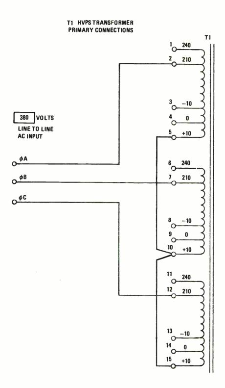
Figure 2-10. High-Voltage Power Supply Transformer Taps, 380-Volt Input.
