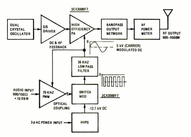
Figure 4-1. 315R-1 Simplified Block Diagram.
