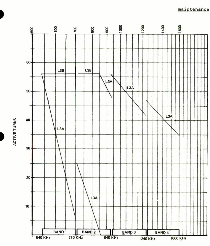
Figure 5-7. 315R-1 Node 2-3 Coupling Coil A9L3.
