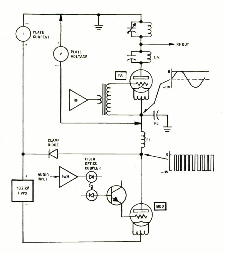
Figure 4-7. Transmitter Simplified Schematic.
