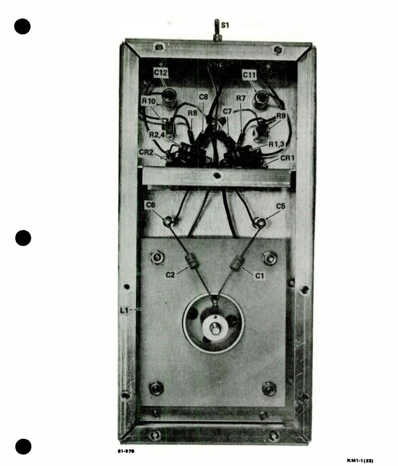
Figure 7-26. RF Power Meter (VSWR) A9A6 (Rear View)
