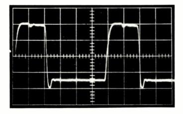
Figure 5-1. RF Exciter Output Waveform.
