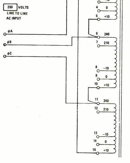
Figure 2-7. High-Voltage Power Supply Transformer Taps, 250-Volt Input.
