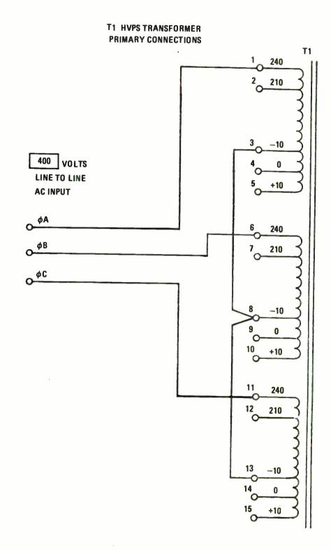
Figure 2-11. High-Voltage Power Supply Transformer Taps, 400-Volt Input.
