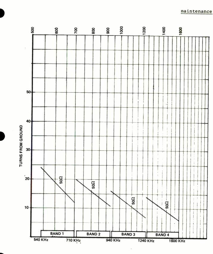
Figure 5-9. 315R-1 Output Tap (on A9L5).
