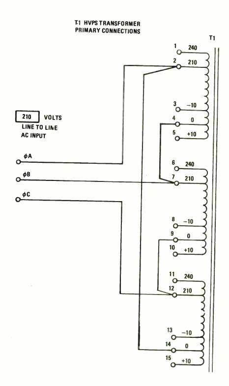
Figure 2-3. High-Voltage Power Supply Transformer Taps, 210-Volt Input.
