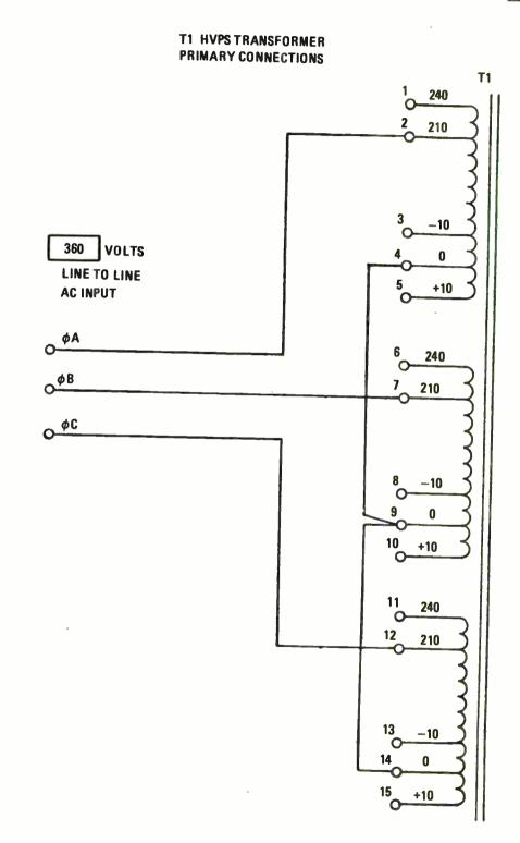
Figure 2-9. High-Voltage Power Supply Transformer Taps, 360-Volt Input.
