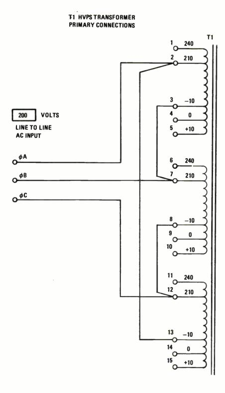
Figure 2-2. High-Voltage Power Supply Transformer Taps, 200-Volt Input.
