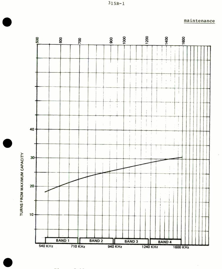
Figure 5-11. 315R-1 Tuning Capacitor A9C6.
