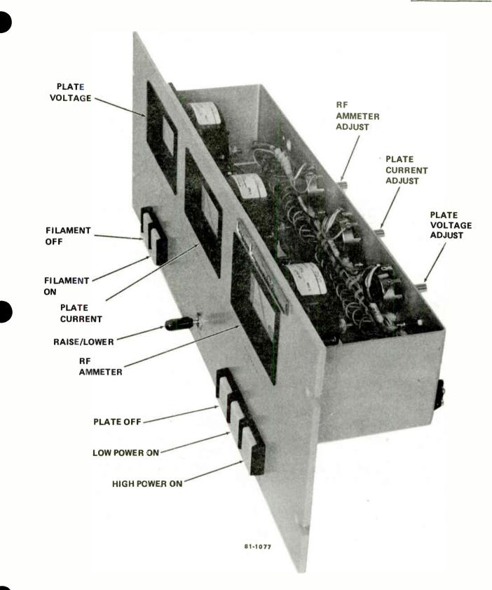
Figure 2-15. Extended Control Panel.
