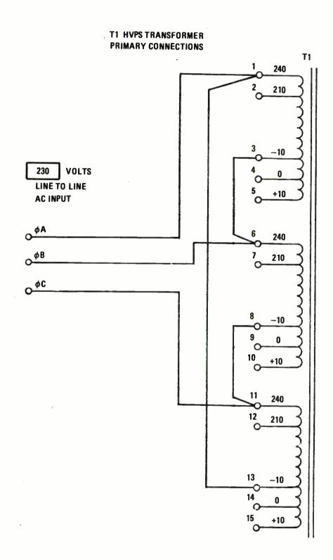
Figure 2-5. High-Voltage Power Supply Transformer Taps, 230-Volt Input.
