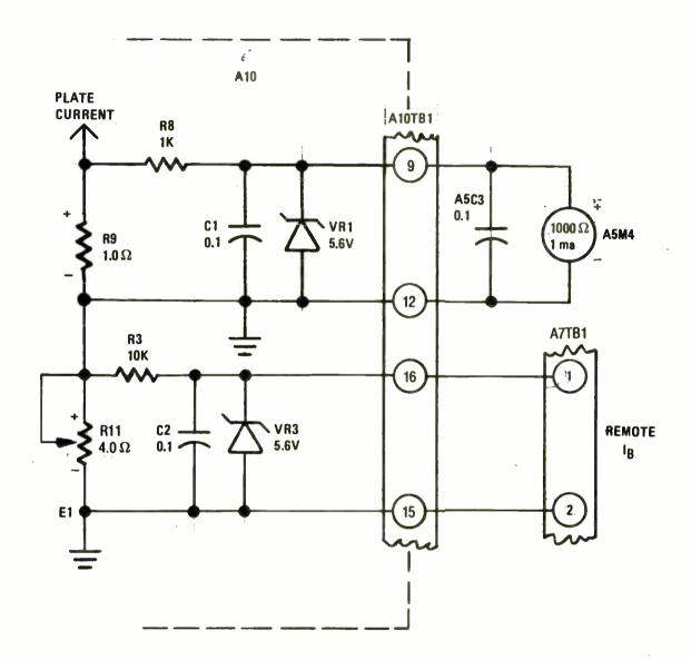
Figure 6-13. Plate Current Metering Circuits.
