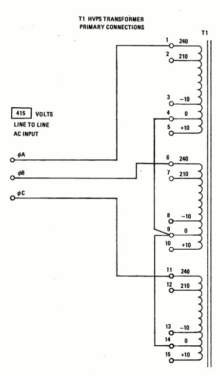
Figure 2-12. High-Voltage Power Supply Transformer Taps, 415-Volt Input.
