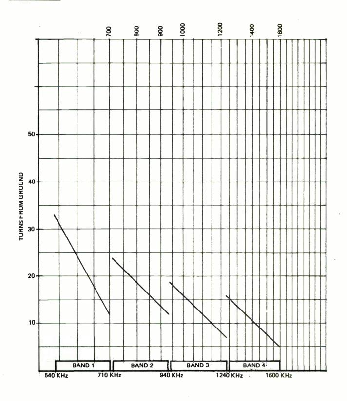
Figure 5-8. 315R-1 Node 3-4 Coupling Tap (on A9L5).
