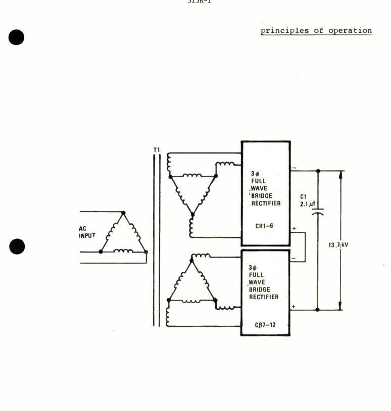
Figure 4-11. High-Voltage Power Supply Circuit.
