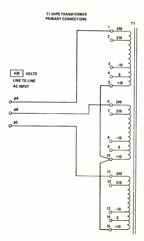
Figure 2-13. High-Voltage Power Supply Transformer Taps, 435-Volt Input.
