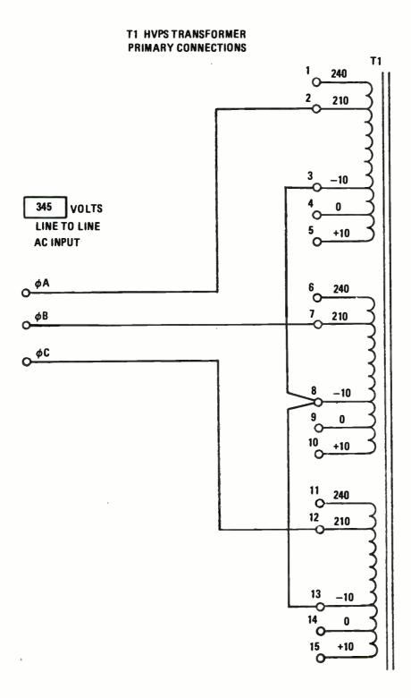
Figure 2-8. High-Voltage Power Supply Transformer Taps, 345-Volt Input.
