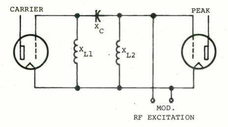
FIGURE 1.5 A SUITABLE CIRCUIT FOR ACCOMPLISHING THIS PHASE ADVANCE
