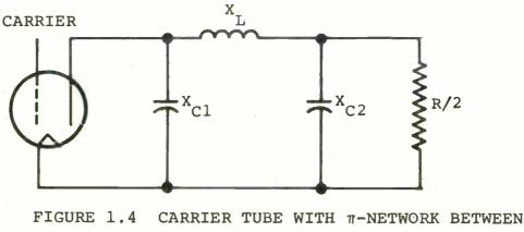
TUBE AND LOAD RESISTOR
