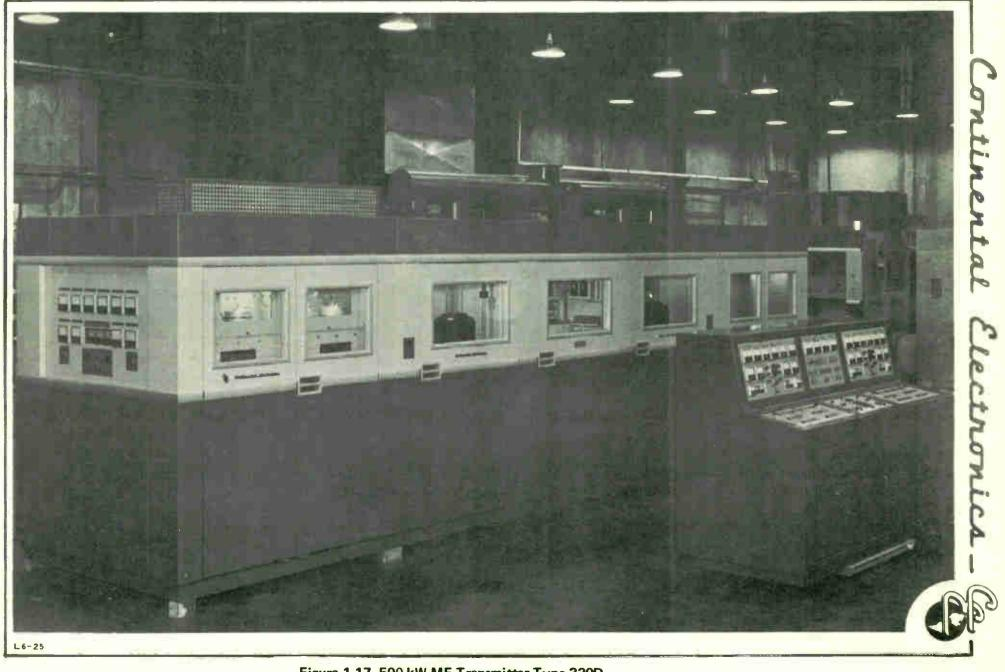
Figure 1.17 500 kW MF Transmitter Type 320D
