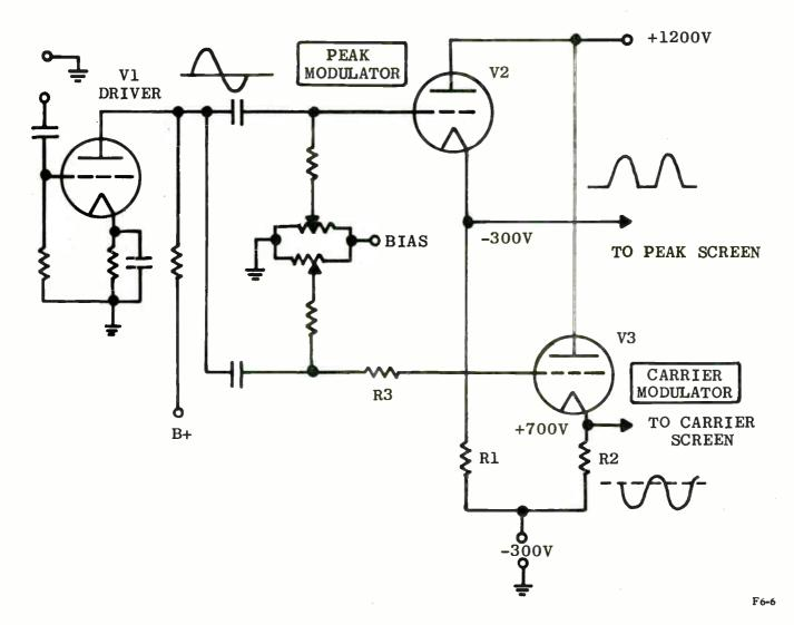
FIGURE 1.11. SIMULATING CLASS B PUSH PULL MODULATOR
