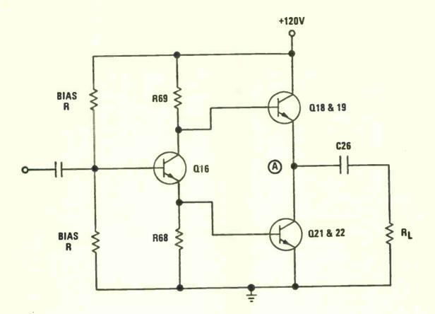
Figure 4-2. Modulator and 2nd Amplifier, Simplified Schematic
