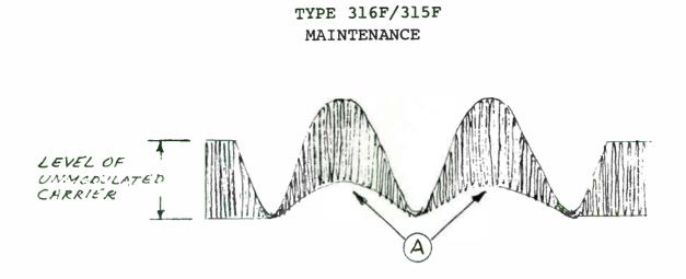
At point (A) in the modulation cycle, the transistors have insufficient base drive to maintain saturation at the time the DC collector voltage doubles its un-modulated value (100% modulation).
