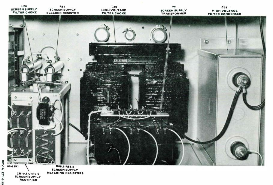
Figure 5-15. High Voltage Plate & Screen Supply Components, Viewed from Rear
