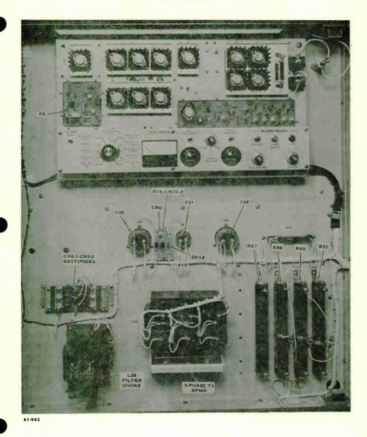
Figure 5-6. +120 Volt Power Supply, Showing Component Locations, Front View
