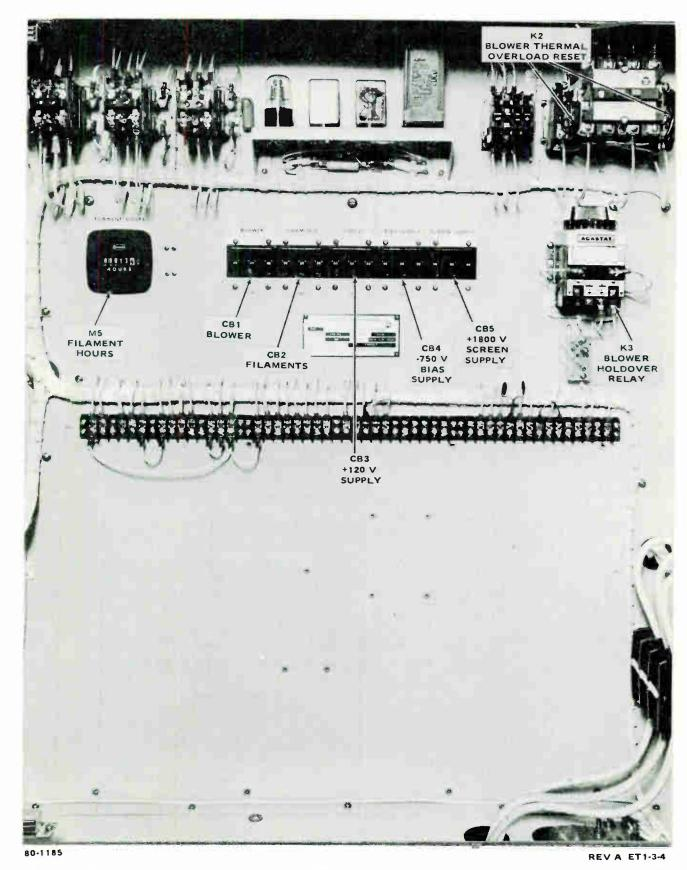
Figure 3-4. Control Section, Showing Circuit Breakers, Front View
