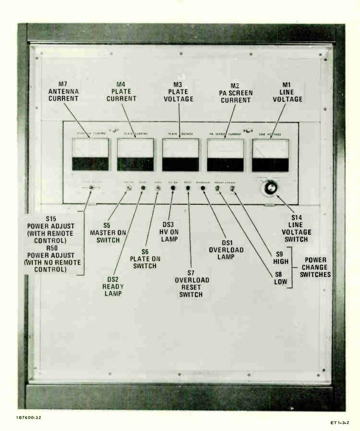
Figure 3-2. Operating Controls and Metering Panel, Front View
