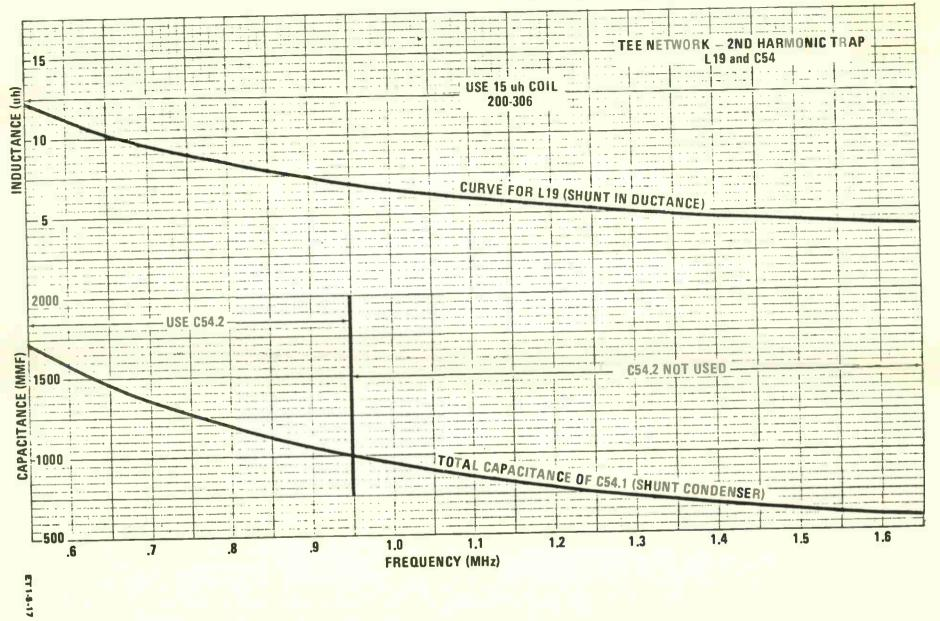
Figure 5-17. Tee Network - 2nd Harmonic Trap (L19 and C54) - Alignment Chart
