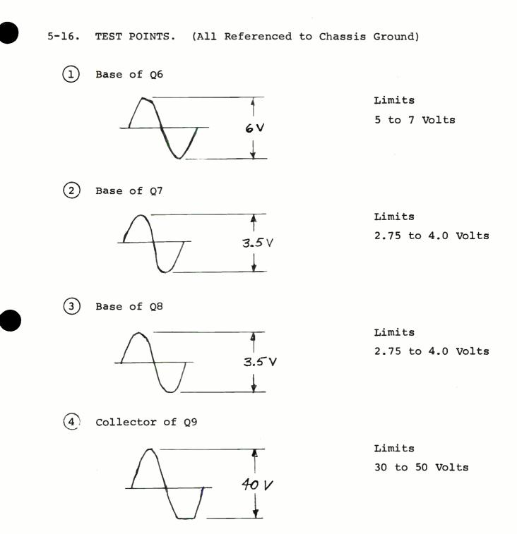
NOTE: If collector voltage swing is less than 30 volts peak to peak, decrease the value of emitter resistor R28 to 5 ohms (Two 10 ohm, 1/2 watt in parallel).
