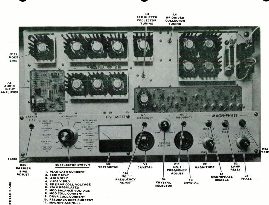
Figure 3-3. Solid State Exciter & Magniphase Control/Indicators, Front View
