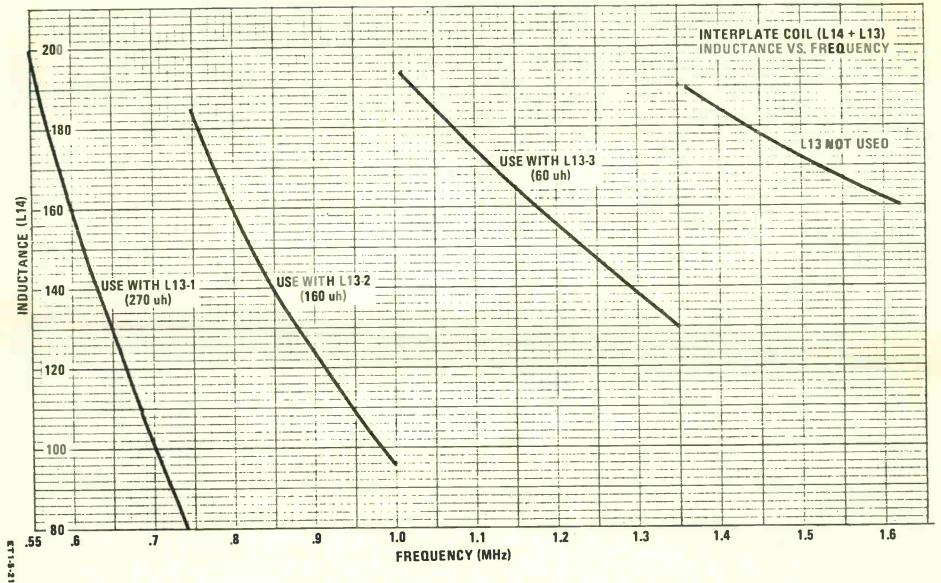
Figure 5-21. Interplate Coil (L14 and L13) - Alignment Chart
