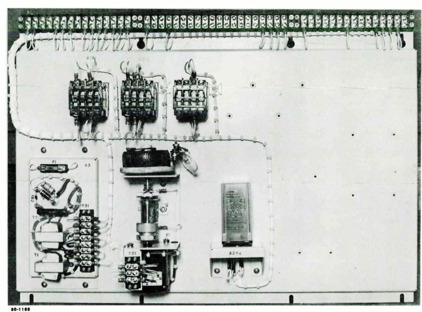
Figure 5-7.1 Remote Control & Power Reduction Components - Optional Equipment.
