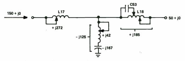
Typical reading for 50 ohm load.
