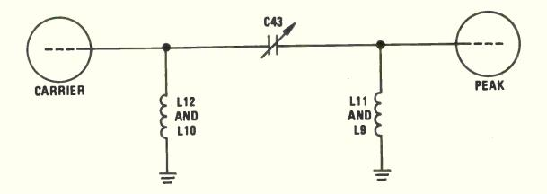
This is the basic 90° network. If capacitance is placed in parallel with the inductances, the network becomes:
