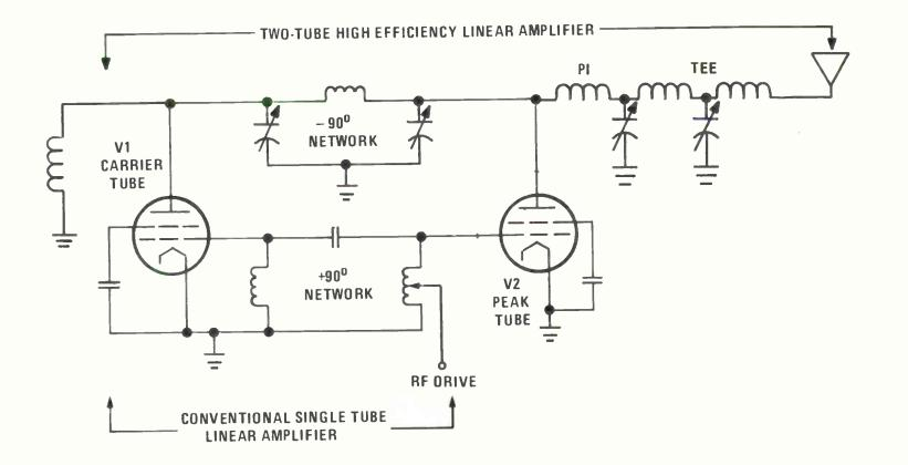
Figure 4-3. High-Efficiency Linear Power Amplifier, Type 316F/315F Transmitter, Simplified Diagram
