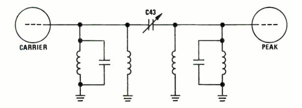
Since the shunt grid inductances on each side of C43.1 are parallel, they can become one coil equal to the parallel combination of the two. Adding the terminating resistance opposite the driven end of the network and tapping in the drive on the peak tank coil, the circuit now becomes:
