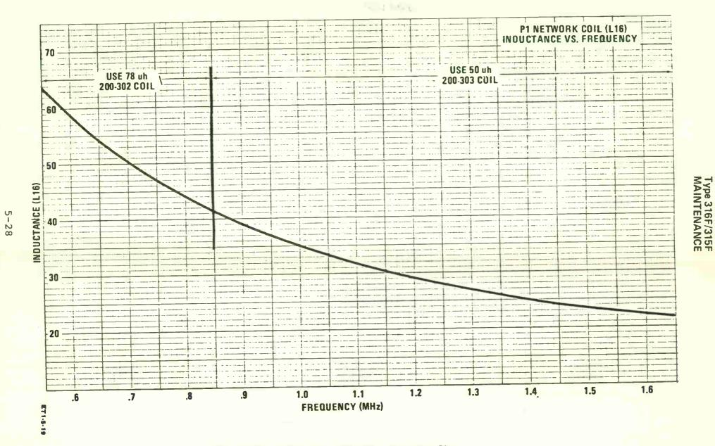
Figure 5-19. Pi Network Coil (L16) - Alignment Chart
