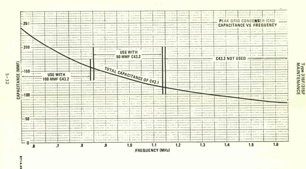
Figure 5-23. Peak Grid Condenser (C43) - Alignment Chart
