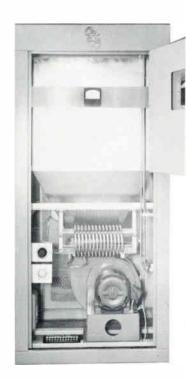
TYPE 517C 50 kw air cooled phantom antenna is forced-air cooled and completely self-contained. It will handle a 50 kw transmitter at 100% modulation, and is supplied as an essentially flat load of sufficient band width for modulation on the specified frequency and impedance in the standard broadcast band. The 517C is supplied
