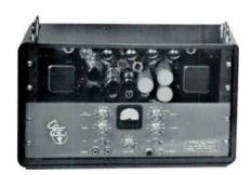
Freq. stability: better than .02% @ 7,000 mc .05% @ 12,000 mc SPECIFICATIONS, MVT/MVR RECEIVER
