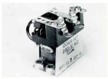
DOSX-7T: 115 vac coil, DPDT 15 amp, 115 vac non-inductive contacts. DOSX-12T: same as DOSX-7, except with 230 vac coil. DOSX-59T: same as DOSX-7, but has 110 vdc coil.
