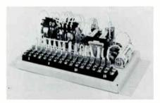
TYPE 31126-B, PROGRAM LINE REVERSING UNIT. Changes transmitter inputs between main and spare program lines. Battery provides studio metering indication according to position of lines.
