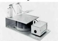
TYPE B31099-1, ANTENNA METERING UNIT. Produces rectified dc sample proportional to R.F. current. ac power not required. For currents of 0 to 15 amperes RF Type B31099-2 used for currents of 15 amps and above.
