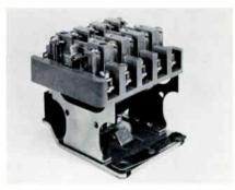
RBM CONTACTORS. Heavy-duty, industrial contactors, they may be connected at TRC-T switching output to control external pushbutton circuit, or for interlocking use in external circuitry. Recommended for Plate on - off control. RBM 101130-101: 115 vac coil, 3 PNO reversible contacts, rated 10 amps, 115 v ac non-inductive. RBM 101150-101: same as RMB 101130-101 but has 5PNO reversible contacts. RBM Contactors also available with 230 vac coils, and with 15 amp reversible and 25 amp N.O. contacts.
