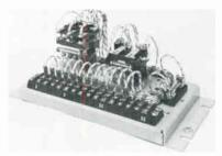
TYPE 31122-B, ELECTRICAL LATCHING RELAY UNIT. Similar to Type 31121-B, except unit is held in "on" position through its own contacts, will automatically release if transmitter site power fails momentarily. DPDT contacts rated 10a, 115 vac, non-inductive.
