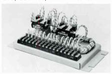
TYPE 31123-B, MOMENTARY OUTPUT RELAY UNIT. Connects between TRC-T unit and transmitter for control of circuits locally controlled by push-buttons, such as pattern change, and existing motors. Two sets DPDT contracts rated 15a, 115 vac, non-inductive.
