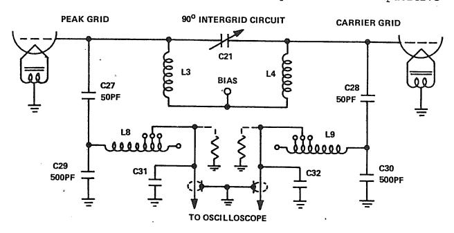
Figure 4.16 Simplified Schematic of PA Grid Circuit
