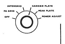
Proper 90° phasing of the power amplifier plate circuit is indicated by the vertically oriented ellipse on the oscilloscope when the tuning selector switch is in either the PEAK PLATE or POWER ADJUST positions. With the selector switch in the PEAK PLATE position, the ellipse will lean either left or right when the TUNE switch is operated and will change much slower than was noticed with grid circuit tuning. Proper tuning is with the ellipse upright.
