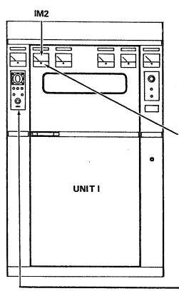
With the tuning selector switch in the CARRIER PLATE position tune for a closed diagonal line concurrent with a dip in TOTAL PLATE CURRENT as indicated on 1M2. If the dip doesn't exactly correspond with the closing of the line, tune for the closed line which indicates the 1800 phase comparison of carrier tube RF grid and plate voltage.
