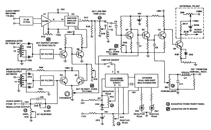
Figure 4.13 Simplified Schematic of Audio Amplifier
