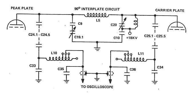
Figure 4.17 Simplified Schematic of PA Plate Circuit
