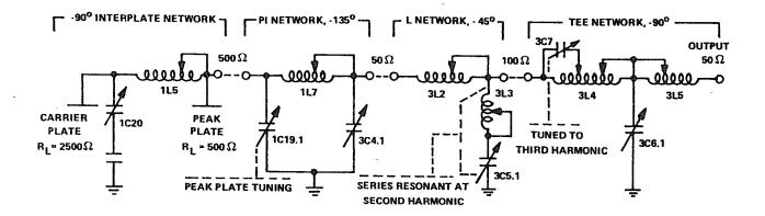
Figure 4.3 Simplified Schematic of Output Network
