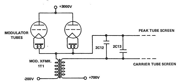
The modulation transformer (1T1) voltage ratio (turns ratio) is 1:1 and the primary and secondary turns are laid adjacent to one another (bifilar) over the full multilayer winding. The leakage inductance of this type of winding is the lowest possible and also, since the primary and secondary voltages are equal, the voltage stress between windings reduces to simply the DC voltage difference
