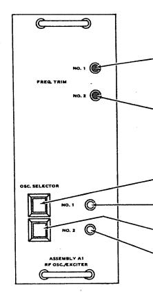
Use insulated tuning tool (screw driver blade) to set carrier frequency when No. 1 oscillator LED is lighted.
