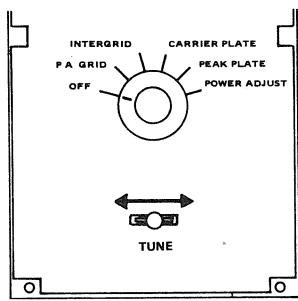
OFF Oscilloscope and tuning motor power off.
