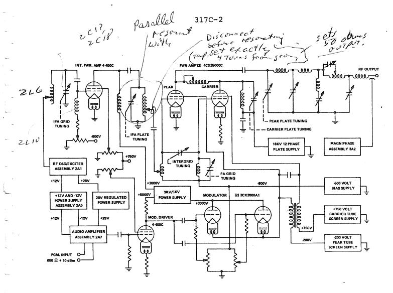
Figure 4.2 Simplified Schematic Diagram
