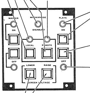
PLATE ON LED lights green when the PLATE ON switch (green button) is pushed. The 3 phase vacuum contactor (4K1) closes and RF excitation is applied 100 milliseconds later.
