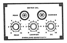
In series with each relay coil/resistor is a 50 ohm rheostat. These are the front panel sensitivity controls. At maximum sensitivity (fully clockwise or 10 on the dial scales) the rheostat is at zero resistance so that the relays will operate at 4 VDC. At minimum sensitivity (fully counter-
