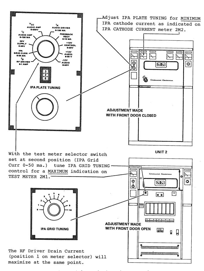
Figure 4-8. Unit 2 Tuning Controls
