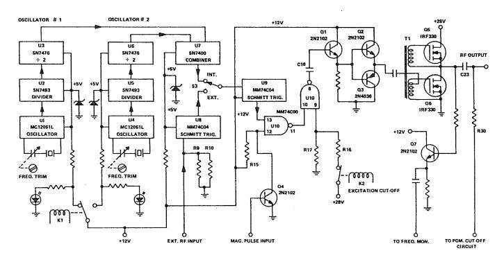
Figure 4.12 Simplified Schematic of Oscillator/Exciter Assembly
