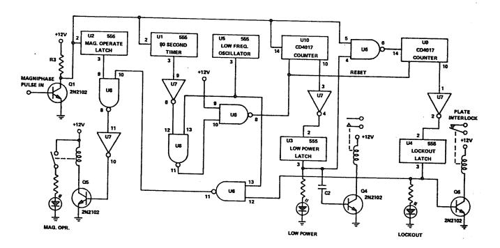
Figure 4.15 Simplified Schematic of Magniphase Control (2A6)
