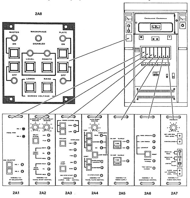
Subassemblies 2Al through 2A7 are plug-in modules. Before unplugging or re-installing remove all DC power from solid-state circuits by manually turning off circuit breakers 2CBl and 2CB2 located just below subassembly 2Al.
