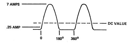
The average or DC value of the waveform will be  $7/\pi = 2.23$  amps. The grid current of .15 amps and about .2 amps screen current will raise the DC cathode current of the Peak tube to about 2.6 amps at 100% modulation.
