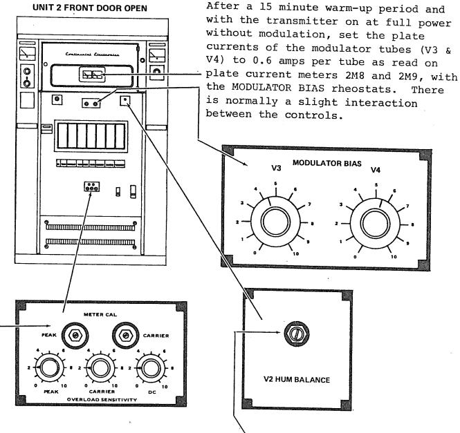
The peak and carrier METER CALI-BRATE controls (two upper controls with shaft locks) are factory set with a 1% DC ammeter to provide accurate indication of the peak and carrier tube cathode currents as indicated on the unit 1 TEST METER (1M6). The three OVERLOAD SENSITIVITY controls are normally set at 2 which will accommodate very high average program modulation.
