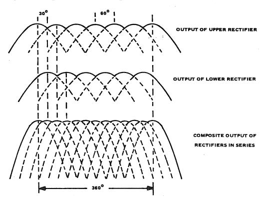
The DC level is 9 + 9 = 18 kV. There are 12 ripple peaks per cycle (hence the term 12 phase) so the ripple frequency is now 12 x 60 = 720 cycles and the ripple level is reduced from 4% to 1% (-40 dB) which precludes any necessity for a filter reactor.
