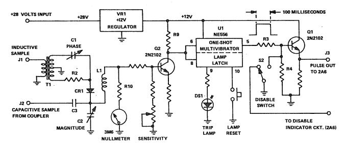
Figure 4-14. Magniphase Simplified Schematic, Unit 3A2
