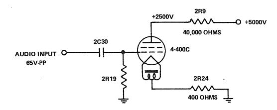
satisfy this requirement is, 2500V/40,000  $\Omega$  = .0625 amps. The plate current excursions necessary to swing  $\frac{+}{2}$  1875 volts (3750 volts P-P) will be, 1875V/40,000  $\Omega$  = .047 amps.
