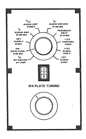
I<sub>d</sub> RF DRIVER 0-1 amp. This is the drain current of the output MOSFETs in the 2Al OSC/Exciter assembly. Typical reading is .4 to .6 amp.
