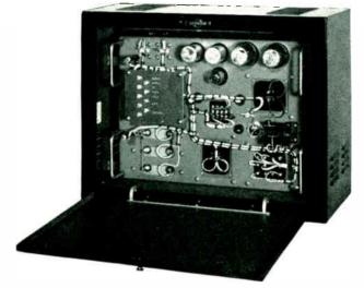
A wall mounting Power Supply for the 212A console, it contains three supplies which furnish d-c power for preamplifiers, monitor and line amplifiers, and 12 volts for relay operation. In addition, it furnishes 6.3 volts a-c to operate all tubes in the console.
