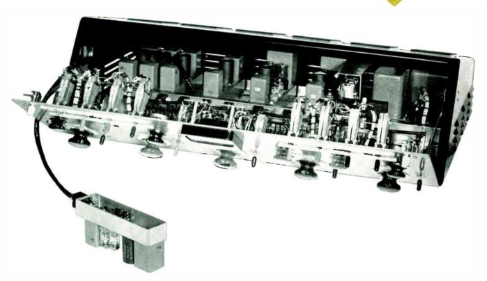
plug-in type of construction allows easy removal or relocation of the units.
