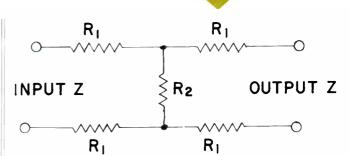
Input and Output Z = 600 Ohms
