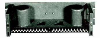
The 117N-2 Repeat Coil Panel is a complete assembly including chassis, terminal board and dust cover, but less repeat coils. This unit will accommodate four Thordarson type repeat coils with an R-4 case. There are 50 terminals on the board for making connections to external equipment. The dust cover is held on by two convenient Dzus fasteners.
