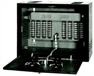
This Relay Control Unit, used with the 212A console, completely controls studio and control room loudspeakers, as well as studio on-off-the-air lights. Two switches on the hinged front panel control power to the power supply and studio warning lights.
