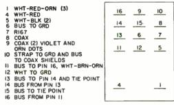
Figure 7-2. KWM-2 and KWM-2A, Location of Chassis Mounted Components, Bottom View
