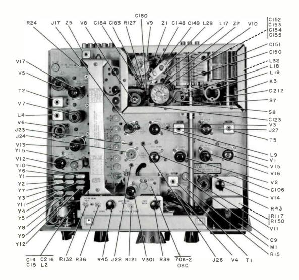
Figure 6-1. Top View, Parts Identification
