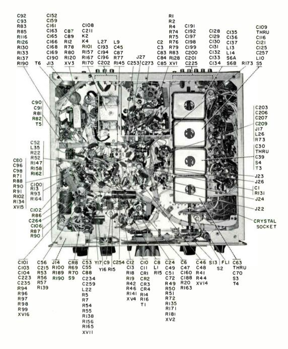
Figure 6-4. Bottom View, Parts Identification
