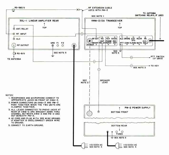
Figure 1-2. Traveling Station Interconnections with 30L-1
