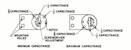
Figure 4-2. Ceramic Trimmer Capacitors
