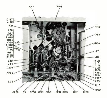
Figure 6-3. PA Grid Compartment, Bottom View, Parts Location
