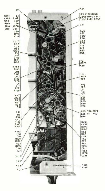
Figure 6-2. Bottom Right View, Parts Identification
