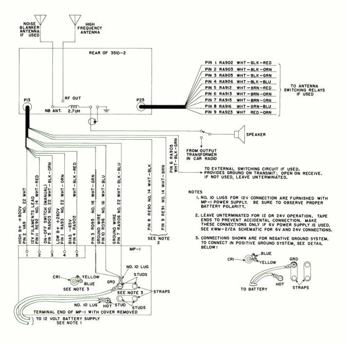
Figure 1-4. Mobile Station Interconnections
