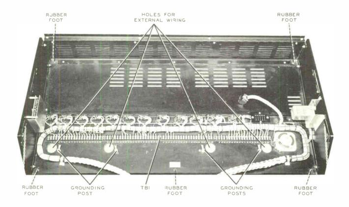
Figure 2-1. Broadcast Console 212G-1, Mounting and Wiring Detail
