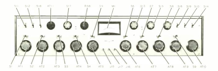
Figure 3-1. Broadcast Console 212G-1, Control Locations
