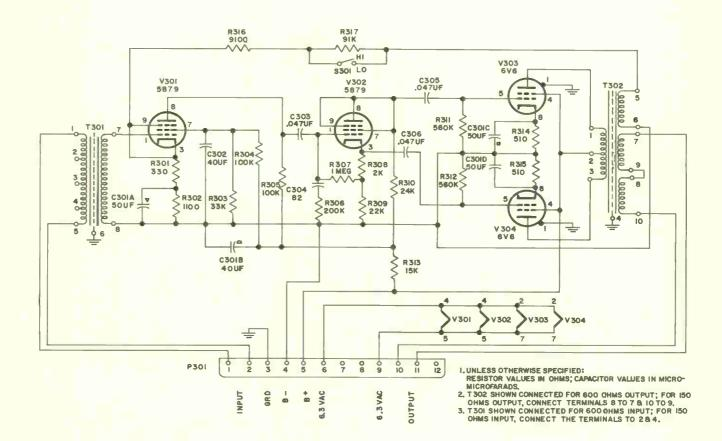
Figure 4. 356B-1 Program/Monitor Amplifier, Schematic Diagram
