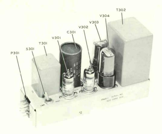
Figure 2. 356B-1 Program/Monitor Amplifier, Top View
