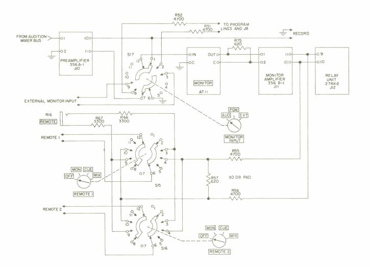
Figure 4-4. Monitor Circuits, Simplified Schematic Diagram
