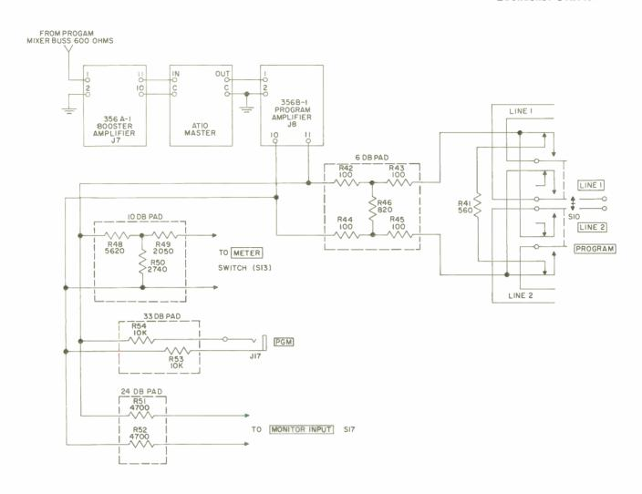
Figure 4-3. Program Circuits, Simplified Schematic Diagram
