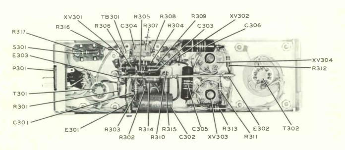
Figure 3. 356B-1 Program/Monitor Amplifier, Bottom View
