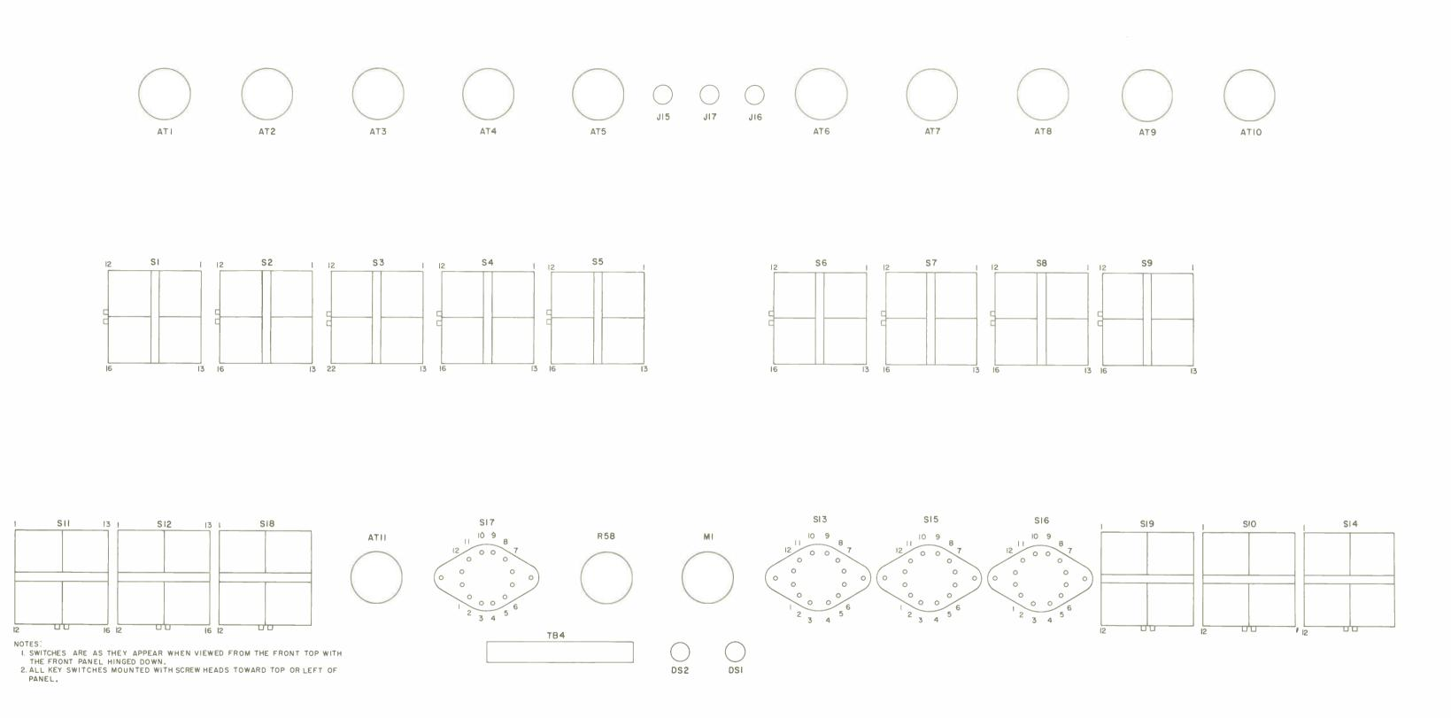
Figure 7-2. Broadcast Console 212G-1 Switch Pin Orientation
