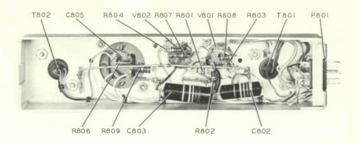
Figure 2. Cue Amplifier 356Q-1, Bottom View
