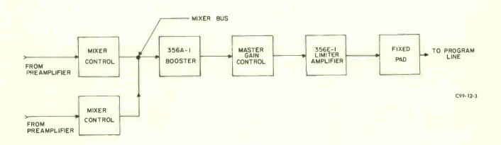
Figure 4. Collins Type 356E-1 Limiter Amplifier as Automatic Mixer, Suggested Arrangement
