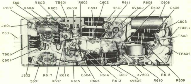
Figure 10. 356E-1 Limiter Amplifier, Bottom View
