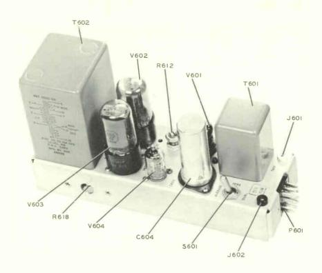
Figure 9. 356E-1 Limiter Amplifier, Top View
