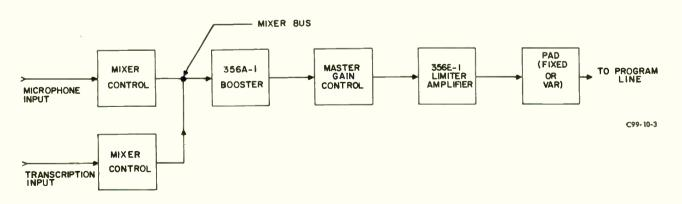
Figure 2. Collins Type 356E-1 Limiter Amplifier as Automatic Fader Control,
