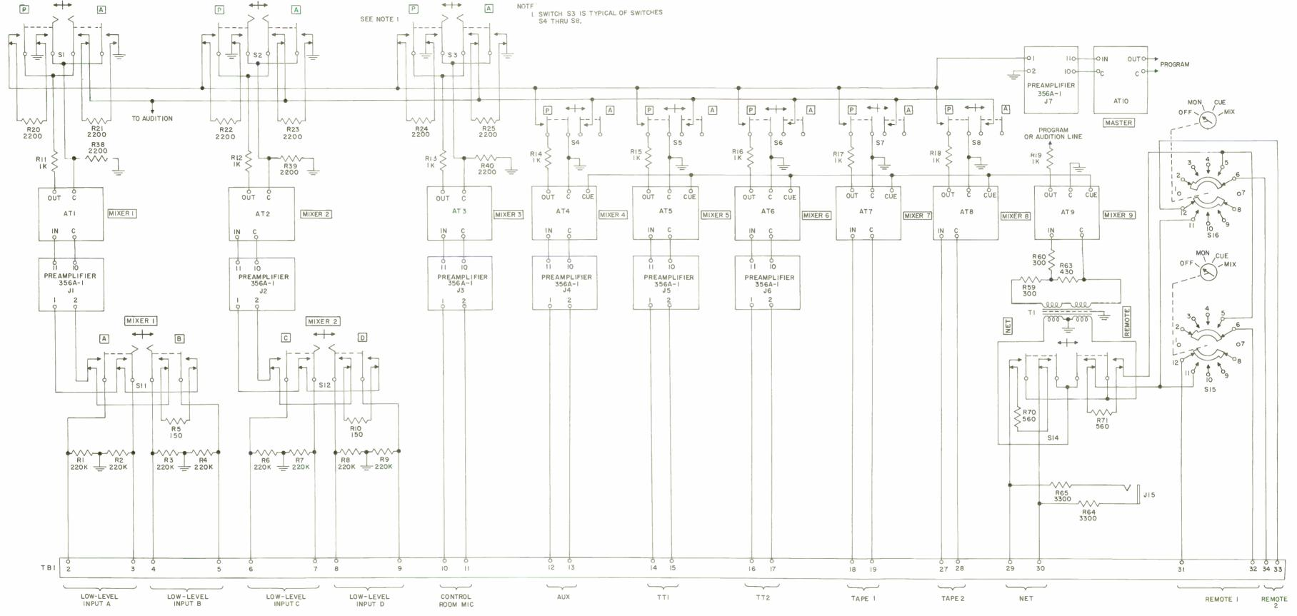
Figure 4-2. Mixer Circuits, Simplified Schematic Diagram
