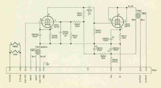
Figure 3. Cue Amplifier 356Q-1, Schematic Diagram
