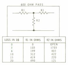
Figure 2-4. Resistor Values for Fixed Pads
