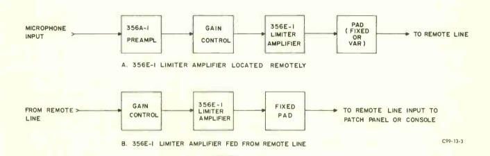
Figure 3. Collins Type 356E-1 Limiter Amplifier as Automatic Level Control,
