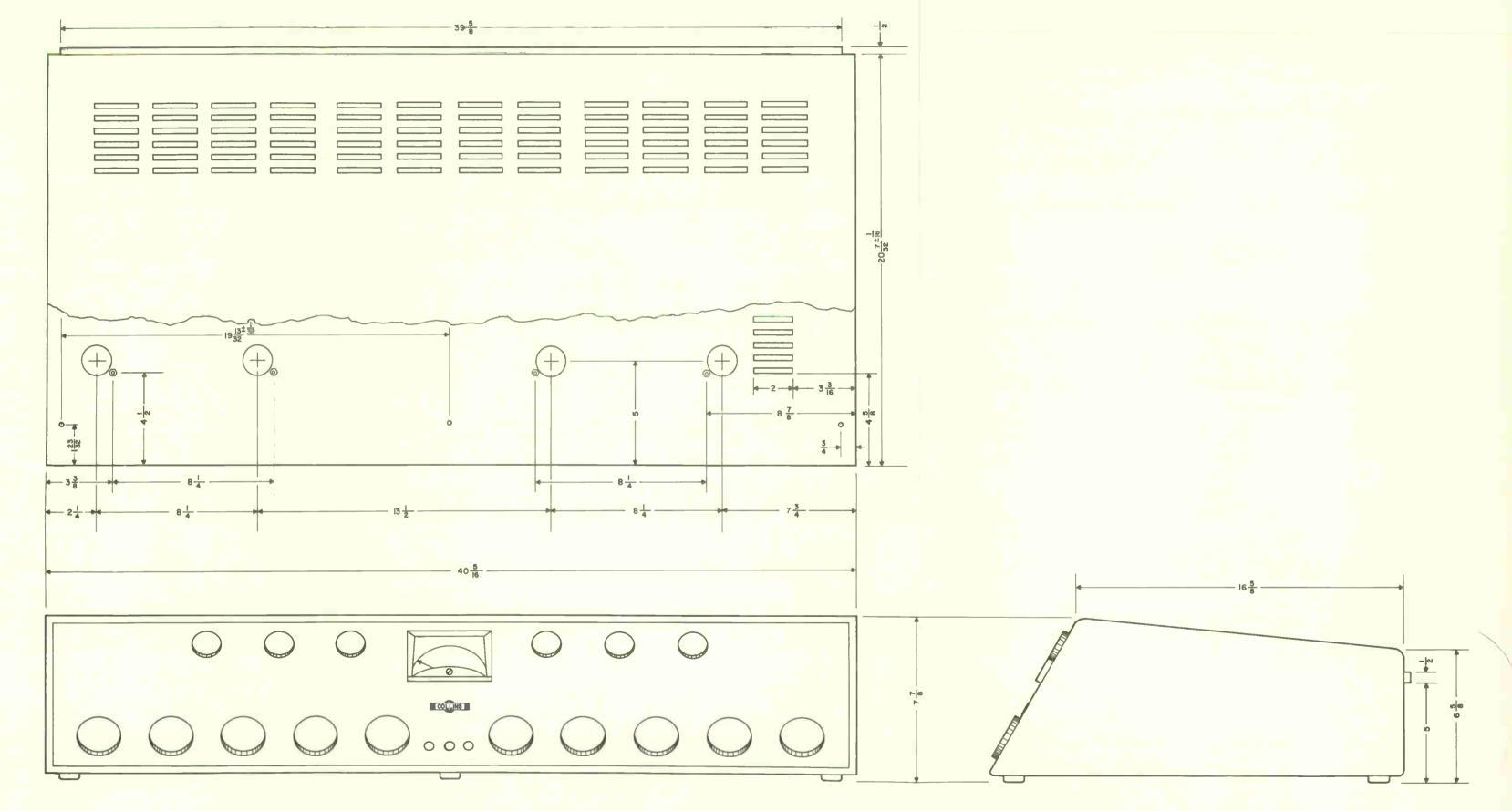
Figure 7-3. Broadcast Console 212G-1, Outline and Mounting Dimensions
