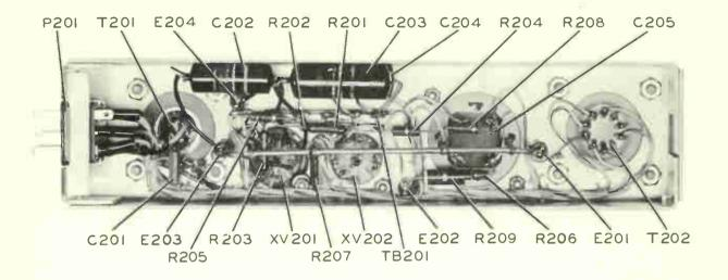
Figure 3. 356A-1 Preamplifier, Bottom View
