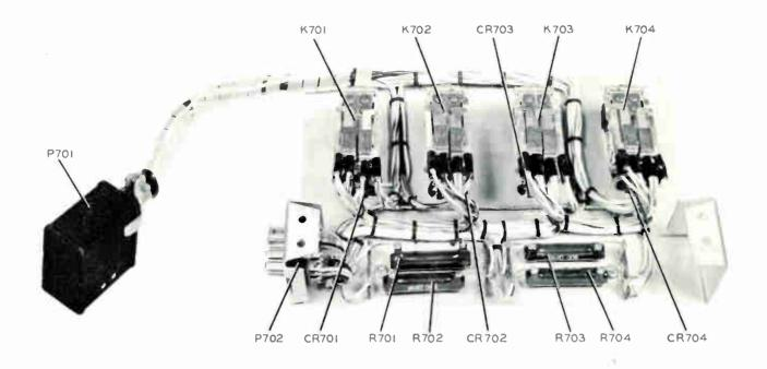
Figure 2. Relay Unit 274K-2, Cover Removed
