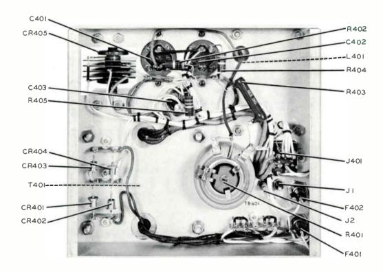
Figure 2. Power Supply 409X-2, Bottom View
