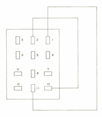
Figure 2-3. Jumper Plug Wiring Schematic Diagram
