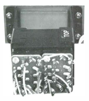
Figure 5-1. Readout Assembly, Rear View.
