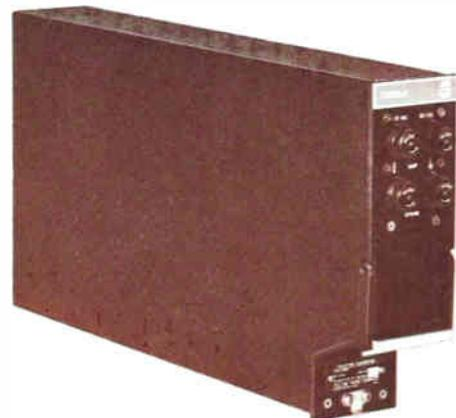
The 700B-2 consists of four plug-in modules on an aluminum chassis housed in a short 1/4 ATR case. All electrical connections are made through a single connector located at the rear. Test points on each module aid in performing maintenance checks. Reliability is greatly enhanced by the use of solid state components.
