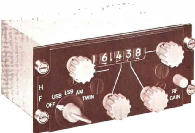
The 714Y-1 is a panel or console mounted control unit which permits selection of frequency, operating mode and RF gain level for a Collins Universal Radio Group receiver, exciter or exciter-receiver installation. Channel frequencies are indicated in a direct reading digital readout and can be selected in 1 kc increments throughout the 2.0-29.999 mc range. All frequency selection terminations are diode isolated to permit paralleling of control units.
