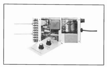
An economical unit to equalize and amplify the output signal of a magnetic phono cartridge, this small transistorized unit is used to replace passive equalizers and console or turntable preamplifiers. The housing of the unit is constructed of steel for magnetic shielding.
