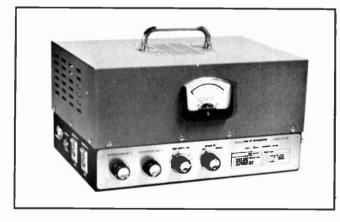
The M-30B/TPS is a 30 watt base station transmitter for communication with mobile units operating in the 152 to 172 megacycle range. The unit provides frequency stability of  $\pm$  .0005% within a temperature range of minus 30 degrees C to plus 60 degrees C. The modulation characteristic is adjusted at the factory for  $\pm$  7.5 kc for 100% modulation at 1000 cycles.
