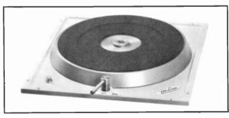
The TT-900 is a turntable designed specially for stereo operation and meets NAB specifications for stereo operation. The chassis is of heavy cast aluminum. A simple speed shift lever is located in the center of the chassis for choice of 2 speeds,  $33\frac{1}{3}$  and 45 rpm. In the off position the drive puck is removed from the rim to prevent flatting. An indentation in the platter eliminates the need for a spindle adapter for 7" 45 rpm records. *Motor:* Synchronous
