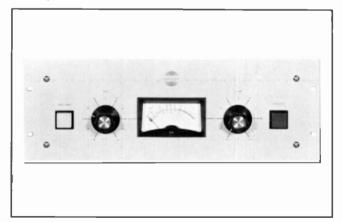
The 216C-2 Recording Amplifier is used with the 642A-2 Recorder/Playback Unit to provide facilities for recording pre-erased tape cartridges. This unit contains preamplifiers for 600-ohm line and 250-ohm microphone inputs, input lecel controls, and an output amplifier. The two inputs may be mixed if desired.
