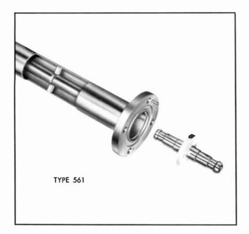
Type 561, Rigid Copper Transmission Line is supplied in standard 20 ft. sections with EIA flanges on both ends. All flanged sections include EIA inner connector, "O" ring gasket and hardware. Specify operating frequency when ordering lines.
