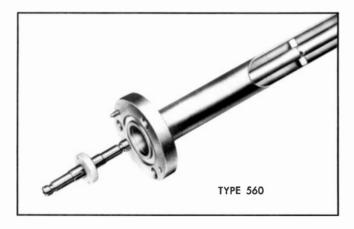
Type 560, Rigid Copper Coaxial Transmission Line is supplied in standard 20 ft. sections with EIA flanges on both ends. All flanged sections include EIA inner connector, "O" ring gasket and hardware. Specify operating frequency when ordering lines.
