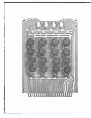
The 384D-1 is used in the 212S-1 and 212M-1 consoles to switch remote lines coming into the consoles.
