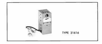
Type 31615 Humidity Sensor is designed to activate remote indicators on alarms at the presence of moisture in the output of dehydrators. The unit is factory installed in any of the 1920 series dehydrators and is set for specific values of humidity. The leads are brought to a terminal block installed in the dehydrator for the external connection.
