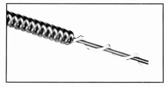
These small diameter air dielectric Heliax cables are ideal for use as sampling lines and in phased arrays where stability of electrical characteristics is important. For all uses, the copper inner and outer conductors assure optimum performance.
