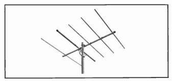
Nominal Impedance: 50 ohms. Average Gain: 9 db. Typical VSWR: Under 1.5. Typical Rear Signal Rejection: 25 db. Power Handling Capacity: 60 watts. Input Connector: Type AN-SO-239 (Amphenol Type 83-
