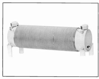
These solenoid wound 2. and 3-wire chokes provide high impedance throughout the broadcast band for isolation of the ac power lines from the antenna. Coils are wound of #10 wire and are rated at 2,000 watts, 120
