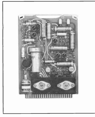
The 356P-1 is supplied for use in 212S-1 and 212M-1 consoles as program output amplifiers.
