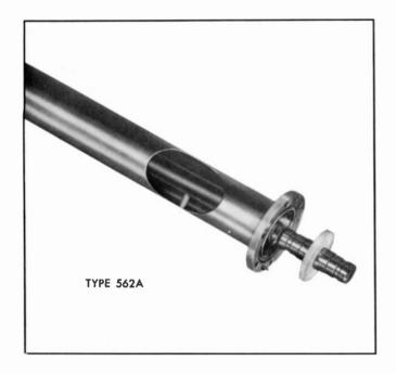
Type 562A Rigid Copper Transmission Line is supplied in standard 20 ft. sections with EIA flanges on both ends. All flanged sections include EIA inner connector, "O" ring gasket and hardware. Standard 19' 8" lengths are available for special frequency applications. Specify frequency or channel when ordering lines.
