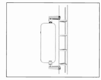
Designed to sample the relative phase relationship of radio frequency energy from 550-1600 kc antenna towers in directional antenna arrays, the Collins 56-1A-1 is made of two loops of #10 copper wire which may be connected either in series or in parallel. The wires are contained within a loop of  $\frac{7}{8}$ " painted, copper tubing which serves as an electrostatic shield.
