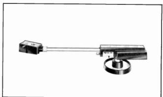
Accepts stereo and monophonic cartridges. Arm features precision ball bearings at all pivot points, plug-in head with positive alignment lock and variable adjustment. Supplied with arm rest, mounting template, mounting hardware and 4-foot cable assembly.
