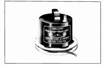
A compact and convenient bulk tape eraser that removes recorded signals from tape up to 35 mm in size and lowers background noise level up to 6 db below that of unused tape. A pushbutton safety switch prevents current from being applied when not in use.
