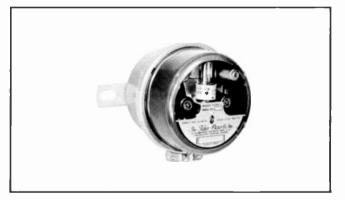
Designed to mount in a standard commercial meter socket. The 63305DB will automatically control broadcast tower lights directly or with auxiliary contactors. Adjustable potentiameter allows adjustment for operation from 0 to 50 f.c.
