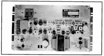
The MR-30/150-170 receiver is used for pickup from a mobile station operating in the 150 to 174 megacycle range. The receiver is sensitive to 0.6 micro-volts or less for 20 db quieting, and is selective to -100 db at  $\pm 32$ kc; -6 db or less at  $\pm 15$  kc.
