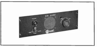
Designed to control visible and/or audible alarm circuits on EBS signal from local or sky wave stations. Frequently tunable from 550 to 1600 kc. Built-in speaker operates upon alarm. Relay circuit is voltage regulated. External bell or light control terminals and antenna terminals on rear terminal board. Available for rack mounting only.
