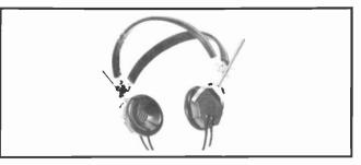
Ideal for general purpose service, the Brush BA-200 headphones have a frequency range from 100 to 5,000 cps. They are especially suitable for general laboratory and studio work as well as for the skilled amateur. Impedance: 45,000 ohms at 1,000 cps.
