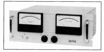
This all new solid-state unit offers basically improved indications of the phase relations in directional antenna systems. It also incorporates provisions for indicating the relative amplitudes of the currents in the various antennas. This Phase Monitor can be used with systems containing up to 9 towers.
