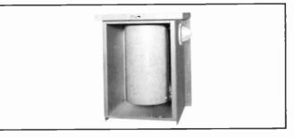
Coil provides isolation for the sampling line in directional arrays, presenting a high impedance for the line across the base insulator. Unit consists of a phenolic coil form which will accommodate 37 turns (approx. 100 ft.) of RG8/U or similar solid dielectric sampling line. May be mounted on wall of tuning shack or in housing similar to that pictured.
