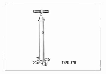
Type 878 Dry Aid Hand Pump pressurizes up to 1,000 ft. of 7/8'' cable and up to 250 ft. of 15/8'' line. Supplied with 1 lb. of silica gel and 8 feet of hose. Weight: Net 10.5 lbs., Gross 12 lbs.
