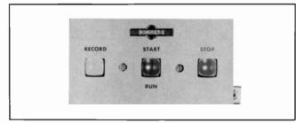
Has illuminated "start," "record" and "stop" buttons for control of one record/playback system from a remote point.
