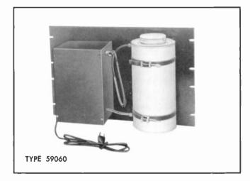
Type 59060, Low Pressure Dehydrator is ideal for pressurizing microwave waveguide systems or small air dielectric cables. This dehydrator maintains a constant pressure of dry air inside the waveguide or coaxial cable.
