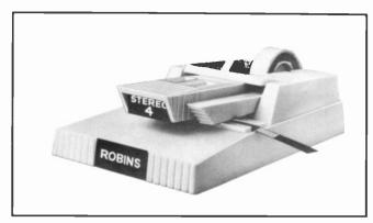
Used for magnetic recording tape, this unit cuts two rounded indentations in the tape splice, giving the splice a "Gibson Girl" shape and leaving the edges of the tape free of adhesive. The unit can be removed from its base and mounted directly on any tape recorder. It comes complete with a roll of splicing tape and tape feed. Part No. 124 0032 178
