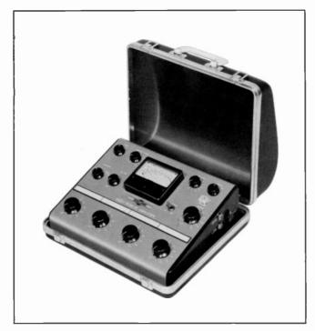
Weighing a total of 22 pounds including batteries and carrying case, the 212Z-1 offers full functions for remote broadcasts. This transistorized remote amplifier mixes inputs from up to four microphones, with program line and communication line outputs as well as an auxiliary output for PA feed.
