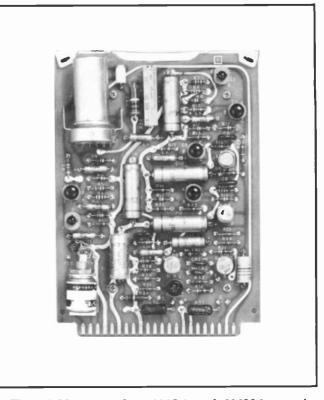
The 356M-1 is used in 212S-1 and 212M-1 consoles as the monitor amplifier.
