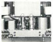
and audio tubes. The bias supply provides approximately 100 volts for the modulator and poweramplifier bias and lesser voltages for other biasing throughout the transmitter.
