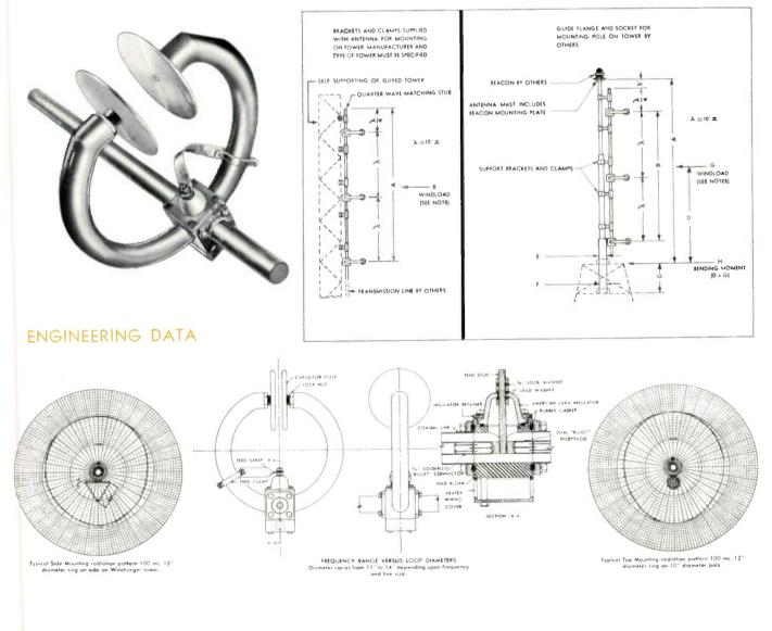
(2) The top or pole mounting design is available on special order for installation on towers where no TV antenna is present or planned. This style of mounting provides the maximum in height and coverage. The light weight and windloading of the top mounting array allow erection on most guyed and selfsupporting towers without extensive tower modification.
