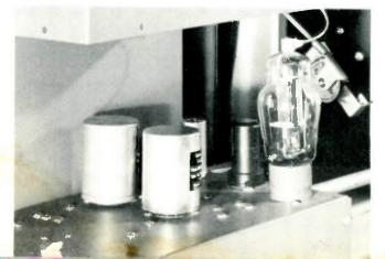
Only seven different tube types are used, resulting in fewer spares to meet FCC requirements.
