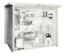
Antenna tuner for towers 2 and 4 in four-tower array of 5 kw station.
