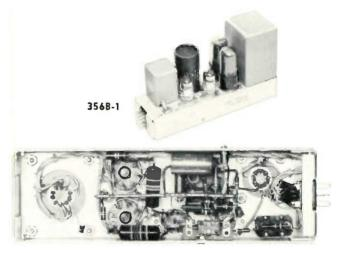
nal. Output Impedance: 150 or 600 ohms balanced or unbalanced. Output Level: +18 dbm maximum Gain: 40 db. Frequency Response:  $\pm 1$  db, 50 to 15,000 cps. Distortion: 0.5% maximum. Noise: -118 at input, or 96 db below full output. Tubes: 2 — 5879. Power Requirements: 6.3 v ac or dc at 0.3 amps. 250 v dc at 6.5 ma or 300 v dc at 7.5 ma. Size: 45%"H, 21%"W, 91/2"D. Weight: 21/4 lbs.
