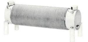
These solenoid wound 2 and 3 wire chokes provide high impedance throughout the broadcast band for isolation of the ac power lines from the antenna. Coils are wound of #10 wire and are rated at 2,000 w, 120 v ac, single phase, assemblies and provided with mounting brackets and standoff insulators for mounting in 42E-7/8 antenna coupling units. Weatherproof cabinets are available for outdoor mounting.
