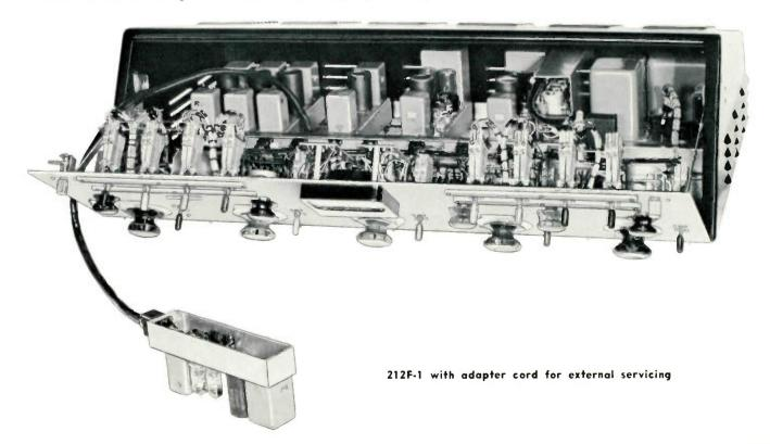
Three of the mixer attenuators have cueing positions. The output of the cue circuit will operate headphones, or a 356A-1 Pre-amplifier may be plugged in to provide 100 milliwatts to a speaker.
