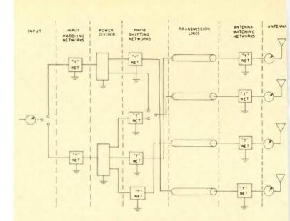
Typical block diagram of Collins directional antenna installation.
