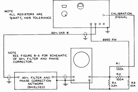
Figure 8-6. Generator Connections for Interference Pattern
