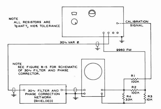
Figure 6-3. Test Set-Up for Phase Relationship, 9960 FM and Calibration Signal
