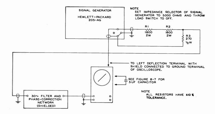
Figure 8-8. Circuit For 30 CPS Channel Calibration
