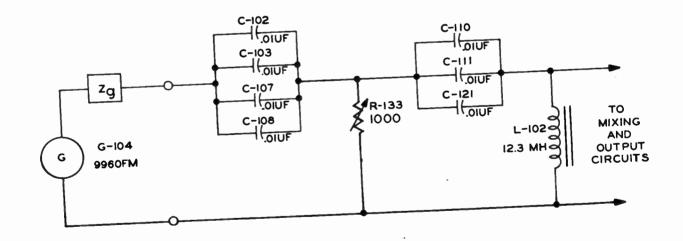
Figure 3-1. Simplified 9960 FM Generating Circuit
