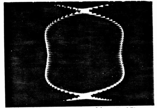
Figure 6-5. Interference Pattern for 180° Line-Up of FM Pickups -- Dial Setting "0"
