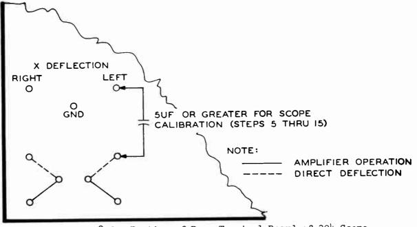
Figure 8-7. Portion of Rear Terminal Board of 304 Scope (Dumont) Showing Amplifier and Direct Connections
