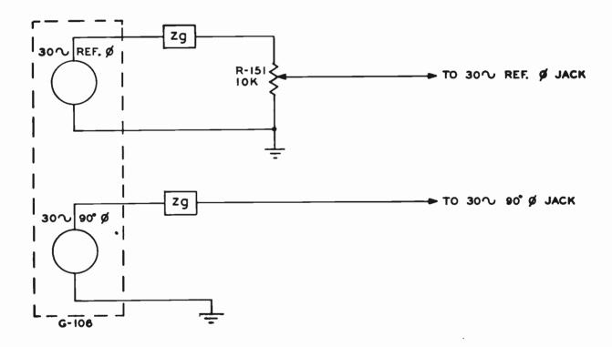
Figure 3-6. Simplified Generating Circuit (30-Cycle Reference Phase and 30-Cycle 90° Phase)
