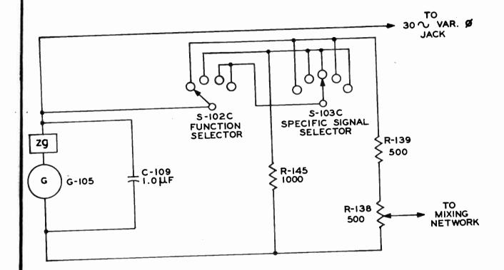
Figure 3-2. Simplified 30-Cycle, Variable Phase Generating Circuit
