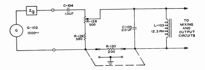
Figure 3-3. Simplified 1020-Cycle Generating Circuit
