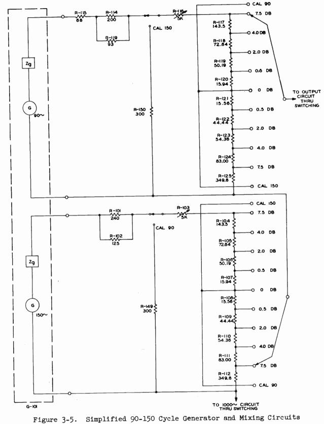
3-20. In the 150 cps circuit with the generator having a resistance of 223 ohms at 25°C.  $(+77^{\circ}F)$  the 125 ohm (at 25°C) resistor (R-102) is paralleled by a stable 240 ohm resistor (R-101). The sum resistance is approximately 300 ohms.
