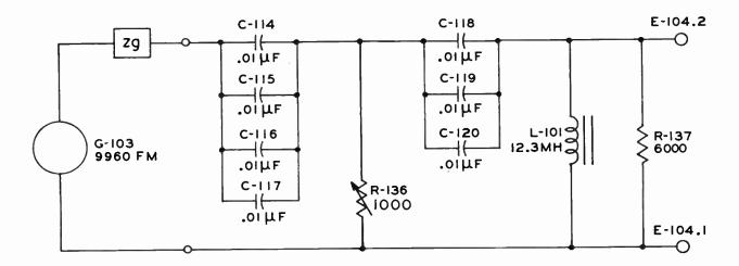
Figure 3-4. Simplified 9960-Cycle FM Generating Circuit (Calibration)
