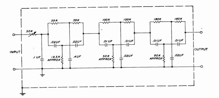
Figure 8-5. 30 cps Filter and Phase-Correction Network
