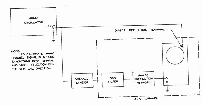
Figure 8-3. Arrangement for Calibration of  $30 \sim Channel$
